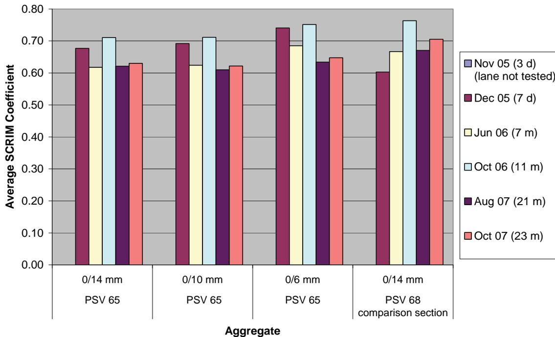
**Figure 6.2 Variation in low-speed skid resistance (SCRIM Coefficient at 50 km/h) over time: Site 1b (A5 Gibbet Hill, Lane 2), Dec. 2005 to Oct. 2007**
