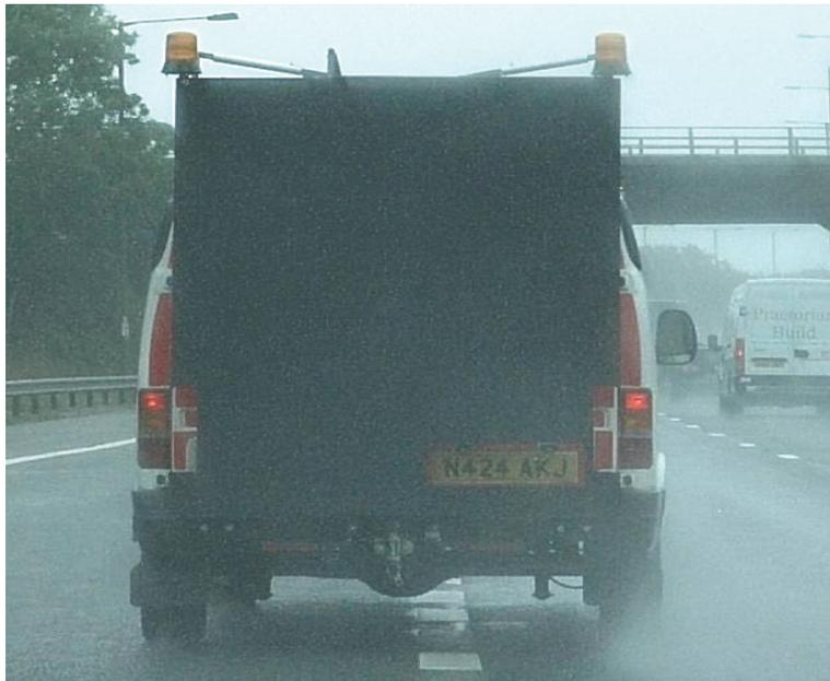
**Figure 7.2 Target board mounted on mini-bus (during a trial run)**
