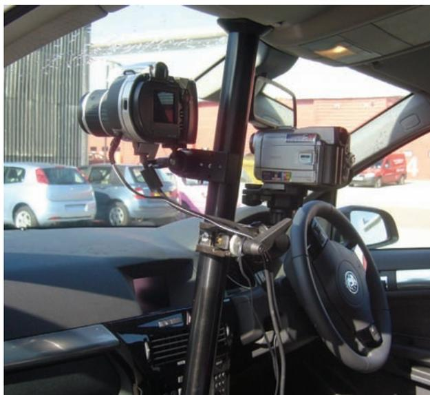
**Figure 7.3** Cameras mounted on an “Autopole” in front of the passenger seat looking through the windscreen
