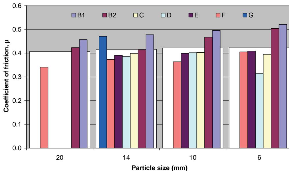
**Figure 6.9**  $\mu_{PWS60}$  against particle size for resin mosaic specimens from different aggregate sources
