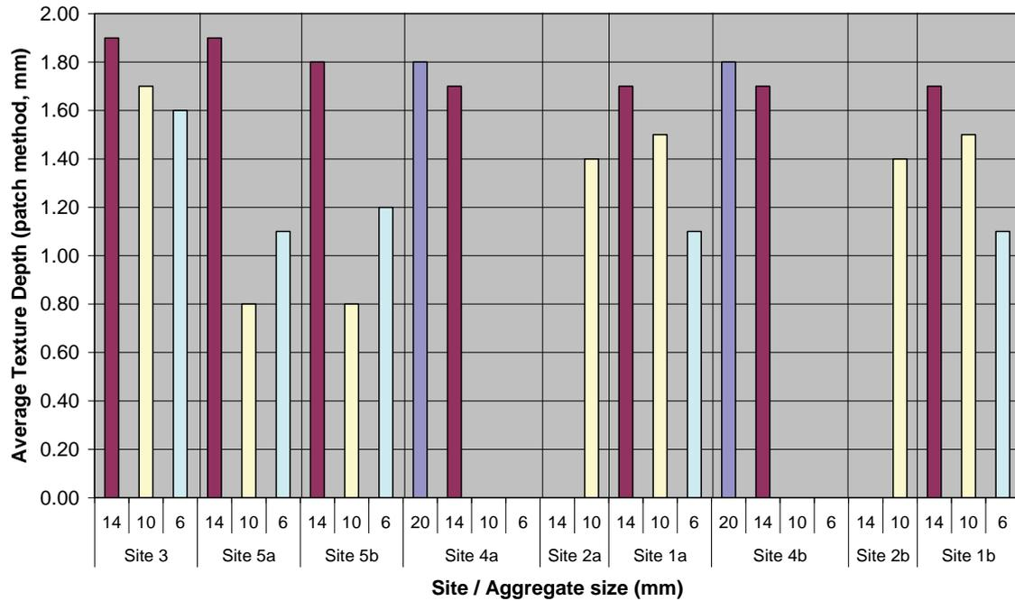
**Figure 6.4 Average texture depth (patch method) on the trial sections when new**
