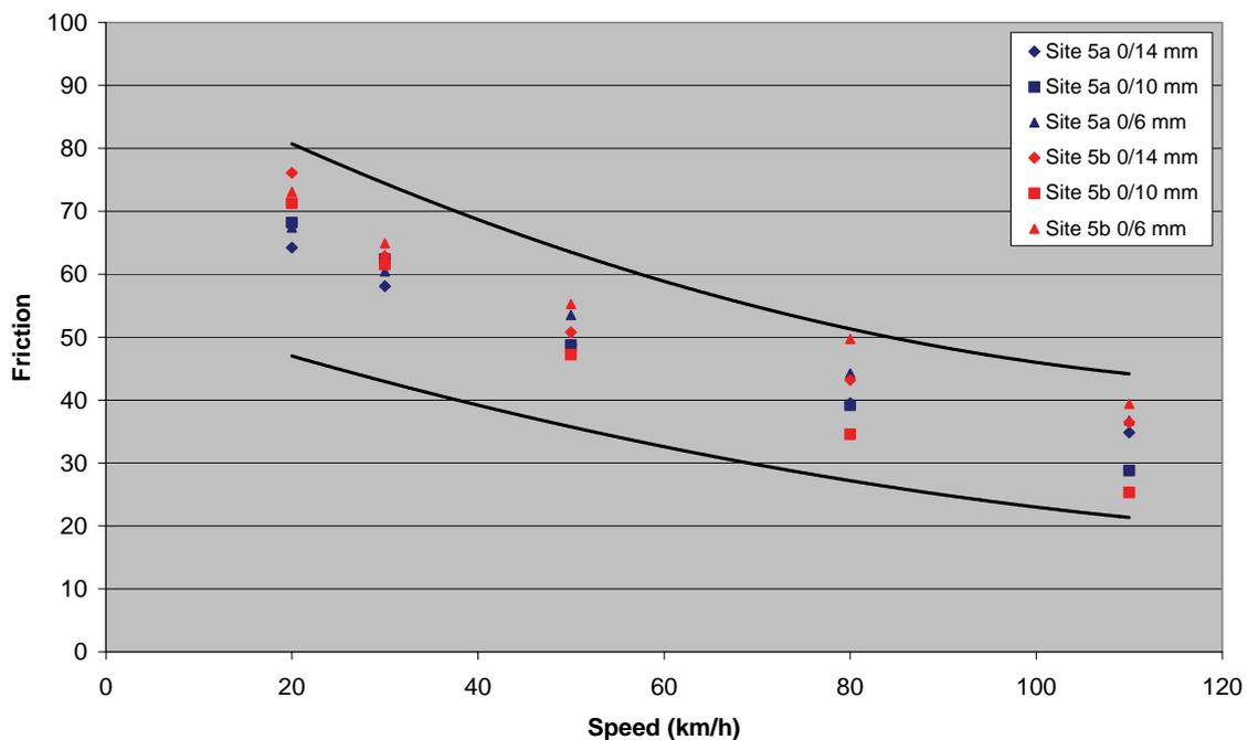
**Figure 6.7 PFT locked-wheel wet friction versus speed for Site 5, November 2007**
