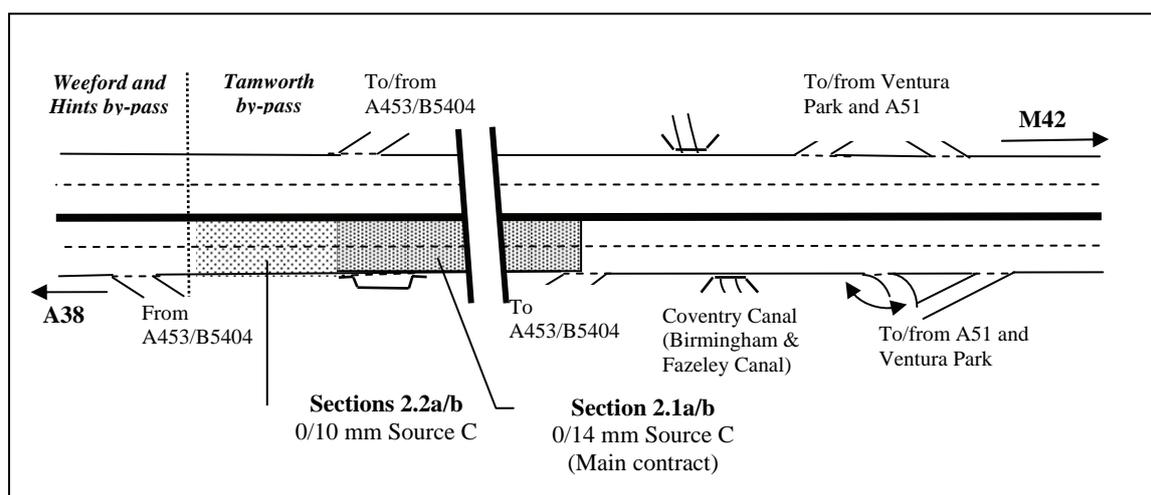
**Figure 9.3 Schematic diagram of Location 2, A5 Tamworth by-pass**
