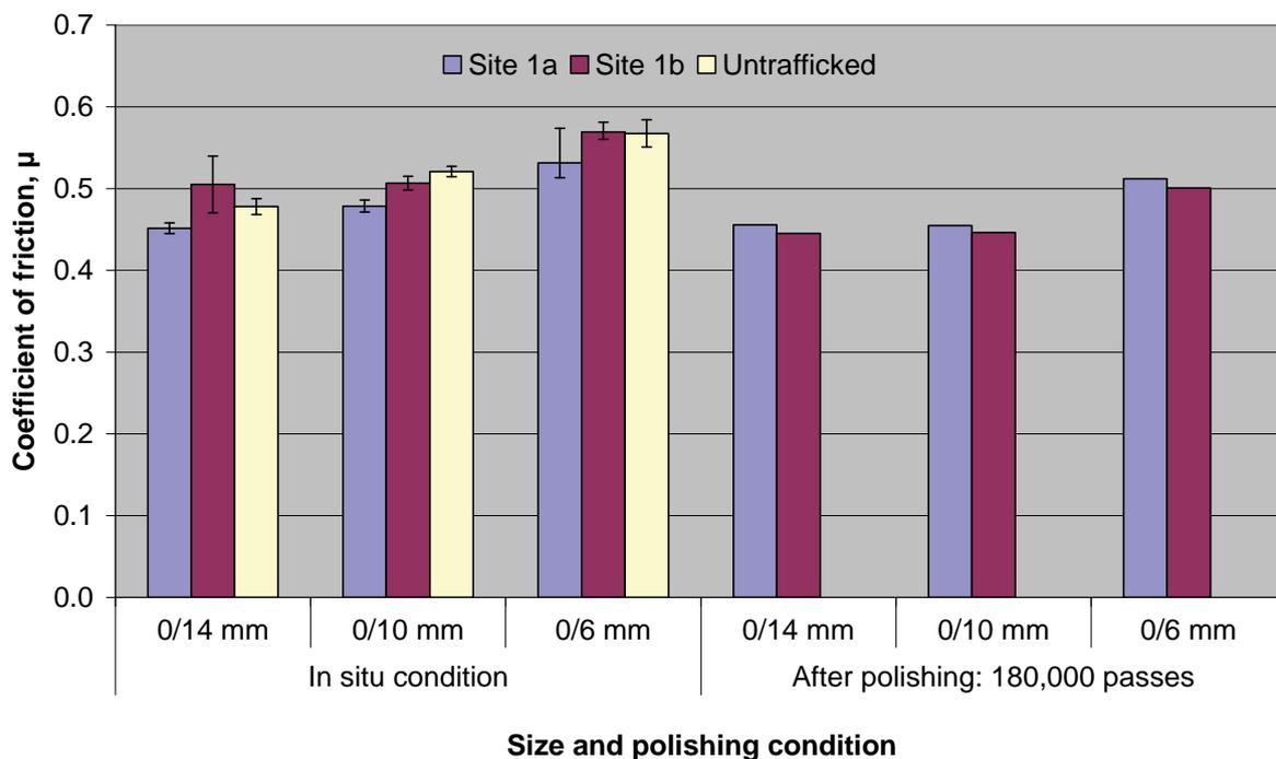
**Figure 6.12 Friction measurements on cores taken from Trial Sites 1a and 1b**
