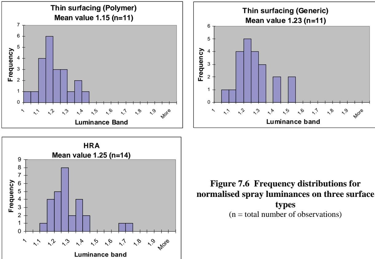
**Figure 7.6 Frequency distributions for normalised spray luminances on three surface types**
