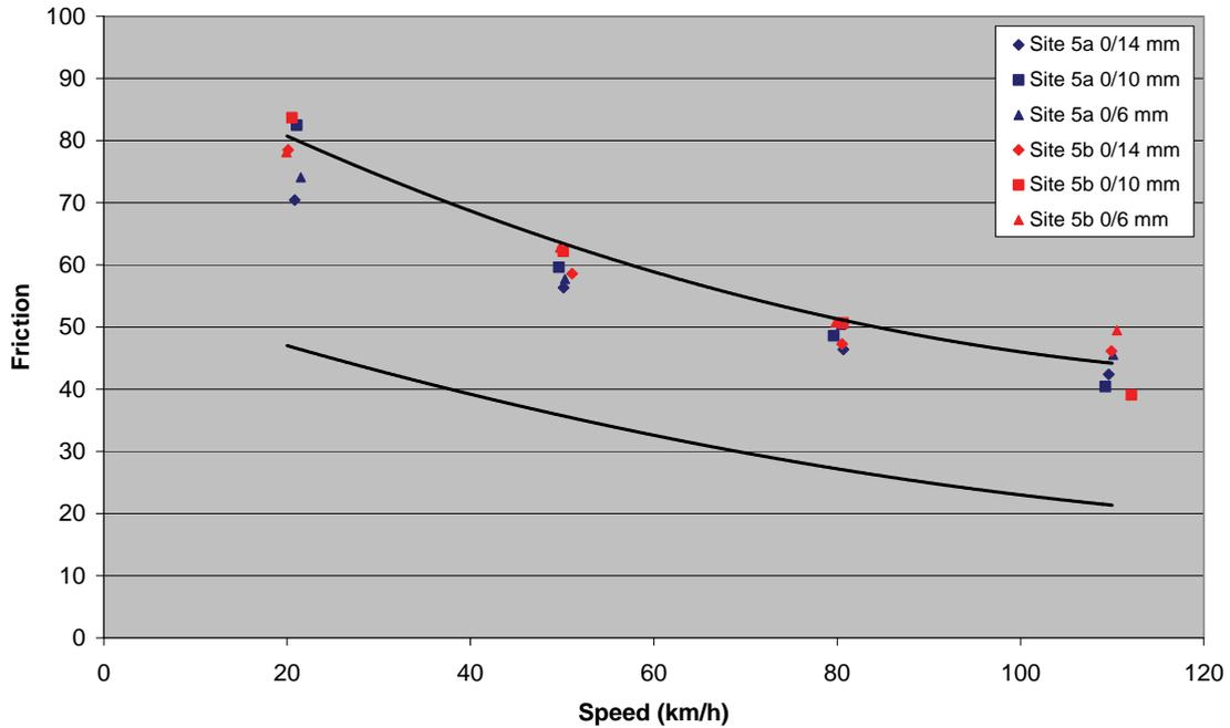
**Figure 6.6 PFT locked-wheel wet friction versus speed for Site 5, November 2006**
