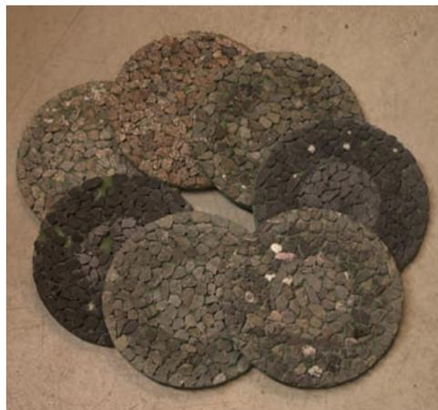
**Figure 5.2** Completed aggregate mosaic specimens using 14 mm aggregate particles
