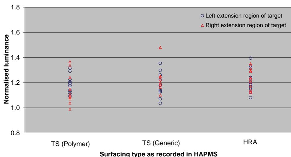
**Figure 7.5 Luminance ratios of left and right extension target regions versus surface type**
