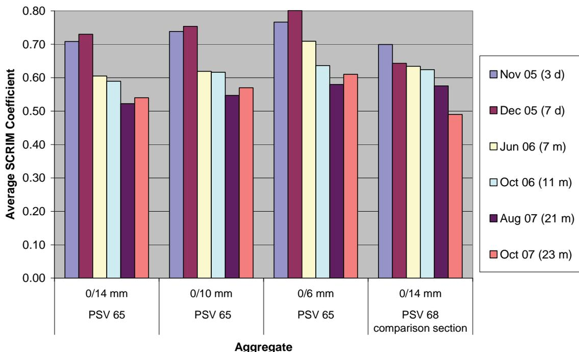
**Figure 6.1 Variation in low-speed skid resistance (SCRIM Coefficient at 50 km/h) over time: Site 1a (A5 Gibbet Hill, Lane 1), Nov. 2005 to Oct. 2007**
