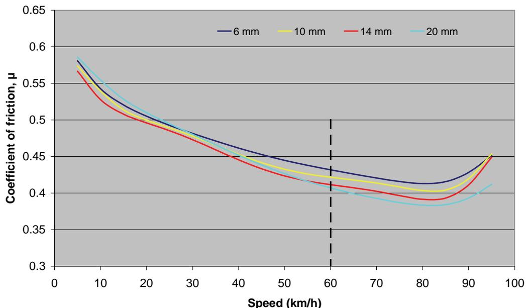
**Figure 6.11** Coefficient of friction against test speed
