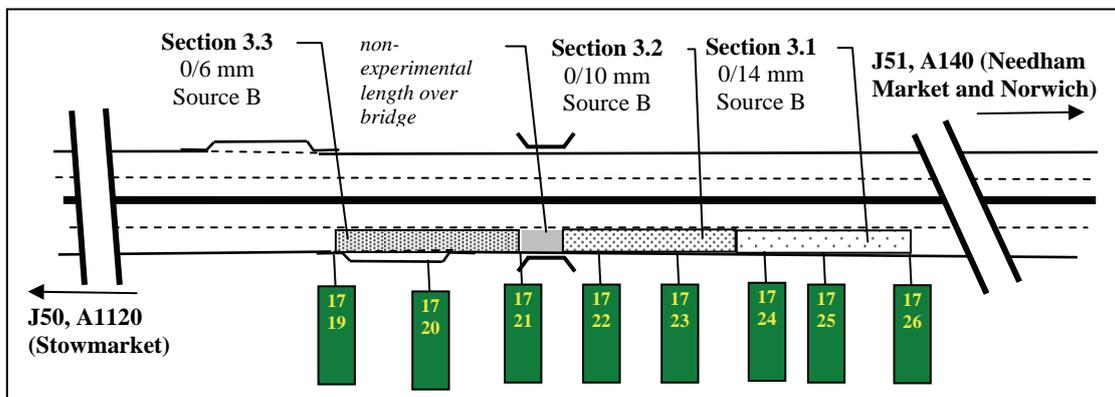
**Figure 9.4 Schematic diagram of Site 3, A14 Creting St Mary**
