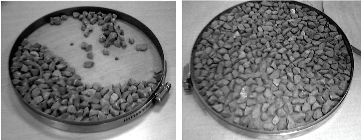
**Figure 5.1** *Left:* aggregate particles being arranged in a mould
