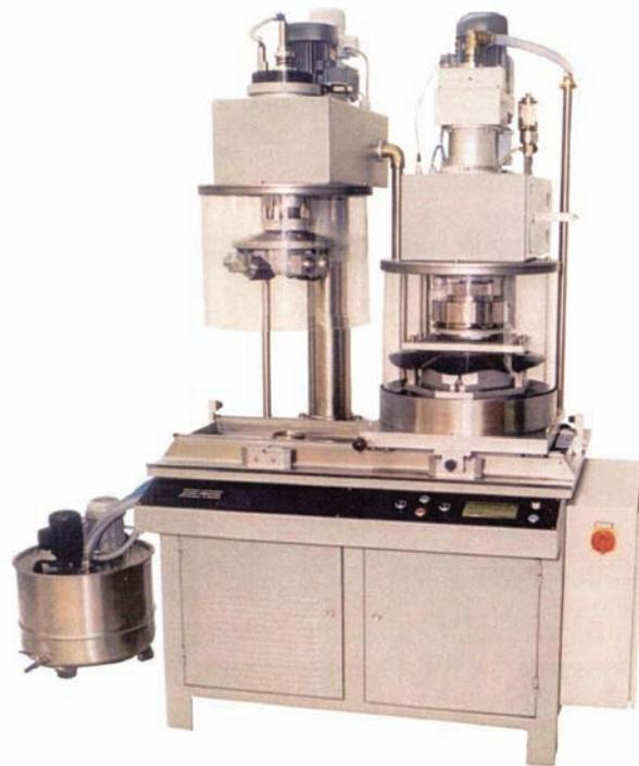
**Figure 9.1 The Wehner/Schulze test equipment**
