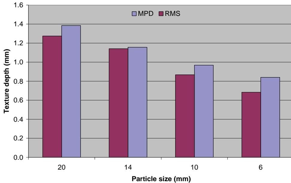
**Figure 6.10** Texture depth on resin mosaic specimens
