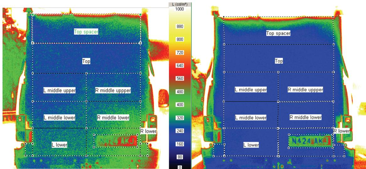
**Figure 7.4 Comparison of false-colour luminance images with spray (left) and without spray (right)**
