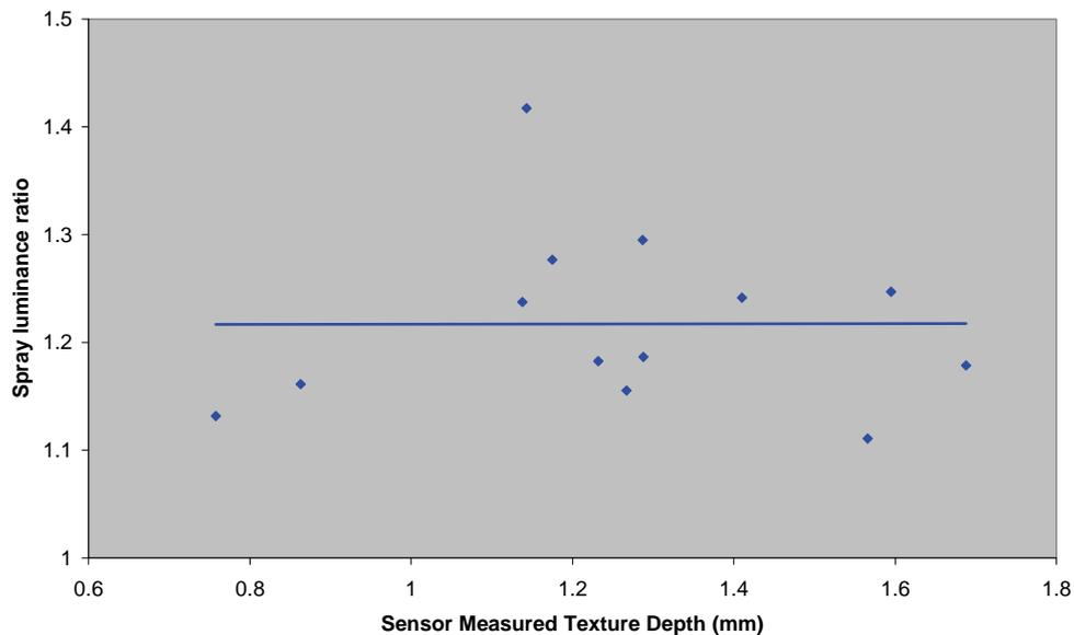
**Figure 7.8 Average spray luminance ratio in “lower extension” zones for a range of texture depths**
