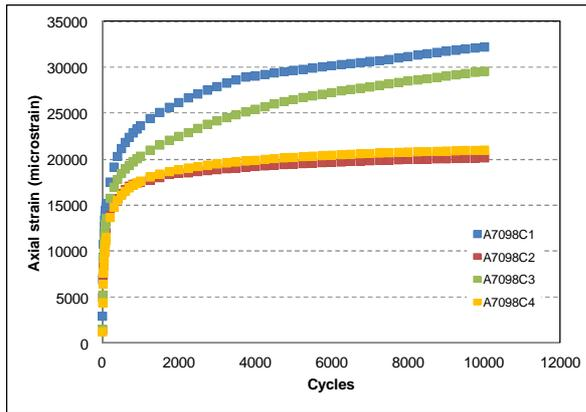
**Figure 5-4: Creep curves for Mixture 1 (LTA binder course)**
