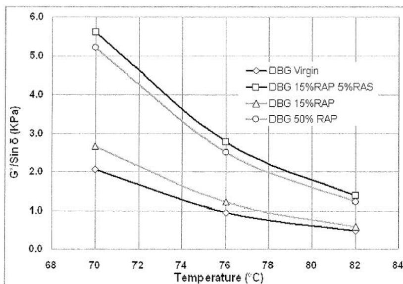
Figure G-1: Recovered bitumen  $G^*/\sin(\delta)$  at different temperatures
