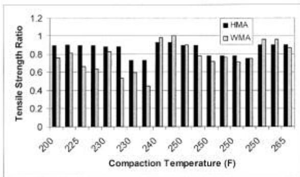
**Figure G-4: TSR results for HMA and WMA**
