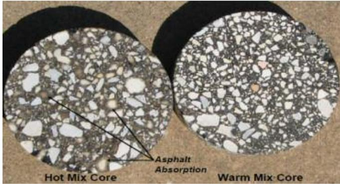
**Figure G-13: Photos of Loop 368 one-year cores**
