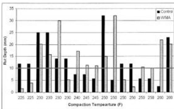
**Figure G-6: Hamburg rut depths for HMA and WMA**
