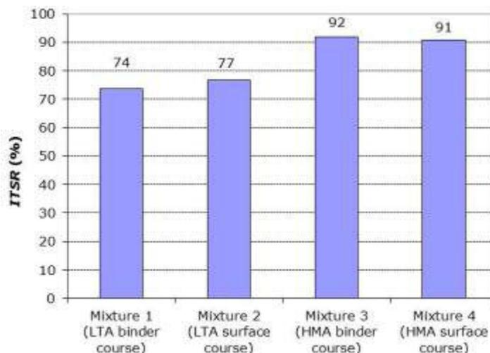
**Figure 5-3: Water sensitivity test results at 20 °C**
