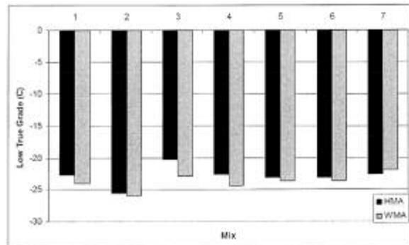
**Figure G-9: Low continuous grades for HMA and WMA**
