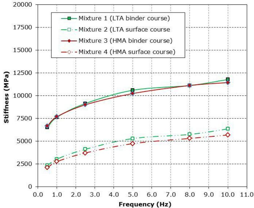
**Figure 5-12: 4PB stiffness test results at 15 °C**
