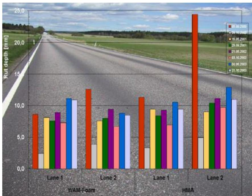
Figure H-1: Rutting 2000 to 2005 on RV120, Hobøl
