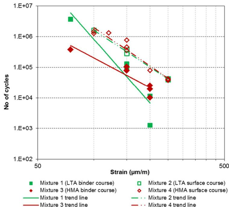
**Figure 5-14: Laboratory fatigue results**
