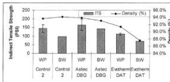
**Figure G-12: Indirect tensile strength of cores for Danley and Murfreesboro plant mixtures**
