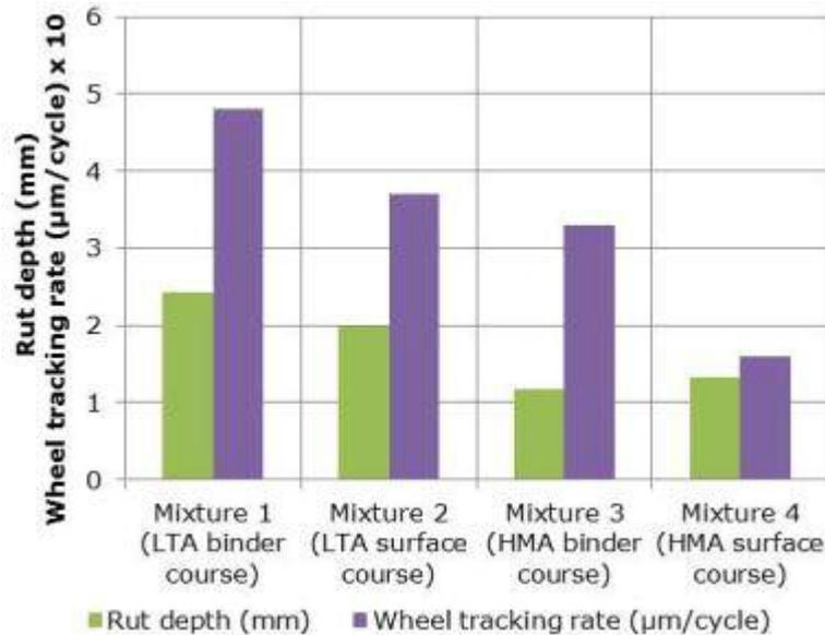
**Figure 5-7: Wheel-tracking results for small size device to Procedure A**
