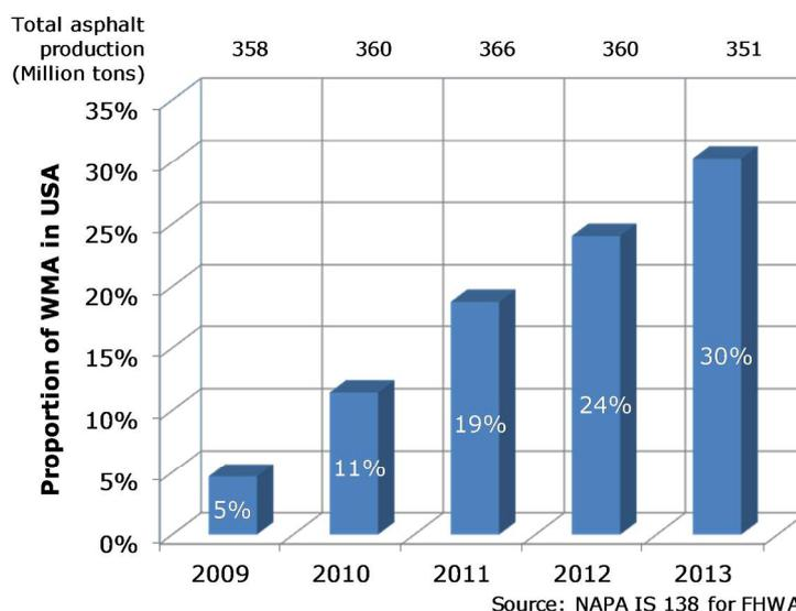
**Figure 7-2: Development in the production of warm mix asphalt in USA**
