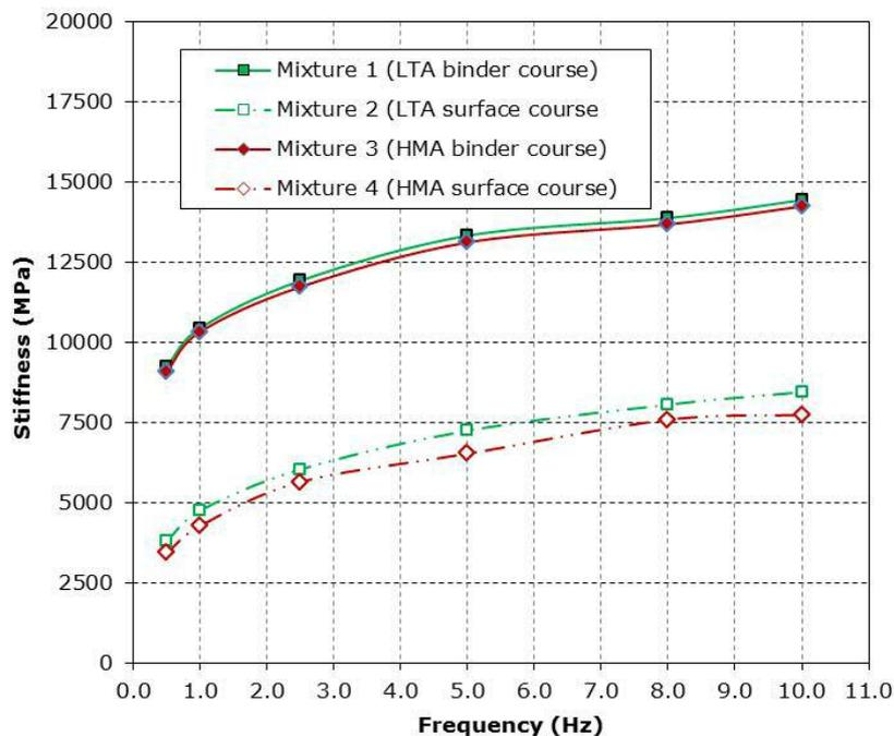
**Figure 5-13: 4PB stiffness test results at 10 °C**
