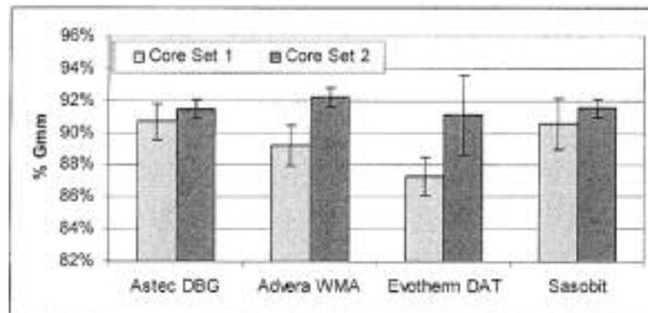
**Figure G-10: Field densities after construction**
