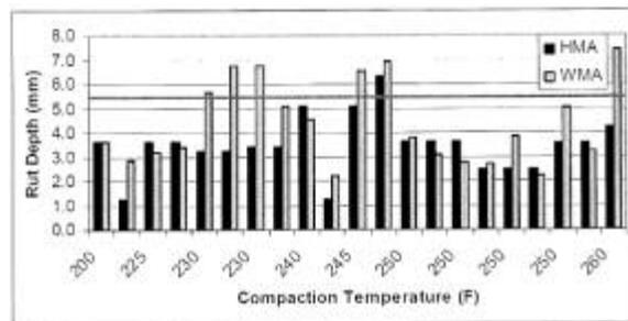
**Figure G-7: APA rut depths for HMA and WMA**
