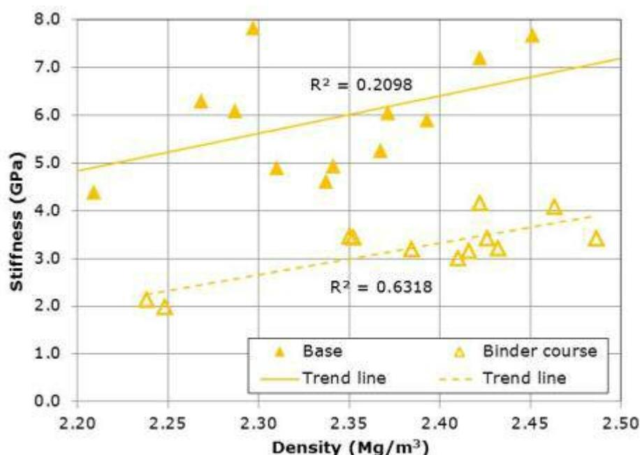
**Figure 7-1: Relationship between stiffness and density of cores**
