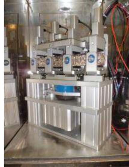
**Figure 5-10: Four-point bending test set-up**
