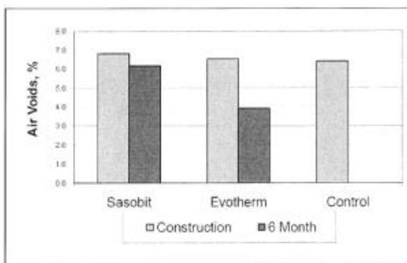
**Figure G-2: In-place air voids contents, Milwaukee trial**
