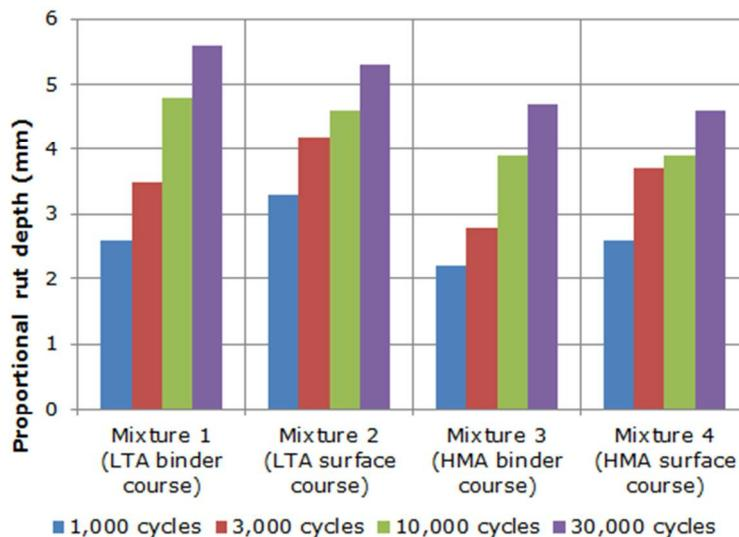
**Figure 5-6: Wheel-tracking results for large size device**
