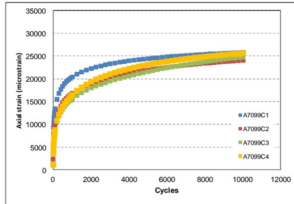
**Figure 5-5: Creep curves for Mixture 3 (HMA binder course)**
