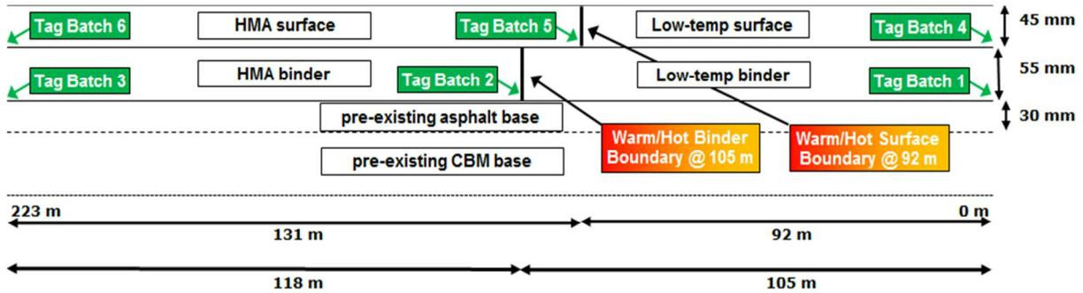
**Figure 2-3: Cross sectional representation of completed works (with site measured distances and RFID tag locations indicated)**
