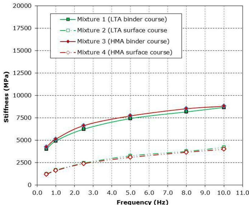
**Figure 5-11: 4PB stiffness test results at 20 °C**
