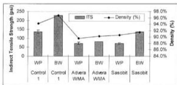
**Figure G-11: Indirect tensile strength of cores for Franklin plant mixtures**
