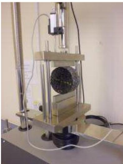
**Figure 5-2: Indirect tensile strength test set-up**
