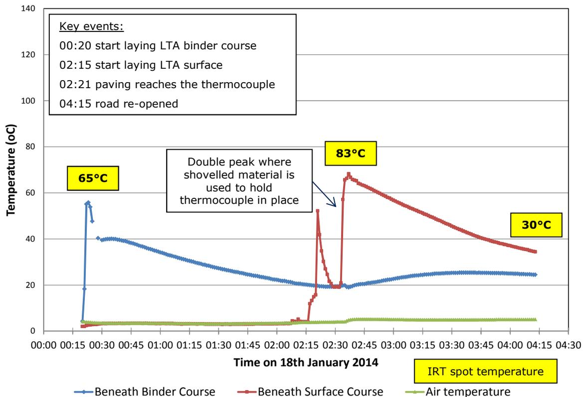
**Figure 4-1: LTA mat temperature profiles (from thermocouples at approximate chainage 2985 m)**
