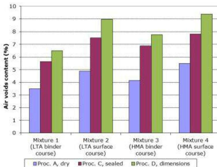
**Figure 5-1: Air voids content of laboratory compacted specimens**
