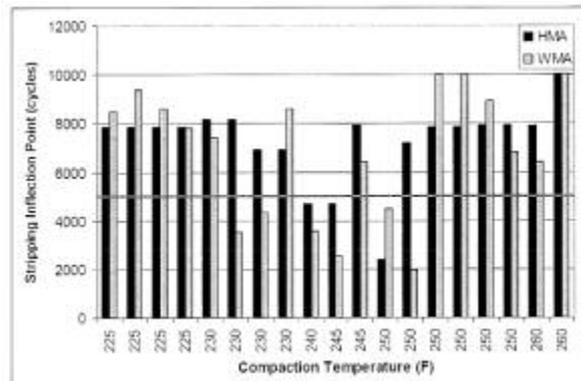
**Figure G-5: Hamburg stripping inflection points for HMA and WMA**
