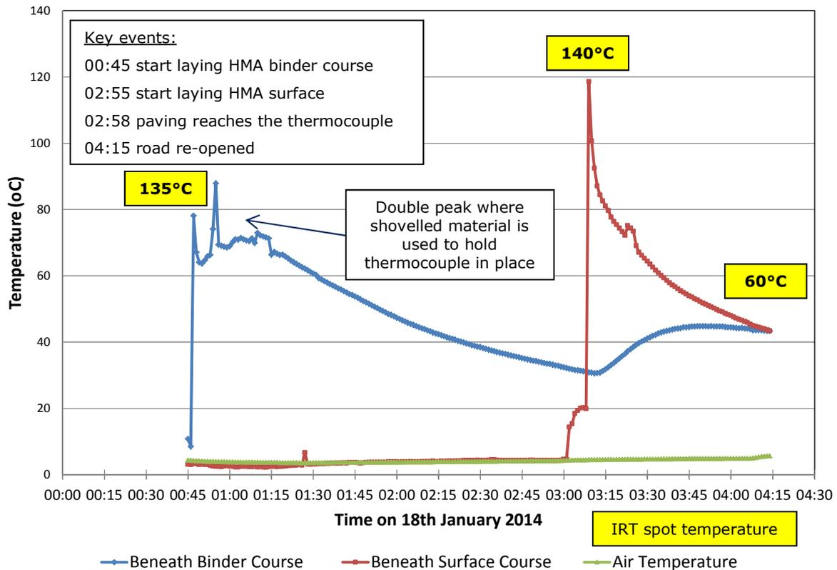
**Figure 4-2: HMA mat temperature profiles (from thermocouples at approximate chainage 3075 m)**
