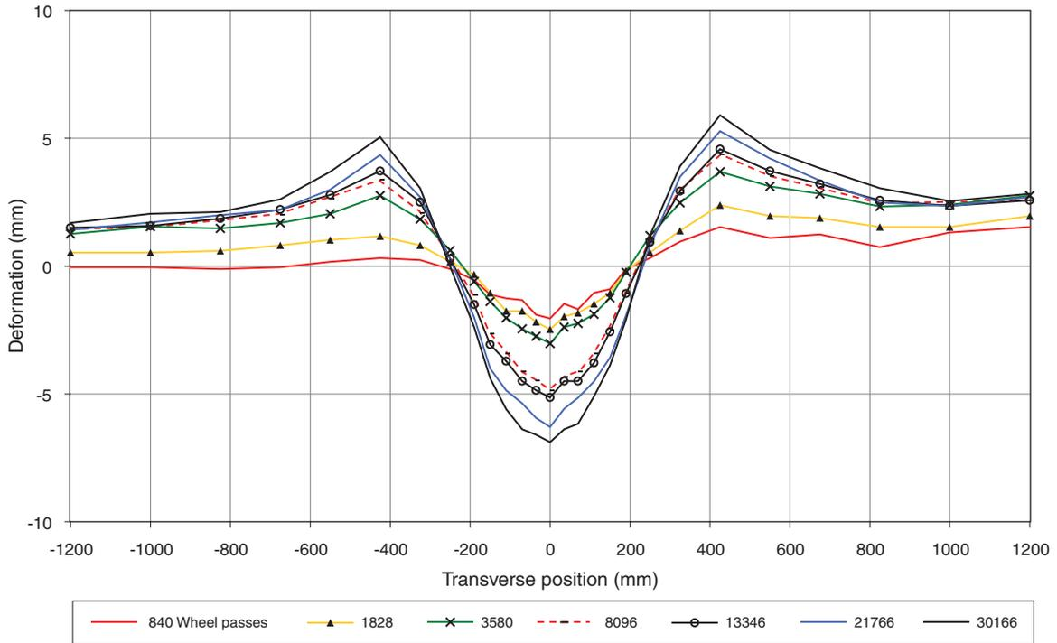
**Figure 8.2** Development of transverse profile in wheel-track 1 (Full width inlay of EME Class 2 binder course)
