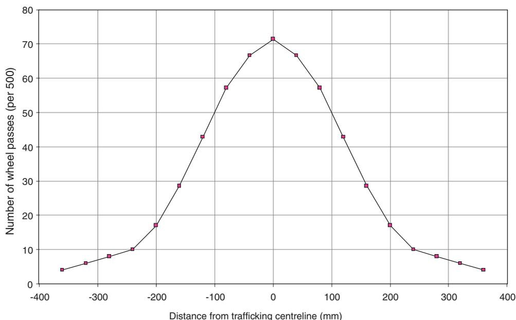
**Figure 6.4** Lateral distribution of wheel loads in the PTF
