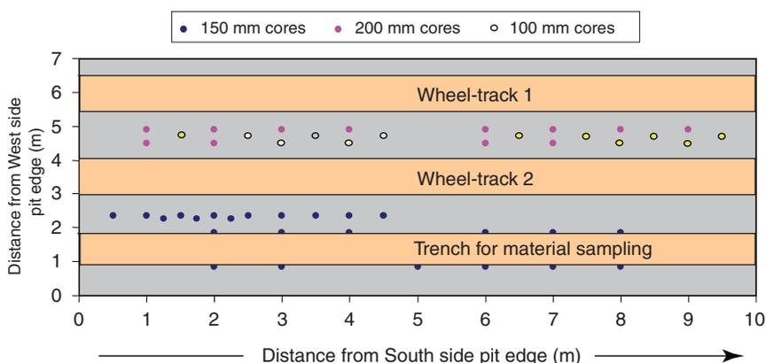
**Figure A.4 Core positions for material sampling**
