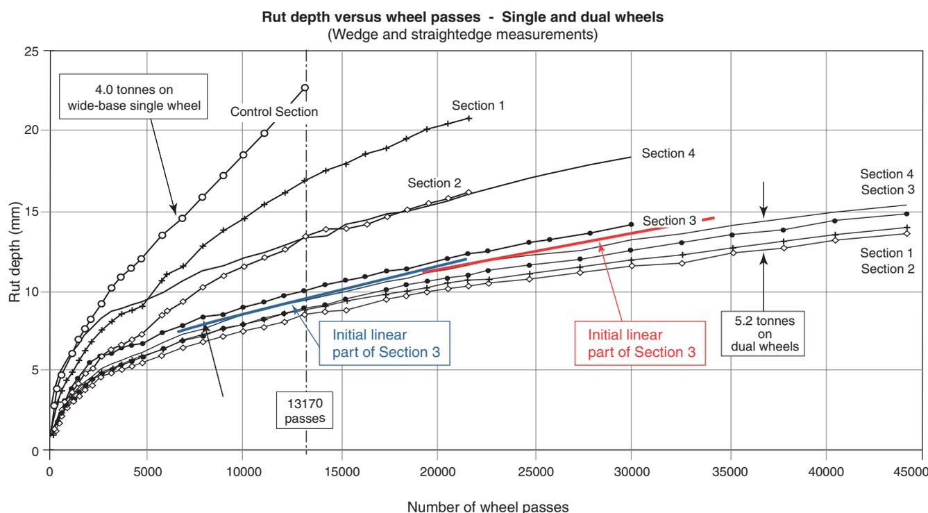
**Figure 9.1** Rut depth versus wheel passes (Weston *et al.*, 2001)
