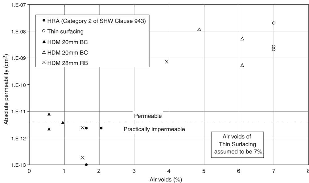
Figure 3.1 Permeability versus air voids
