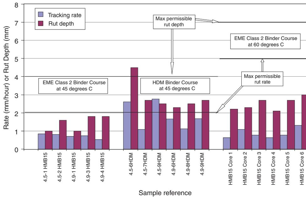
Figure A.8 Wheel-tracking test results of HDM and EME Class 2
