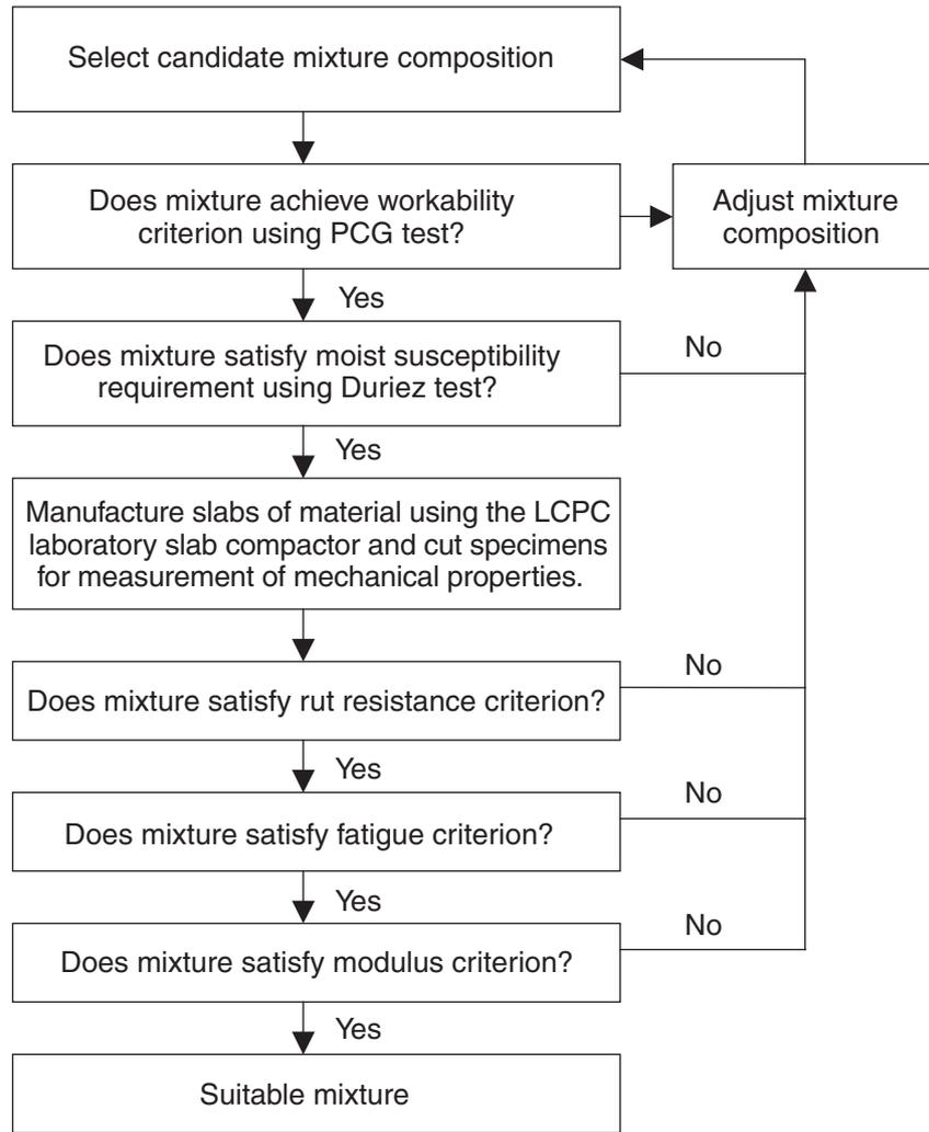
**Figure 4.1** French mixture design procedure
