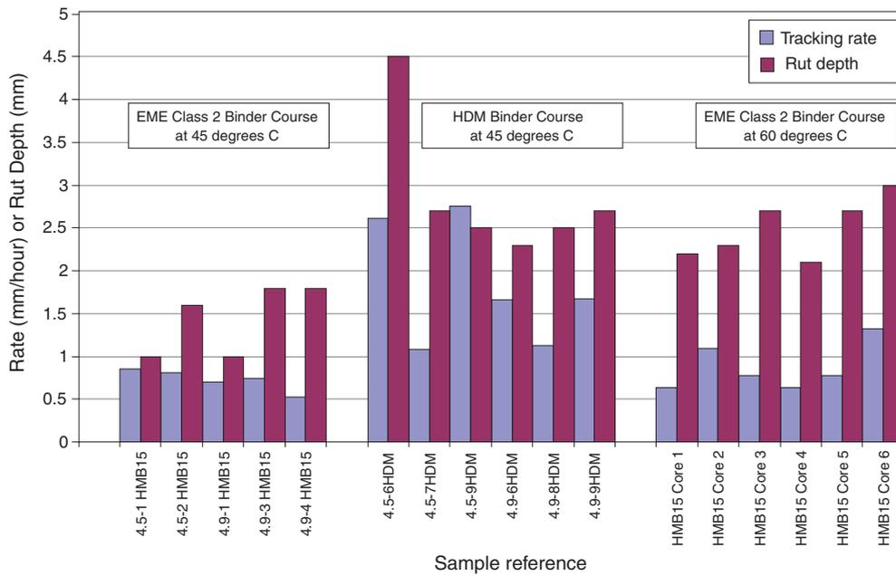
Figure 8.12 Summary of wheel-tracking test results for EME Class 2 and HDM binder courses
