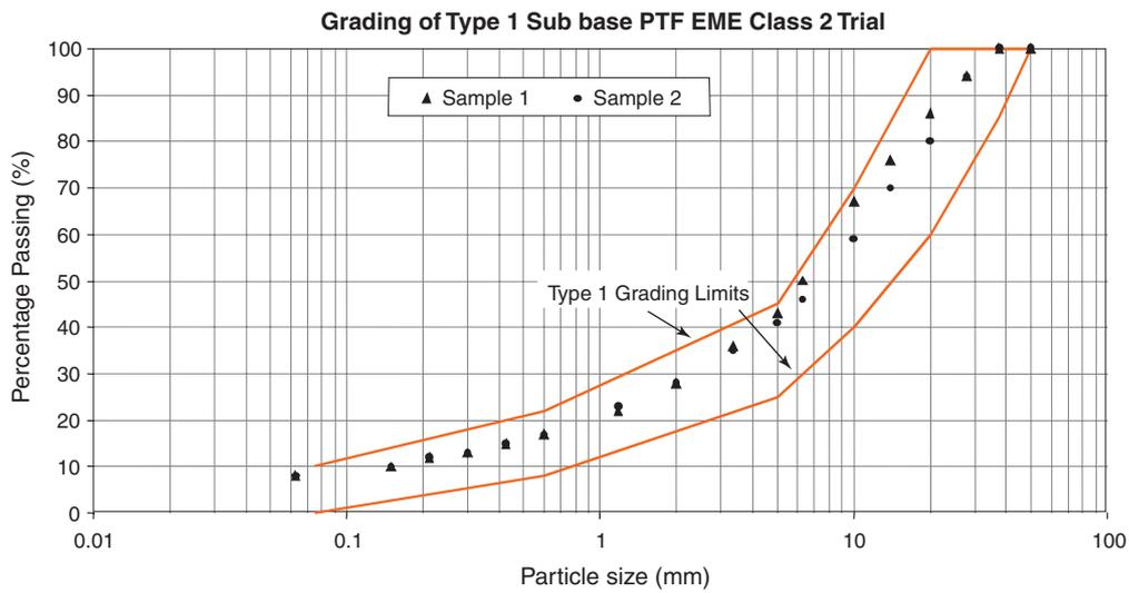
Figure A.2 Grading of subbase
