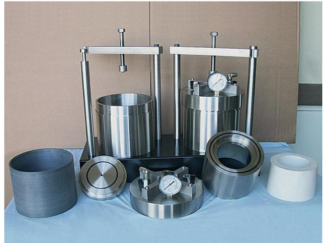
**Figure 7.1** The TRL permeability cell
