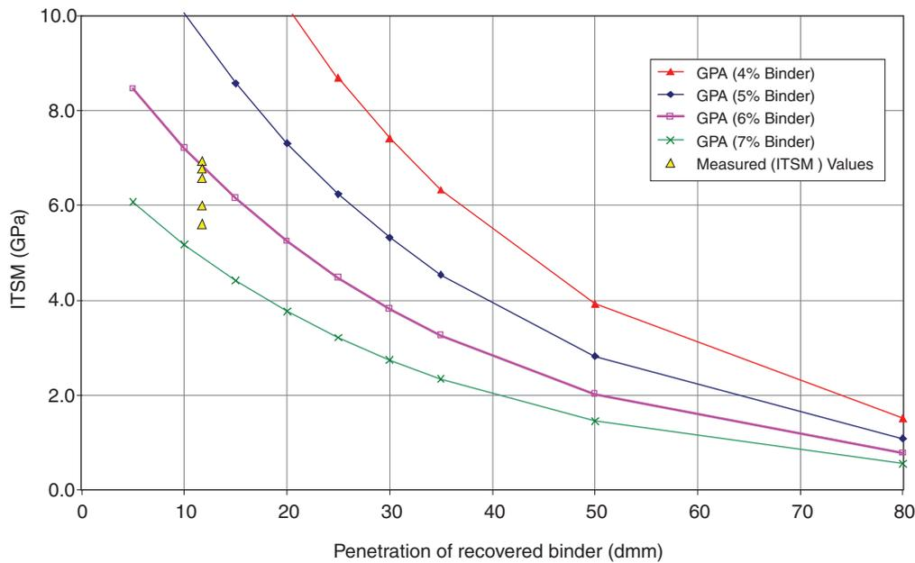
**Figure 10.1** Comparison of theoretical and measured values of stiffness
