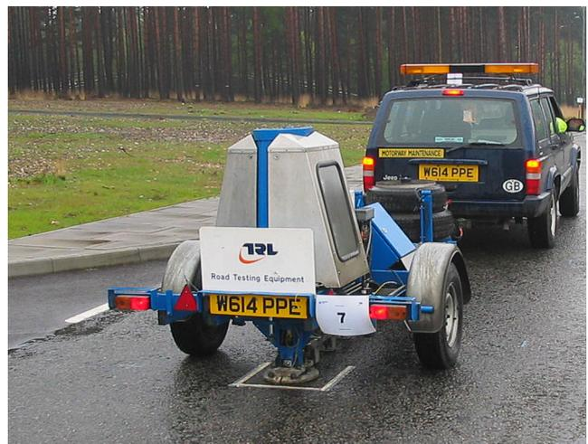
Figure 4.1 The falling weight deflectometer (FWD)
