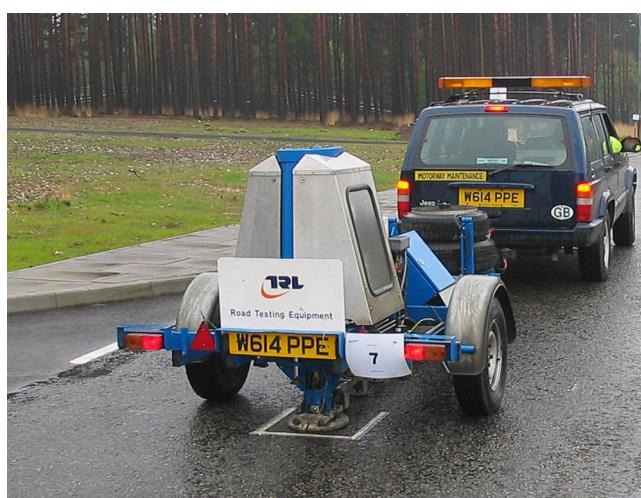
Figure 4.1 The falling weight deflectometer (FWD)
