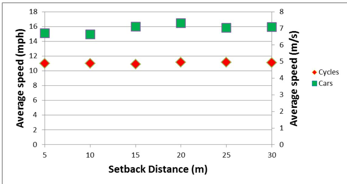
**Figure 7: Average Speed over 60m run for each set-back distance**
