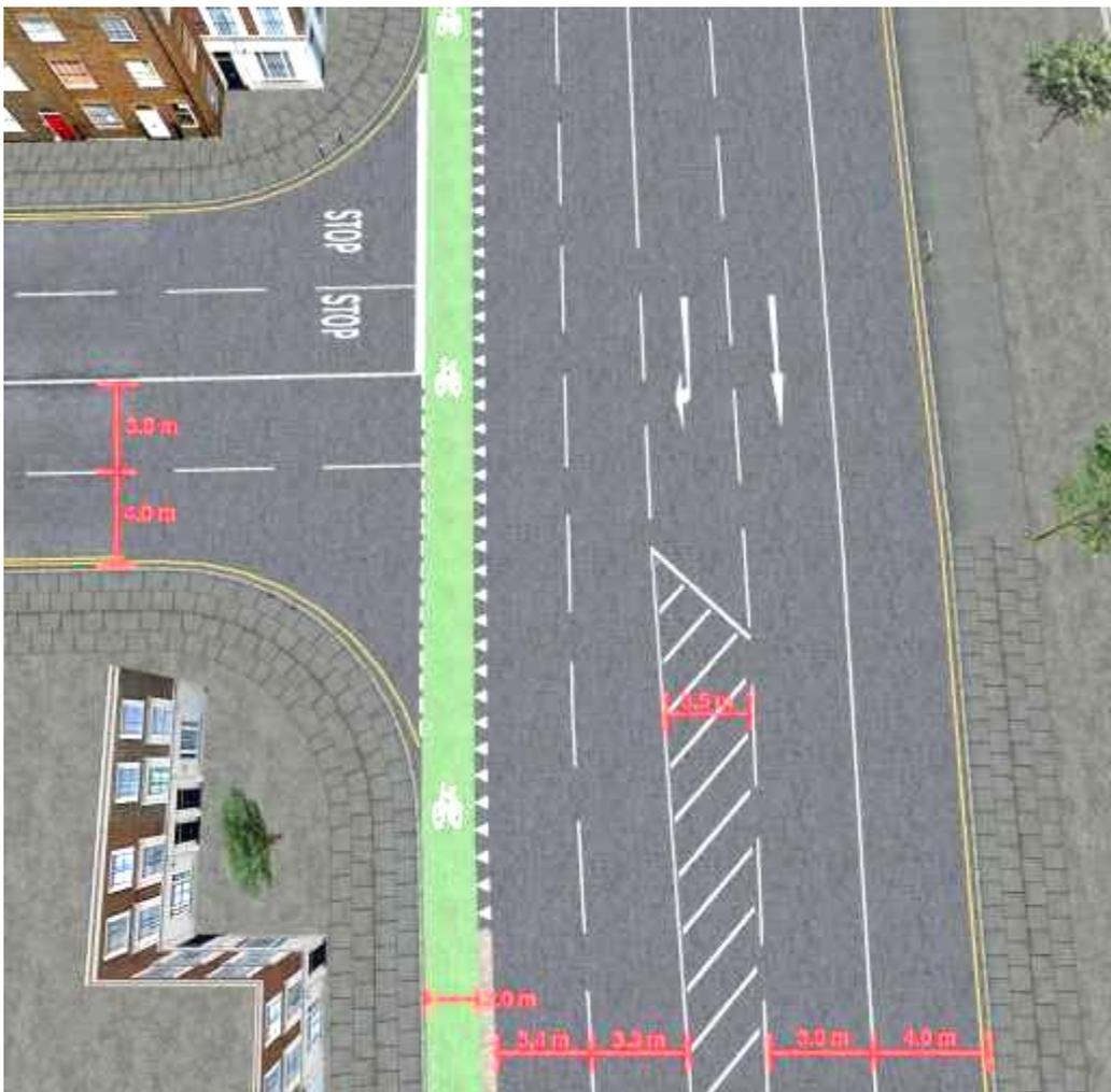
**Figure 4: Screenshot of simulated layout showing lane markings and widths for M13 trial**
