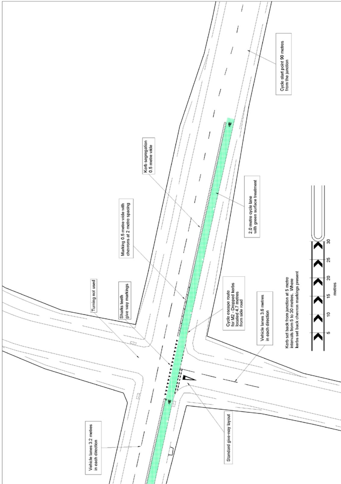
Figure 2: Design layout for track trials (M1, M2, and M4)
