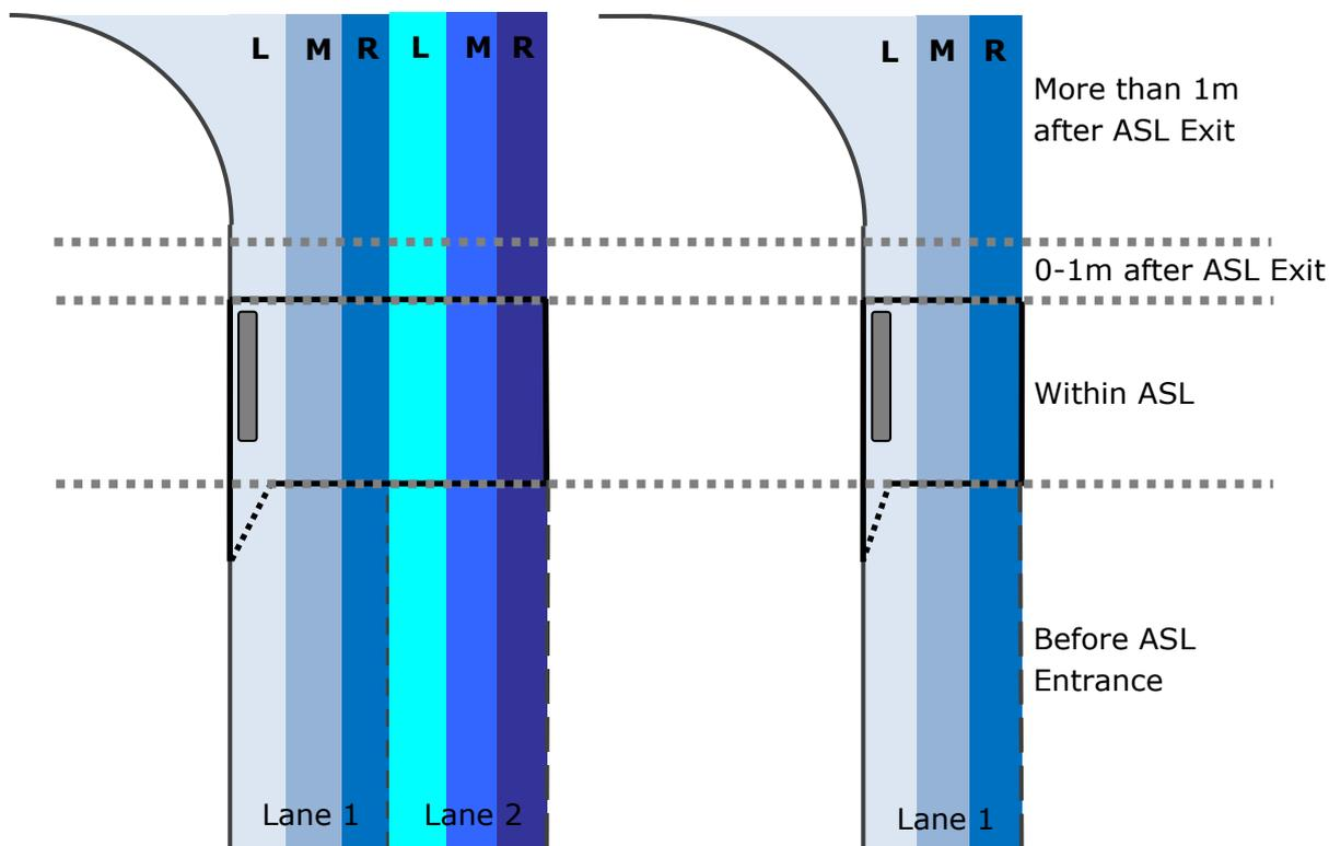
**Figure 9 – Cycle trial: stopping zones**
