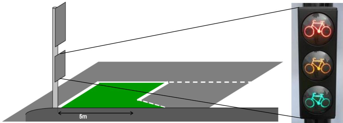
**Figure 4 – Locations of signals and size of ASL**
