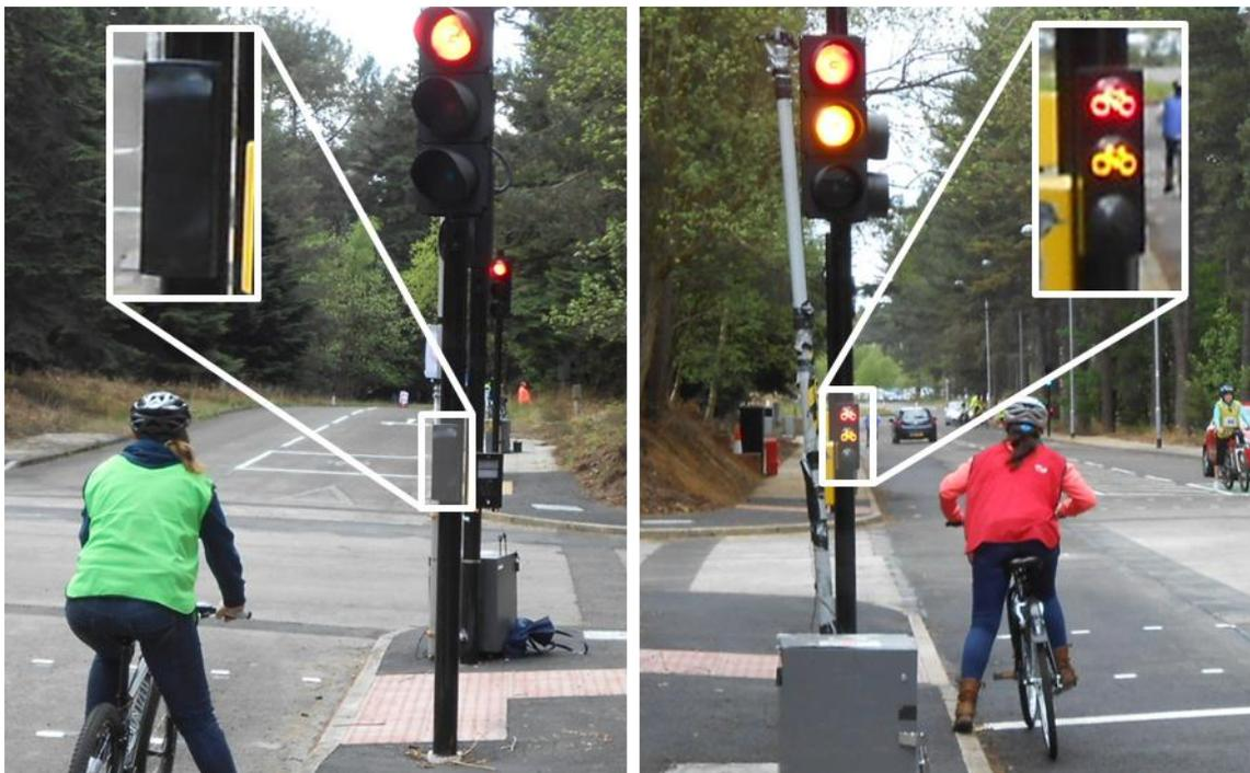
**Figure 3 – “Control”, LLCS covered (left) and “Treatment”, LLCS uncovered (right)**
