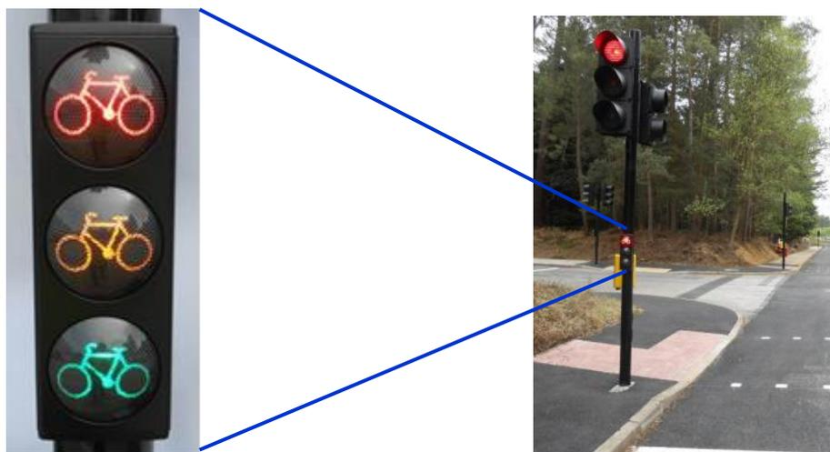
**Figure 1 – Low Level Cycle Signals**
