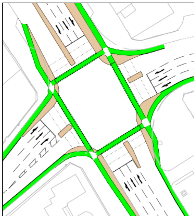
Fully Segregated Signalised Junction - concept
