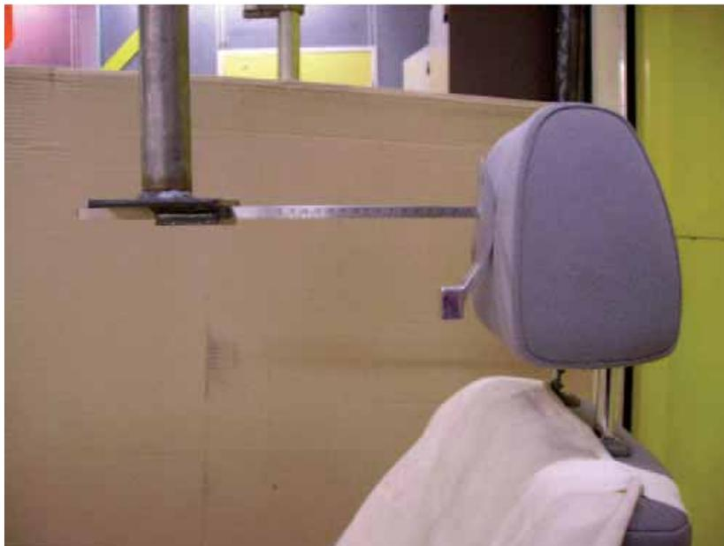
**Figure 5.2** HRMD backset probe held in position using the adjustable portal arm
