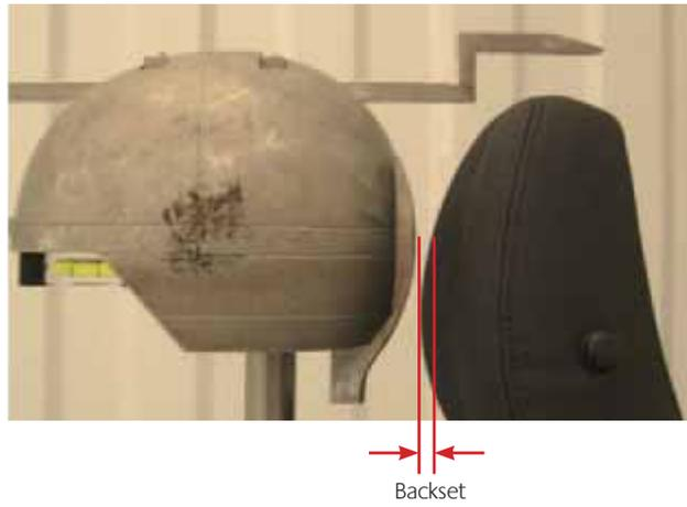
**Figure G1** Head restraint backset, ready for measurement with an HRMD
