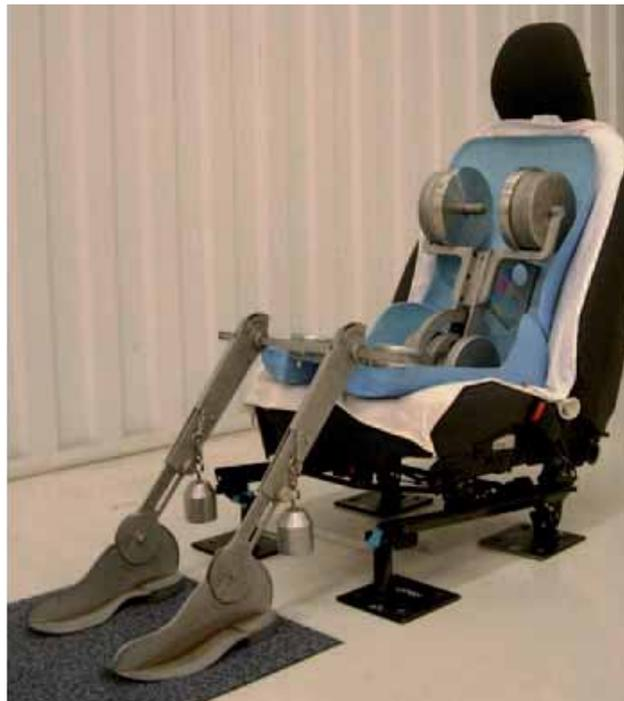
**Figure G3** SAE J826 H-point machine (no HRMD)
