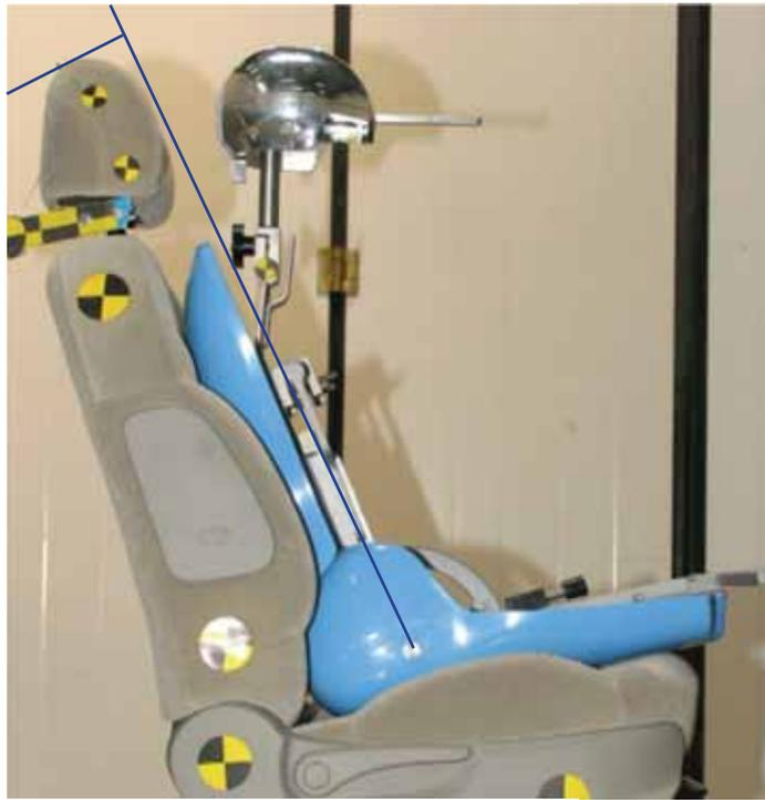
**Figure A1** UNECE Regulation 17 method for measuring head restraint height
