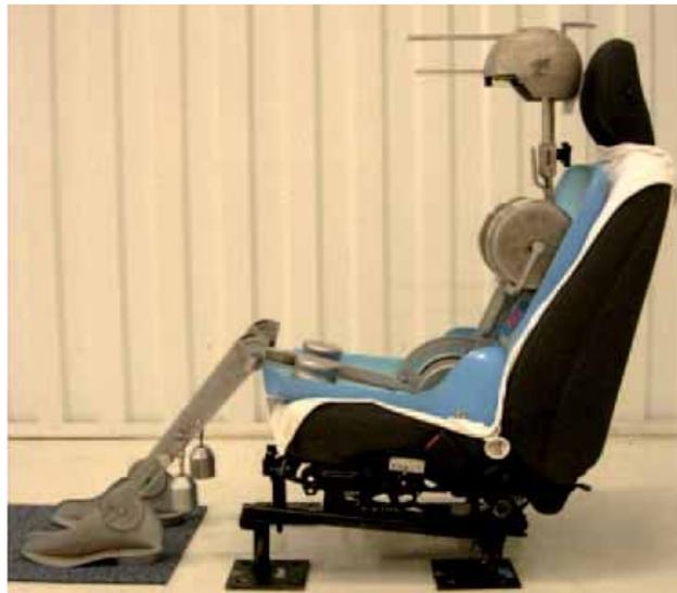
**Figure G2** HRMD fitted onto an SAE J826 H-point machine
