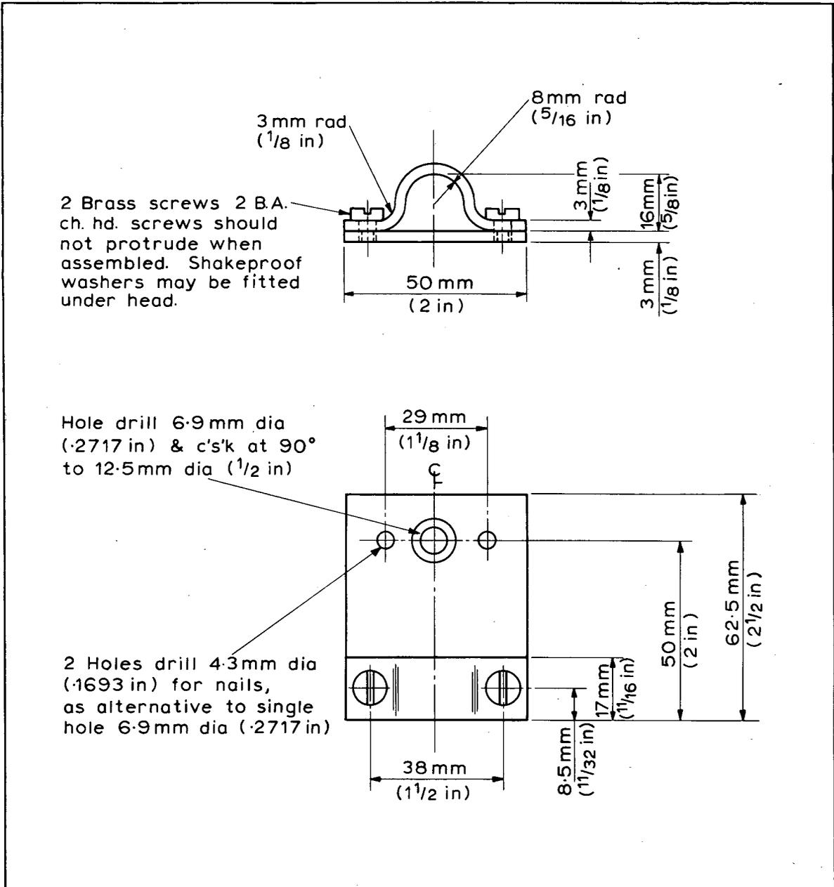
Fig. 3. END FIXING
