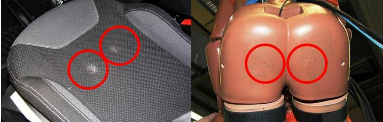
FIG. 3 CONTACT POINTS FROM THE SEAT PAN AND CORRESPONDING DAMAGES AT THE DUMMY BOTTOM IDENTIFIED AFTER A 56 KM/H CRASH TEST AGAINST THE FULL WIDTH DEFORMABLE ELEMENT
