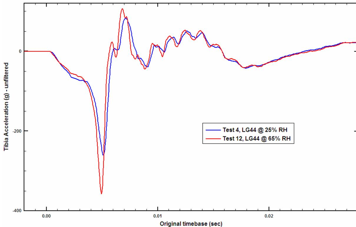
**Figure 4.3. Comparison of tibia accelerations obtained in tests at 25 percent and 65 percent relative humidity, unfiltered**
