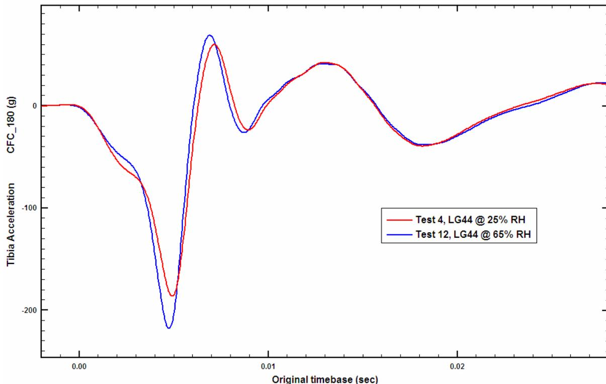
**Figure 4.2. Comparison of tibia accelerations obtained in tests at 25 percent and 65 percent relative humidity, filtered at CFC 180**
