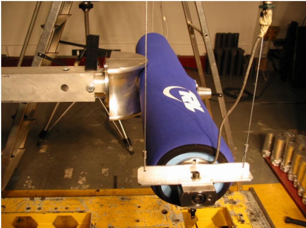
**Figure 2.1. Legform impactor certification rig**
