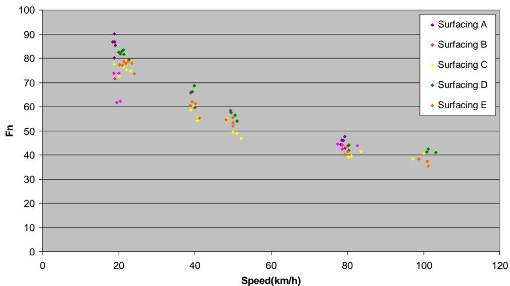
**Figure 8.1 Illustration of the scatter in replicate wet friction measurements using the PFT at different speeds on five different surfacings of similar age**
