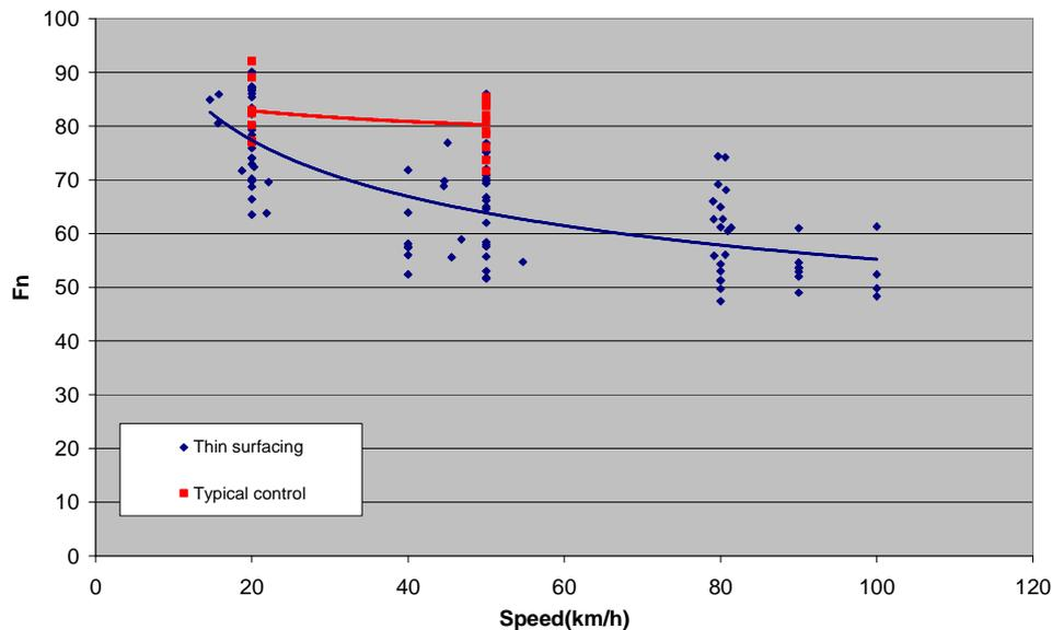
**Figure 8.13 Dry friction measurements at different speeds on all sites from 1 day to 18 months old**
