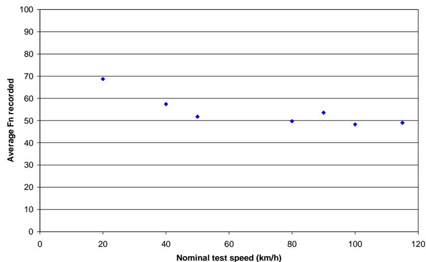
**Figure 8.12 Dry friction versus speed on the A511 (western section) two days after opening**
