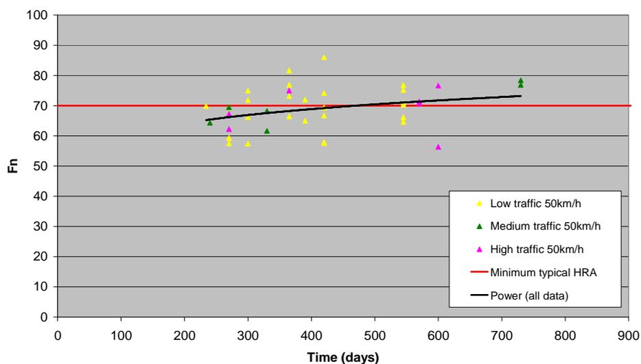
**Figure 8.15 Change in dry friction at 50km/h over time for surfacings from 6-18 months old**
