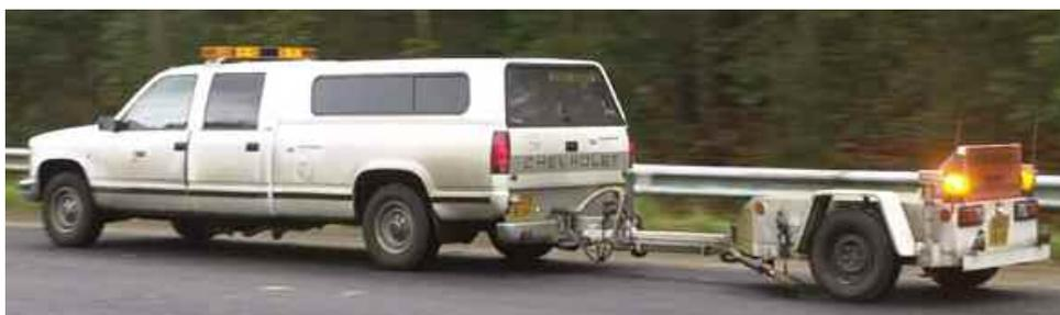
**Figure 4.2 The Pavement Friction Tester**
