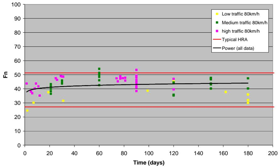
Figure 8.8 Change in wet friction at 80km/h over time for surfacings from 0-6 months old
