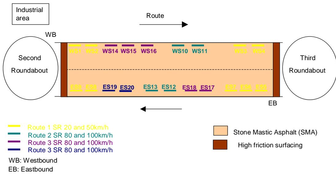
**Figure A2: Schematic plan, western section, A511**
