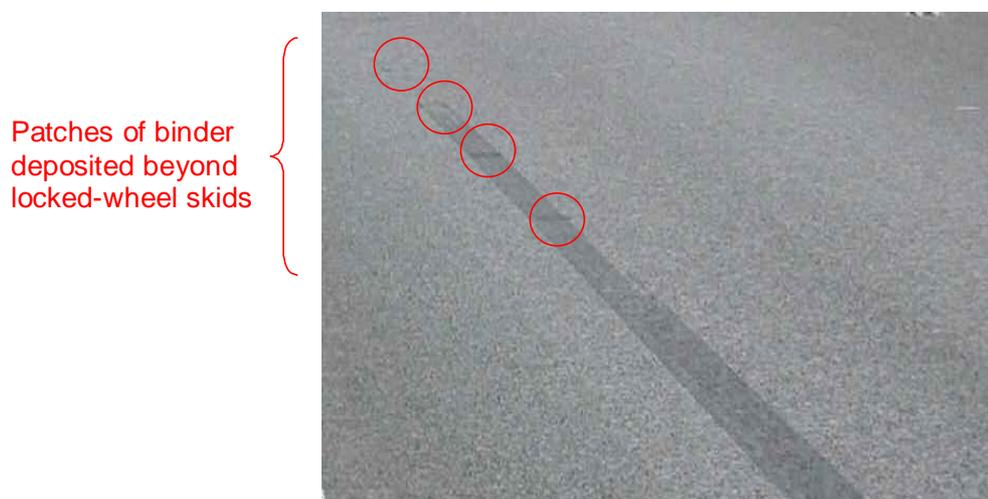
**Figure 9.2: patches of transferred binder visible at the end of a skid mark**
