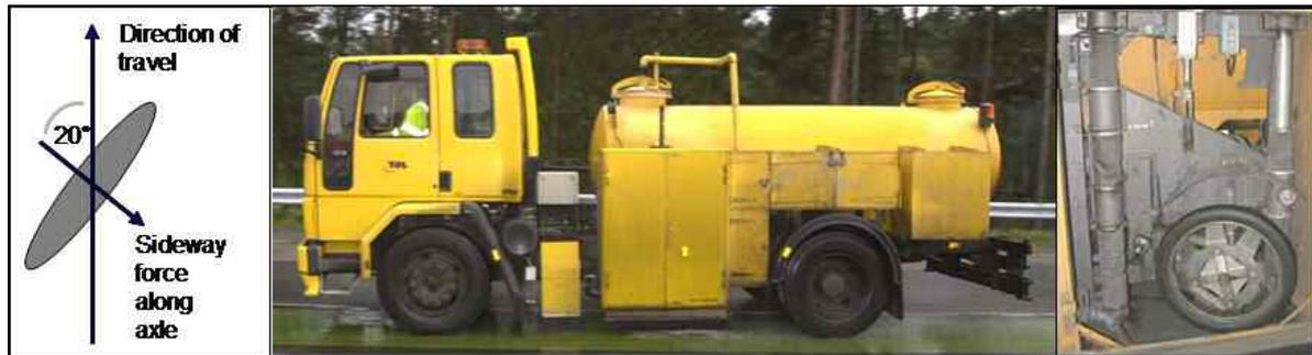
**Figure 4.1 SCRIM – principle and test wheel detail**
