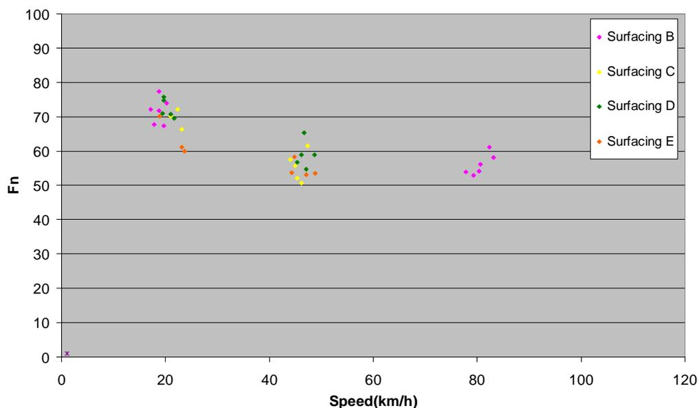
**Figure 8.2 Illustration of the scatter in replicate dry friction measurements using the PFT at different speeds on four different surfacings of similar age**
