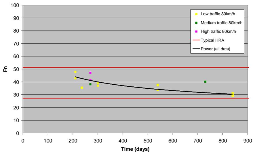
Figure 8.10 Change in wet friction at 80km/h over time for surfacings from 6-18 months old
