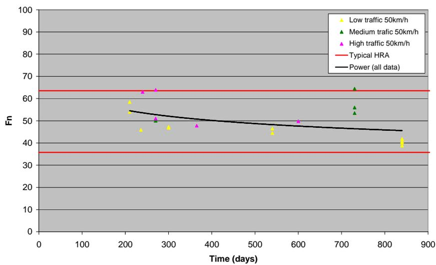
Figure 8.9 Change in wet friction at 50km/h over time for surfacings from 6-18 months old
