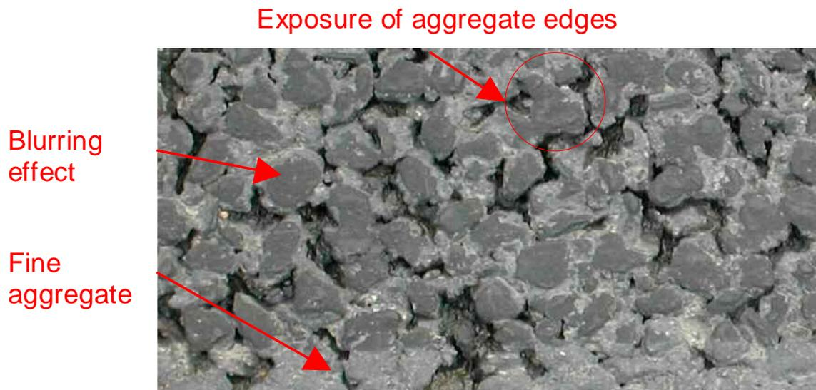
**Figure 9.3: Close-up of part of a dry skid mark**
