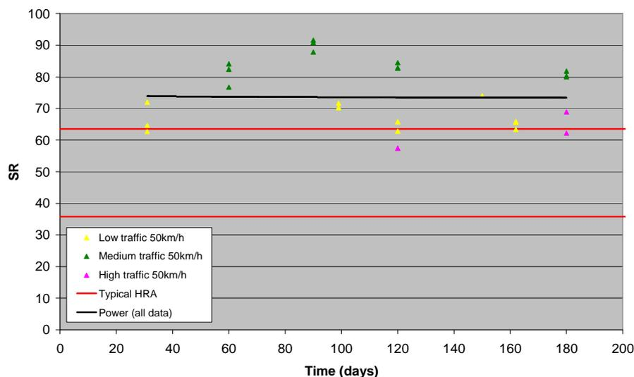
**Figure 8.5 Change in low-speed wet skid resistance (SR) over time for surfacings from 0-6 months old**
