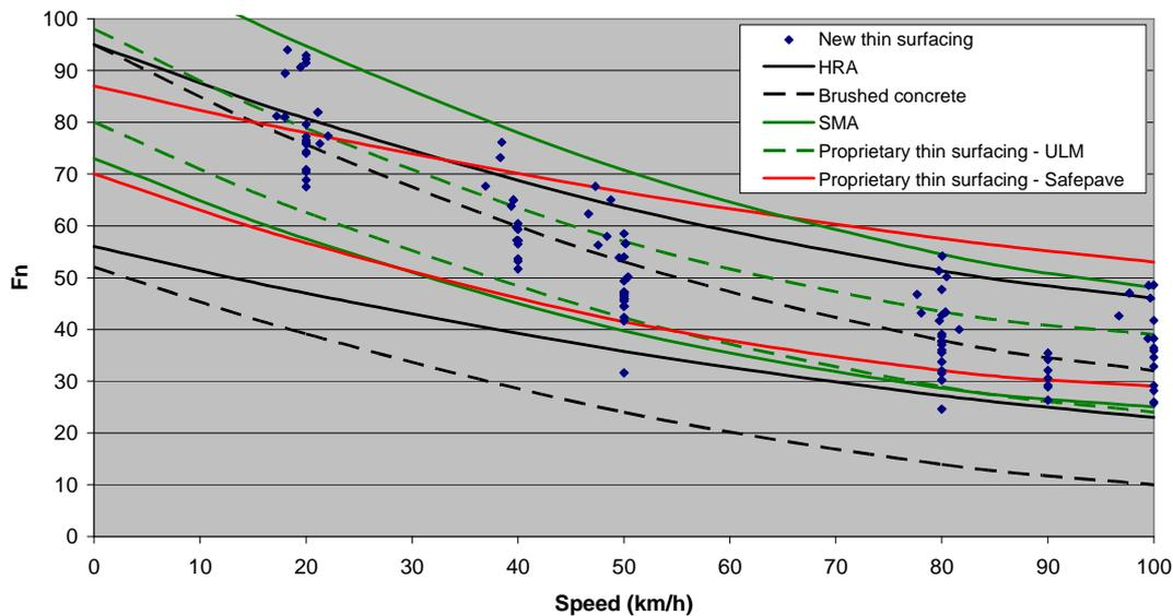
**Figure 8.4 Comparison of wet friction and speed for new thin surfacings with typical ranges for different types of well-trafficked surfacing**
