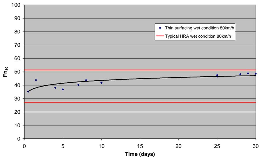
**Figure 8.11 Development of higher-speed wet friction in the first month on the M3 sites**
