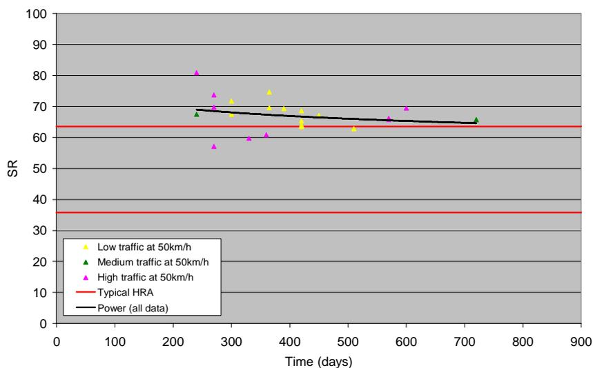
**Figure 8.6 Change in low-speed wet skid resistance (SR) over time for surfacings from 6-18 months old**
