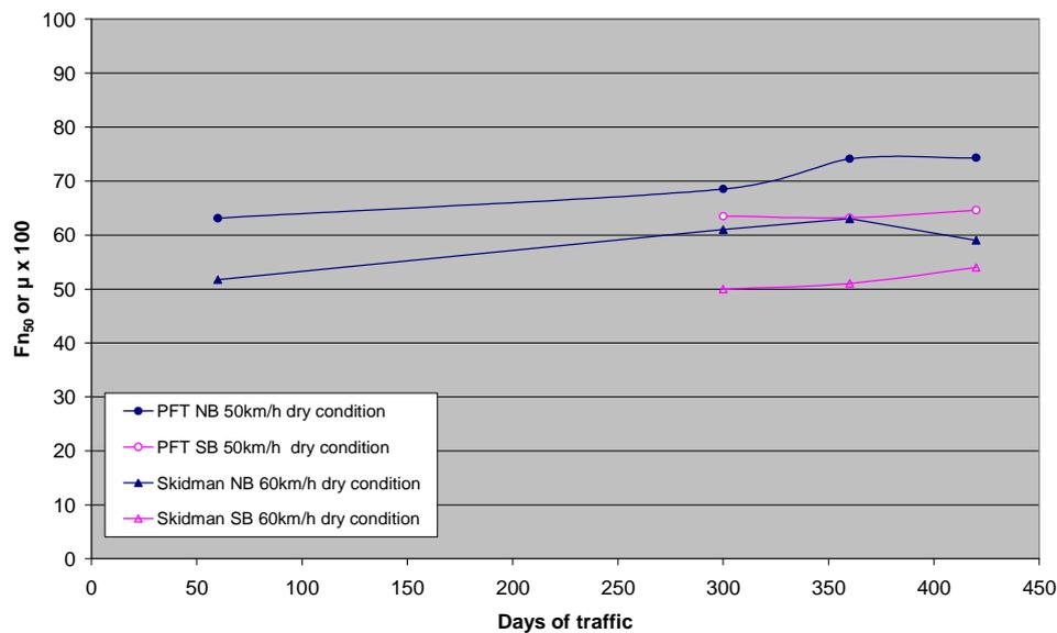
**Figure 8.17 Comparison between Skidman and PFT dry friction measurements on the A621**
