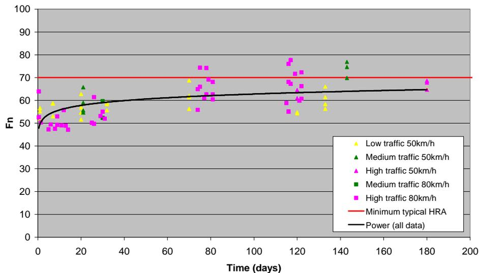
**Figure 8.14 Change in dry friction at 50 or 80km/h over time for surfacings from 0 - 6 months old**
