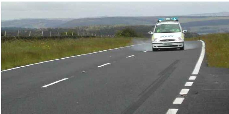
**Figure 4.3 Police car conducting a “Skidman” dry test**
