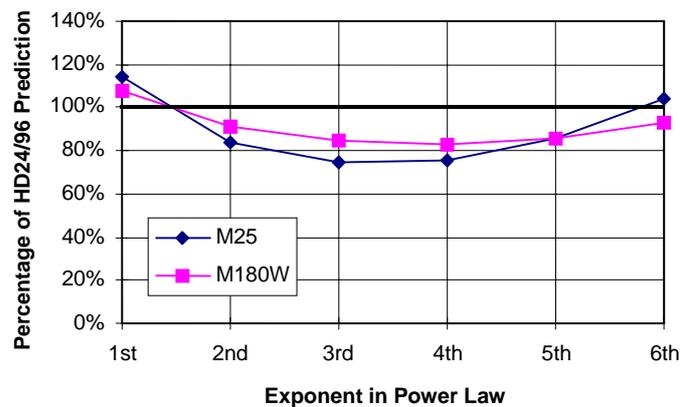
**Figure 4.1: Predicted Design Traffic using different exponents (expressed as a percentage of Design Traffic predicted using the HD24/96 method)**
