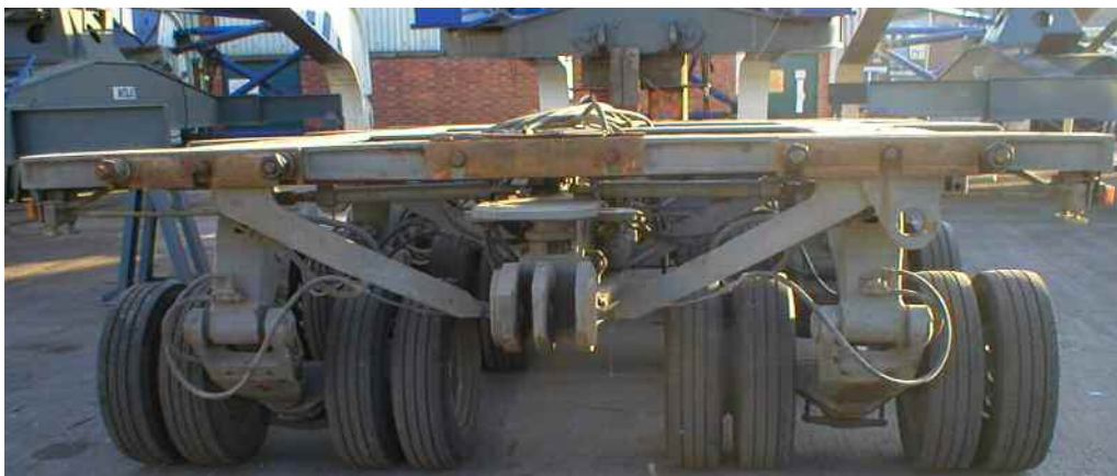
Figure 4.8 Trailer axle with four twin-wheel arrangements
