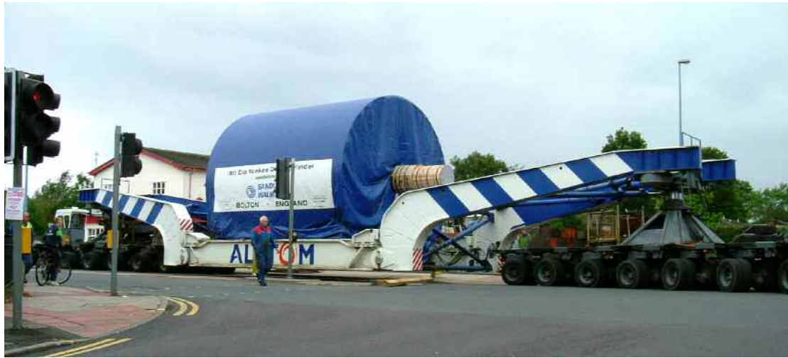
Figure A3 View of a girder frame vehicle with a close-up of the unloaded girder set
