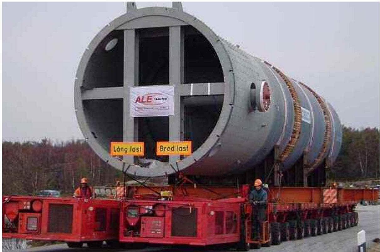
Figure A4 View of a self-propelled modular trailer
