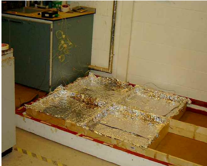
Figure 6. Slabs placed within a frame in groups of four and covered with aluminium foil
