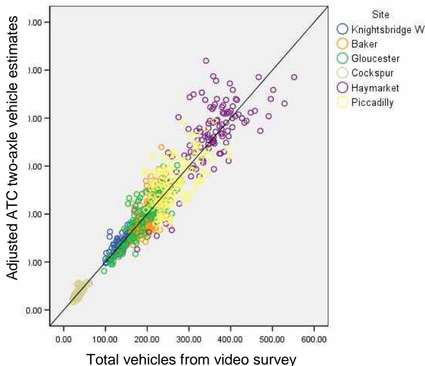
Figure 10: Total vehicles from video survey compared to Adjusted ATC estimates (each quarter hour)
