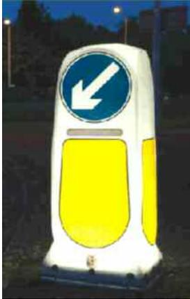
Standard type internally lit bollards have developed over the years and if installed correctly will now often survive impacts from vehicles and remain functional. If the bollard sustains damage and becomes deformed in shape then it can still operate to some extent. In the event of a severe impact, which shears the bollard from the base completely, the base light will still be operational and perform a similar function to a cat's eye.
