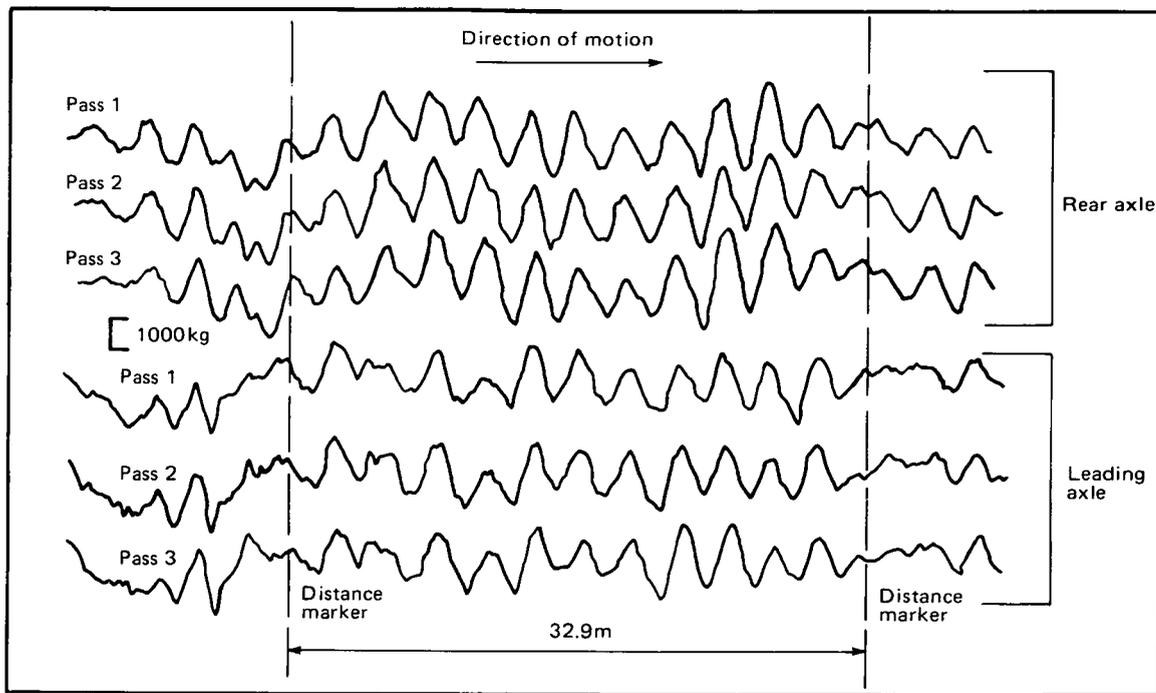
**Fig. 9 Measured axle load variations on a 2-axle semi-trailer at 32 km/h on the TRRL track showing repeatability (Static loads 9 tone/axle) (Addis, Halliday and Mitchell, 1986)**
