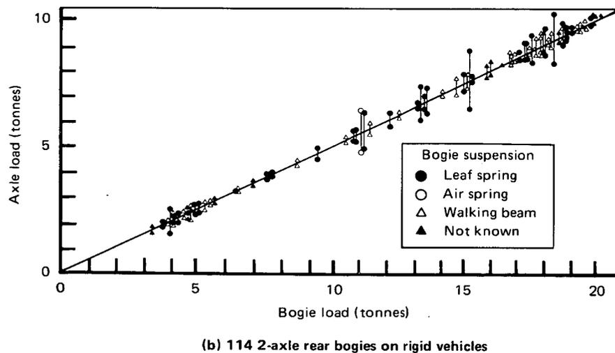
Fig. 2 Axle and bogie loads measured in a roadside survey on the M6 at Stafford, 1985
