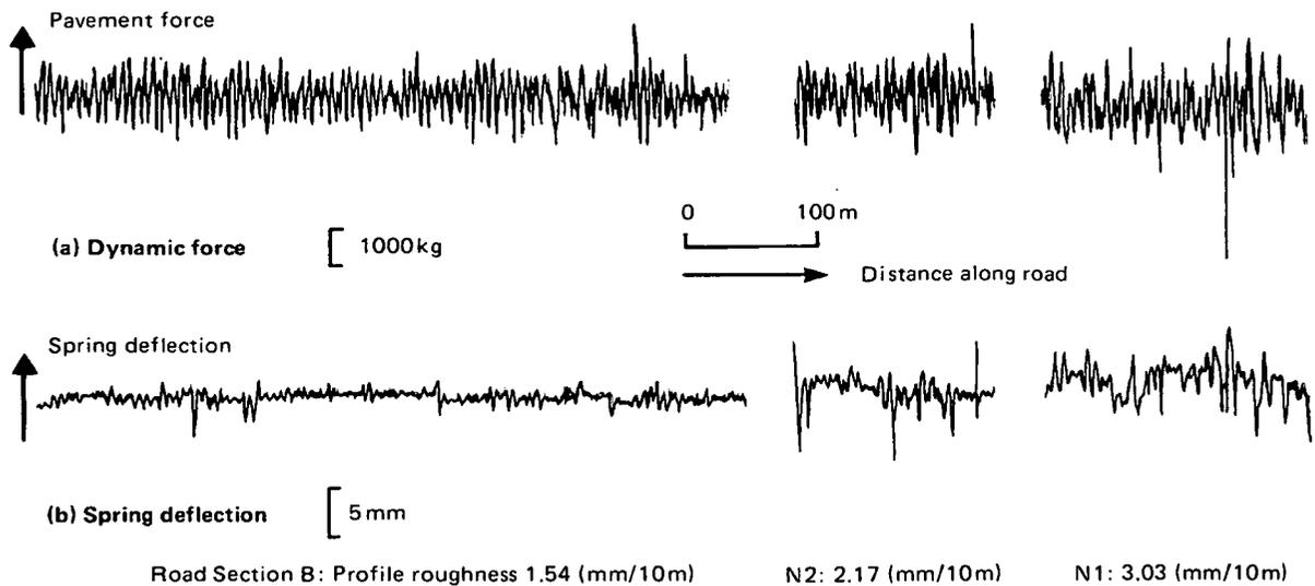
**Fig. 7 Dynamic pavement force and spring deflection vs. distance.**
