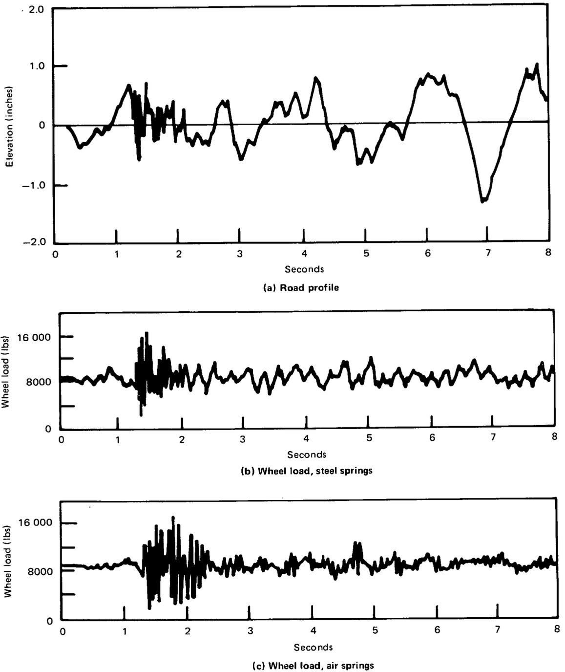
Fig. 10 Road loads under the offside rear wheel of a 2-axle semi-trailer on a defined road profile at 64km/h
