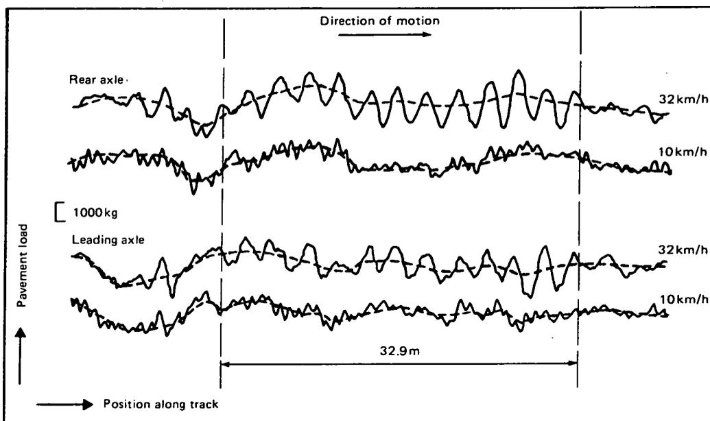
Fig. 4 Quasi-static load transfer between axles on a 2-axle semi-trailer bogie at 10km/h and 32km/h on the TRRL track
