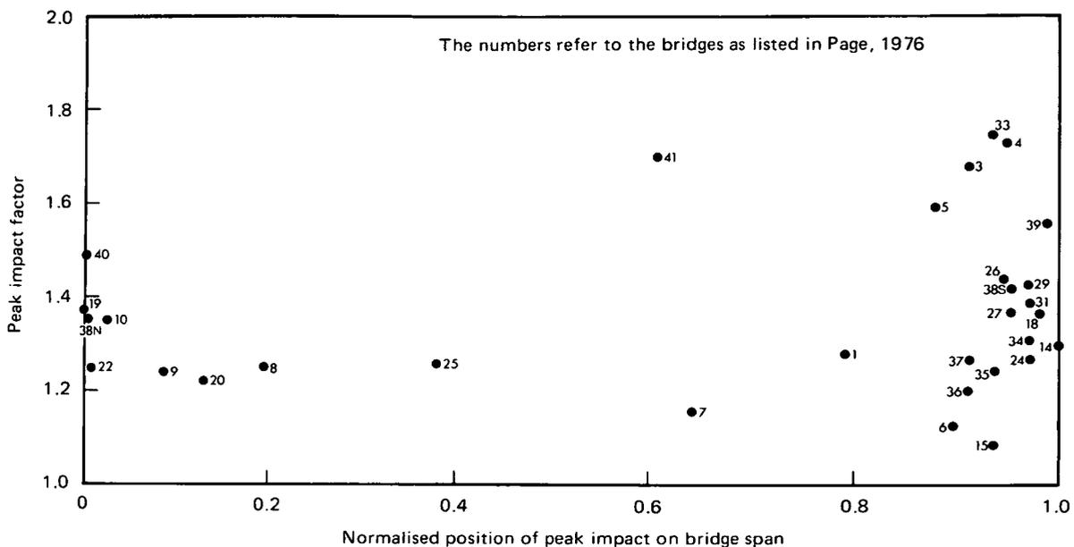
Fig. 6 Position on bridge where the peak impact occurs during a crossing by a 16tonne 2-axle goods vehicle (Page, 1976)
