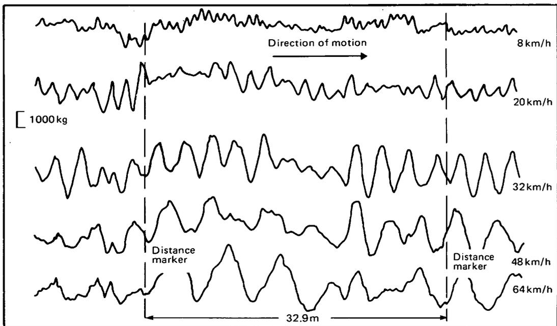
**Fig. 8 Measured dynamic pavement forces for the semi-trailer axle of a 3-axle articulated vehicle on the TRRL track (9tonne static axle load) (Addis, Halliday and Mitchell, 1986)**
