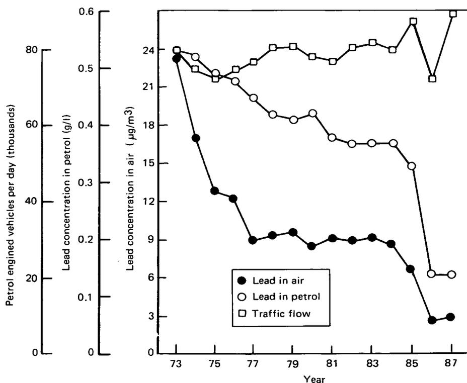
Fig. 3 Average lead in air, lead in petrol and flow of petrol engine vehicles
