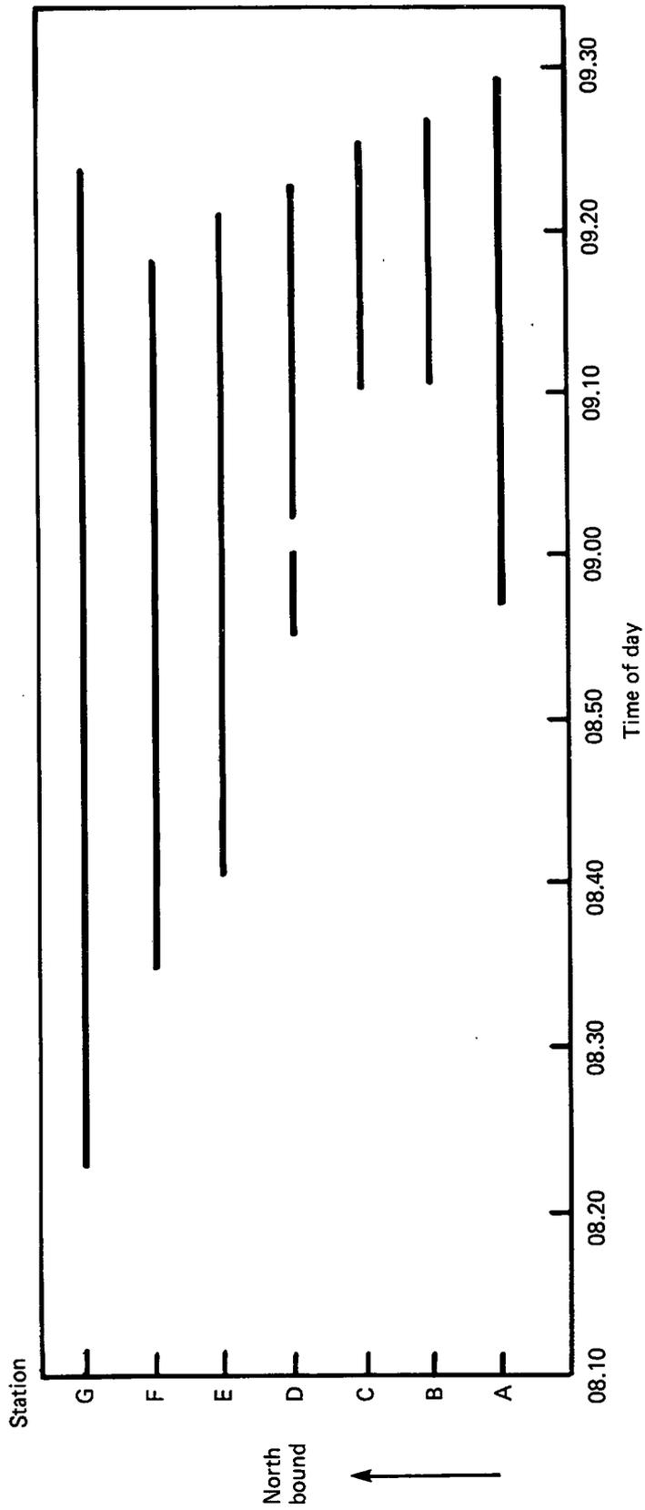
Fig. 4 Times of HIOCC alarm messages caused by an accident north of Station G (nearside lane only plotted)
