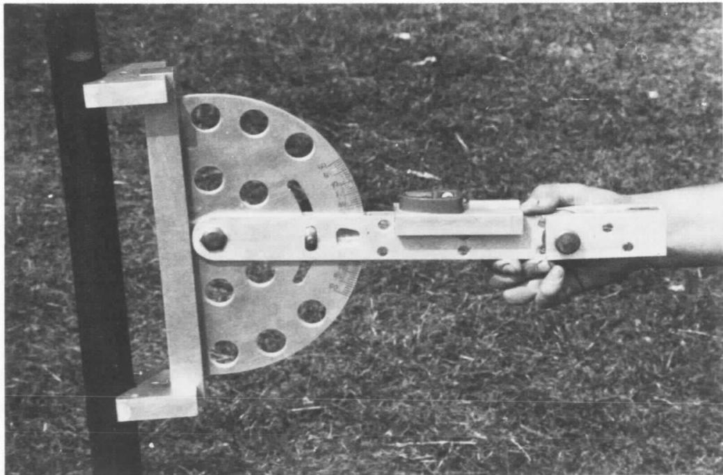
Plate 2 Simplified DOD with sighting prism
