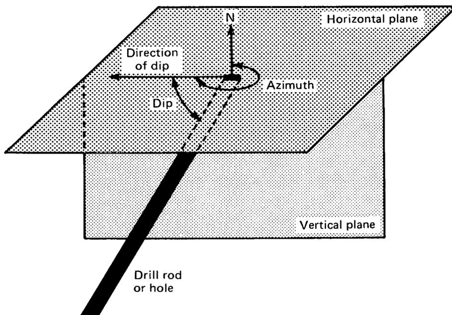
**Fig. 1** Measurement of drill rod or drill hole orientation
