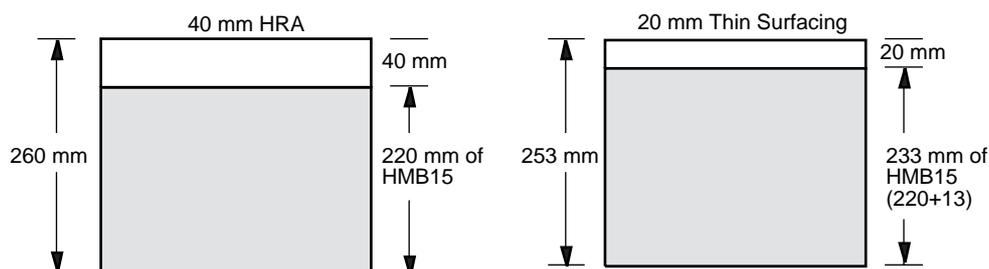
**Figure 3** Illustration of roadbase adjustment using a thin surfacing
