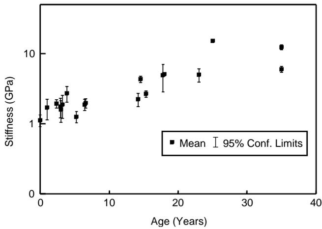
**Figure A9** Change in roadbase stiffness of in-service roads over time
