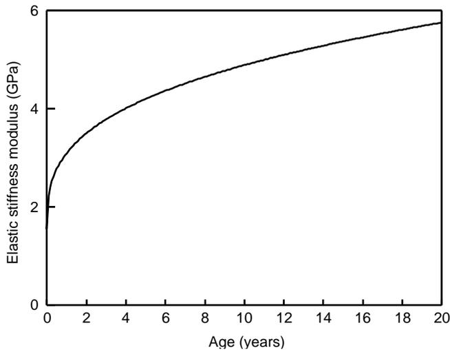
**Figure C2** Typical curing curve for macadam roadbase
