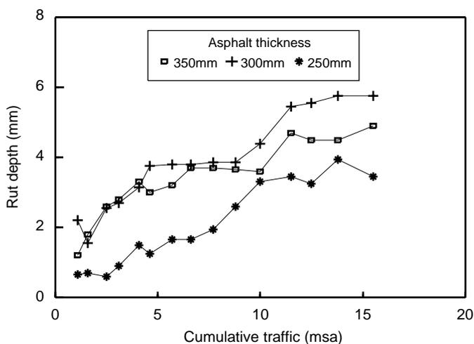
Figure A2 Rut development of experimental pavements
