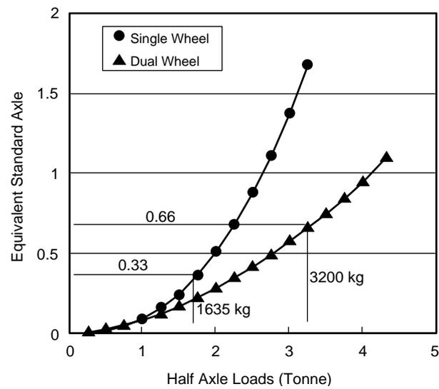
**Figure B8** Equivalence factors for different wheel loads
