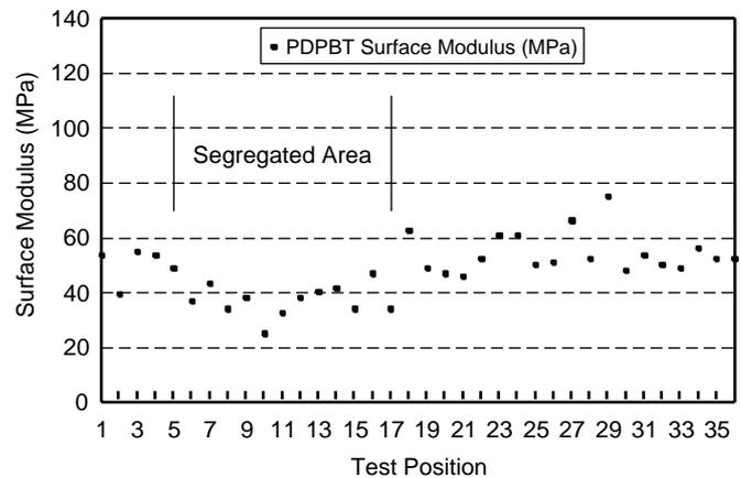
Figure B13 Stiffness at the formation (PDPBT results)
