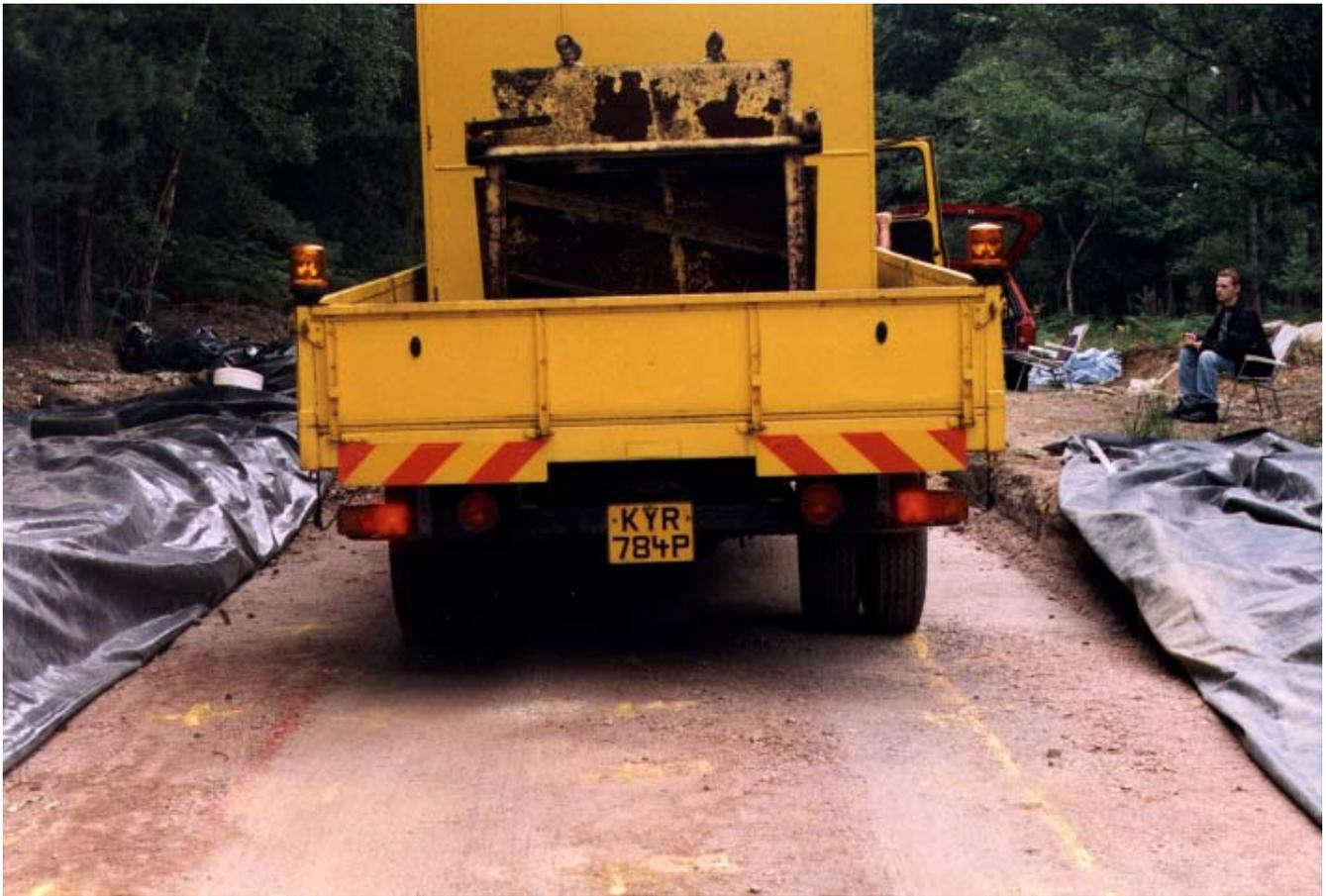
**Figure B7** Lorry used for trafficking the trial foundations
