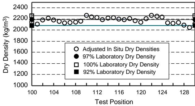
**Figure B14** In-situ dry density on the completed foundation
