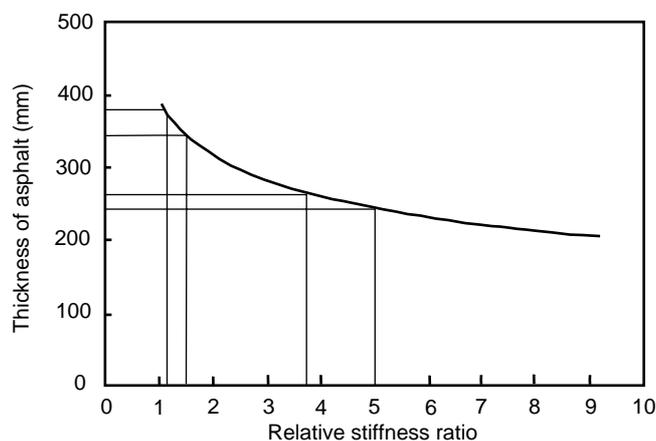
**Figure E2** Relative stiffness ratio versus asphalt thickness
