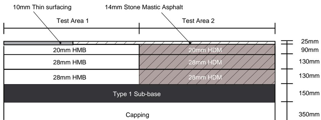
**Figure 6 Construction thicknesses in M65 trial**
