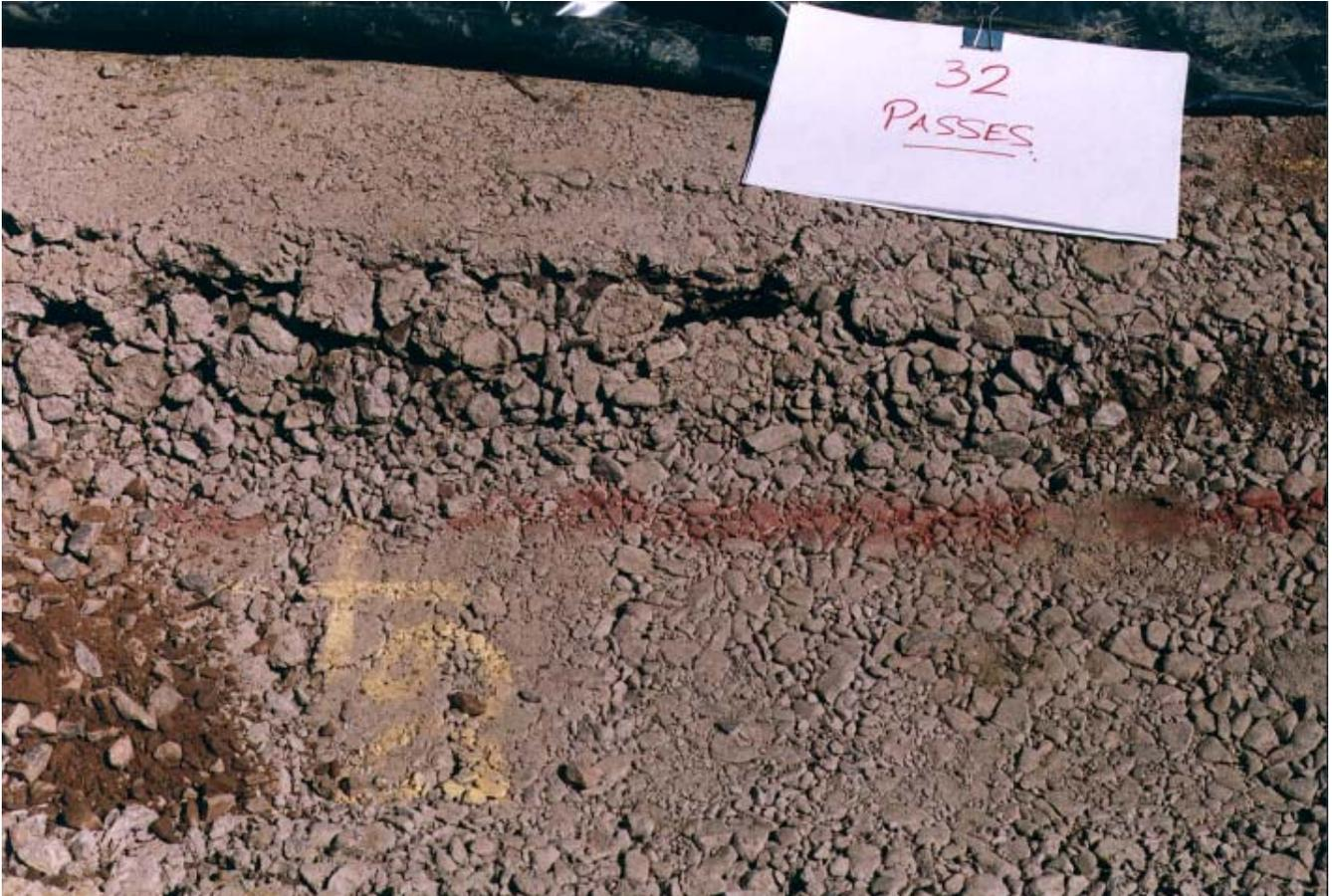
**Figure B10** Failure of Section D after 32 passes
