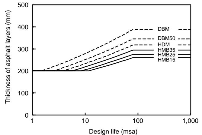
Figure 4 Design curve for high modulus roadbase (HMB)
