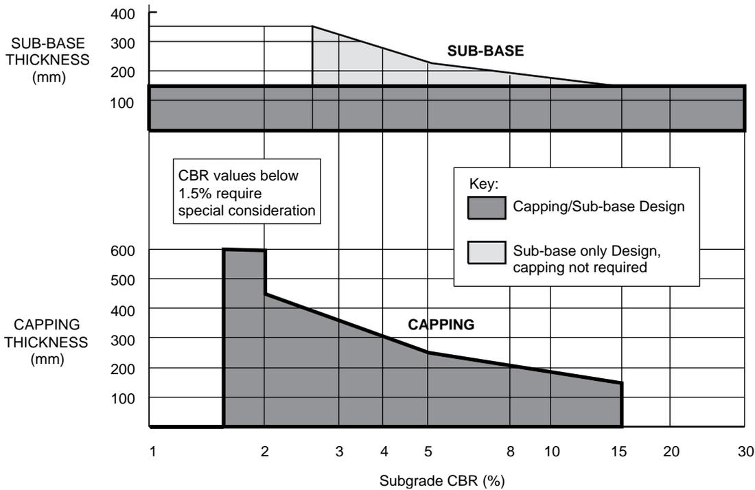
**Figure B1** Capping and sub-base thickness design
