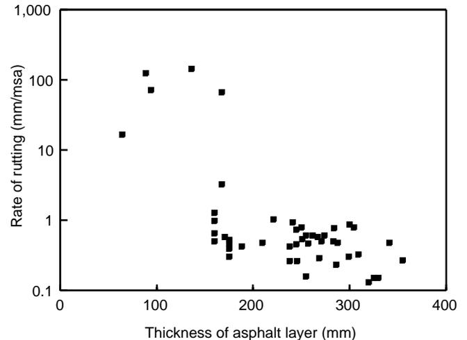
**Figure A3** Measured rate of rutting of trunk roads with DBM roadbase
