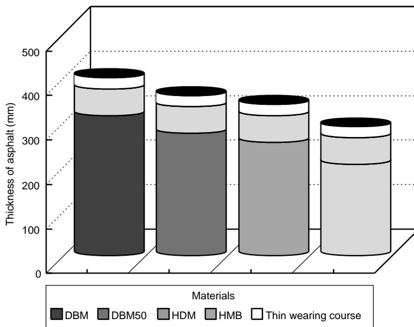
**Figure 5** Pavement designs to resist surface rutting
