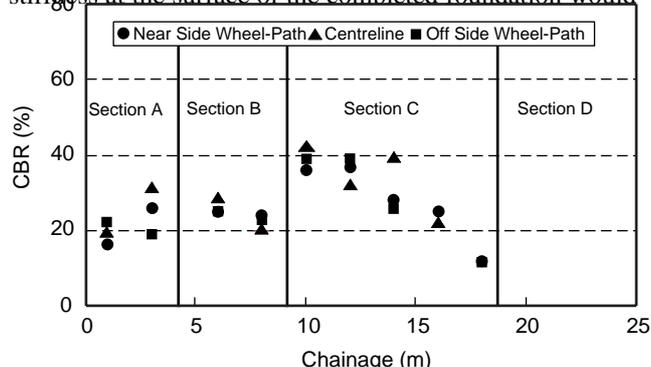
Figure B4 CBR results derived from DCP testing
