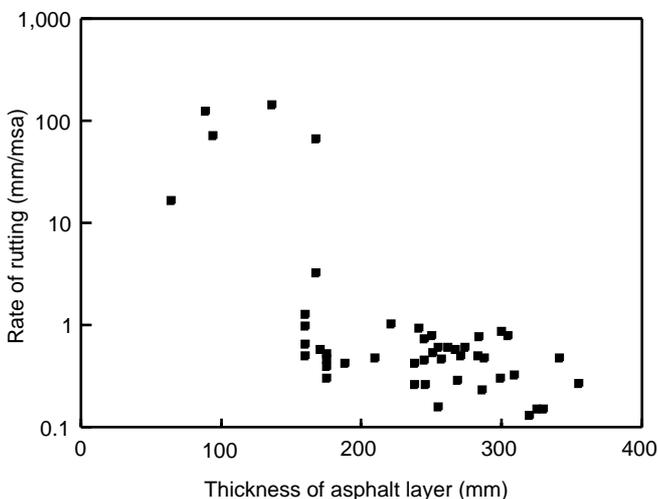
**Figure C1** Rate of rutting versus thickness of asphalt layer
