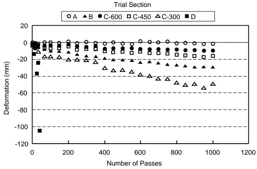
**Figure B9** Cumulative foundation deformation under trafficking
