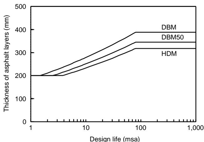
Figure C3 Design curve for roads with asphalt roadbase
