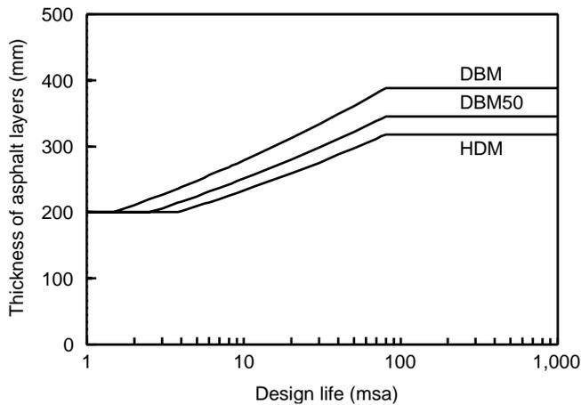
**Figure 2** Design curve for roads with asphalt roadbase
