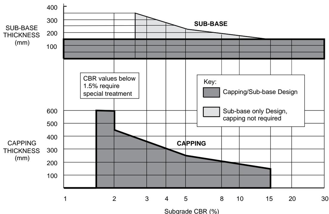
Figure 1 Capping and sub-base thickness design
