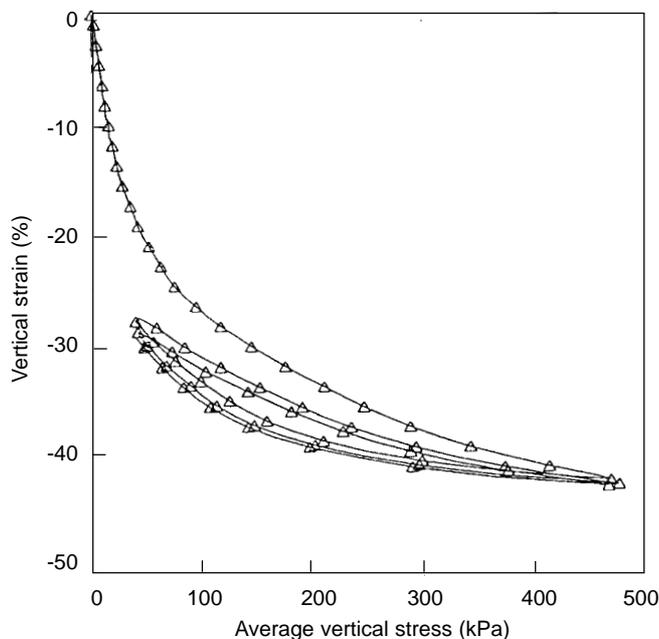
**Figure 14** Deformation of shredded tyres under cyclic loading (Humphrey et al, 1993)
