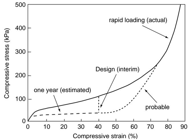
**Figure 4** Stress-strain behaviour of EPS at various strain rates (Horvath, 1995)
