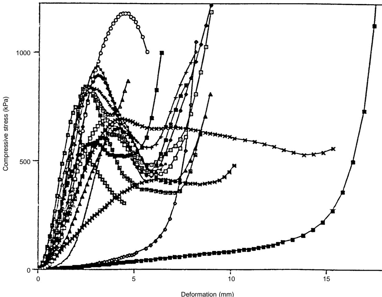
**Figure 8** Stress-strain curves for a variety of geocomposite drainage core products (after Geosynthetic Research Institute, 1995)
