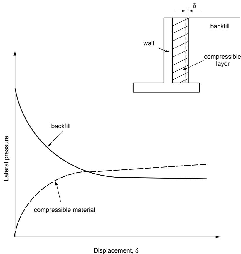
**Figure 1** Design principle using a compressible layer (after Horvath, 1995)
