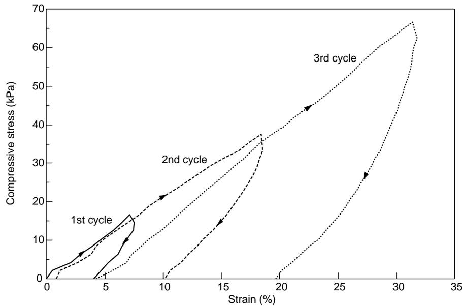
**Figure 6** Effect of three consecutive loading cycles on elasticised expanded polystyrene (standard grade)
