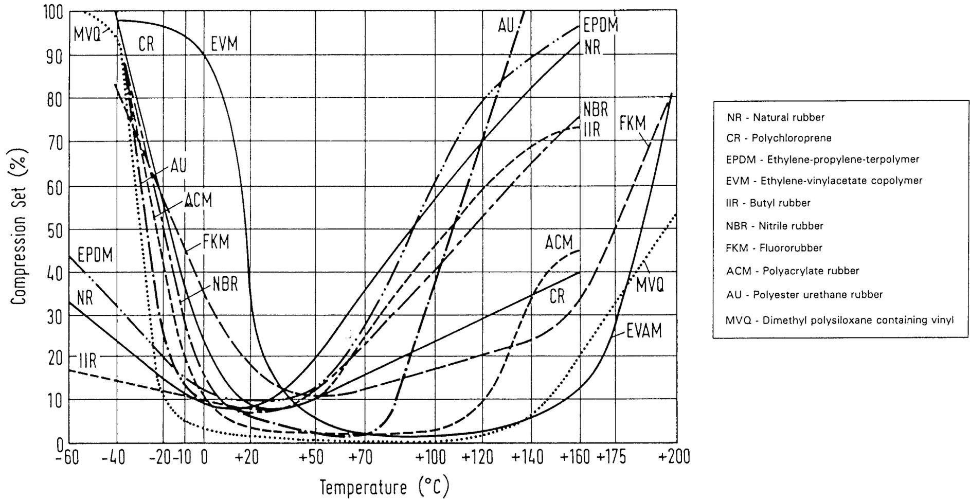
**Figure 10** Compression set of some rubbers versus temperature (Hoffman, 1980)
