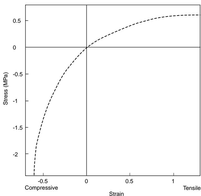
**Figure 9** Uniaxial extension and compression curve for rubber (after Freakley and Payne, 1978)
