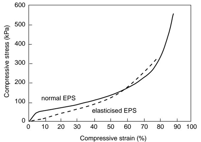
**Figure 5** Comparison of stress-strain behaviour in uniaxial compression of EPS and elasticised EPS (Horvath, 1995)
