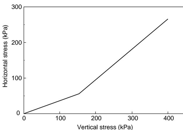
Figure 13 Horizontal stress against vertical stress for shredded tyres (Newcomb and Drescher, 1994)
