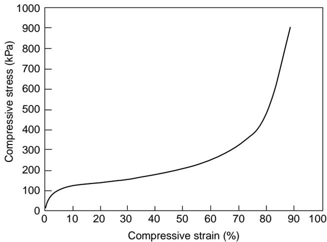
**Figure 2** Typical stress-strain behaviour of EPS under uniaxial compression (Horvath, 1995)
