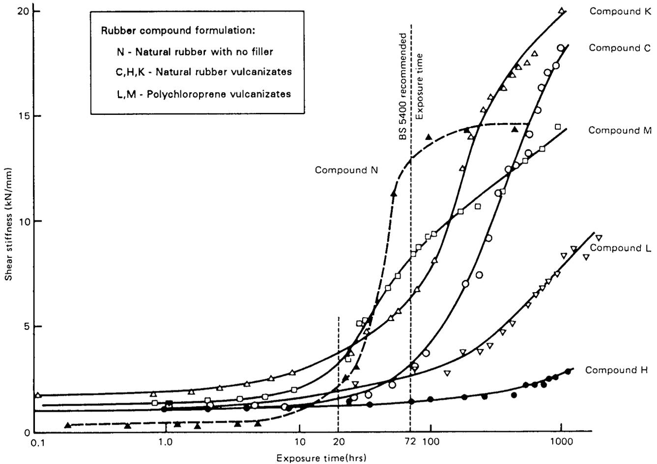
Figure 11 Increase in stiffness of full-size rubber bearings at -25°C (Eyre and Stevenson, 1991)
