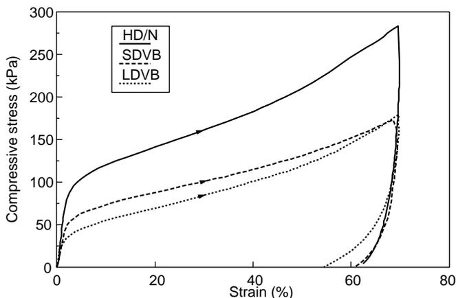
**Figure 3** Stress-strain behaviour of different grades of EPS
