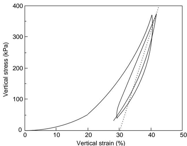
Figure 12 Vertical stress against vertical strain for shredded tyres (Newcomb and Drescher, 1994)
