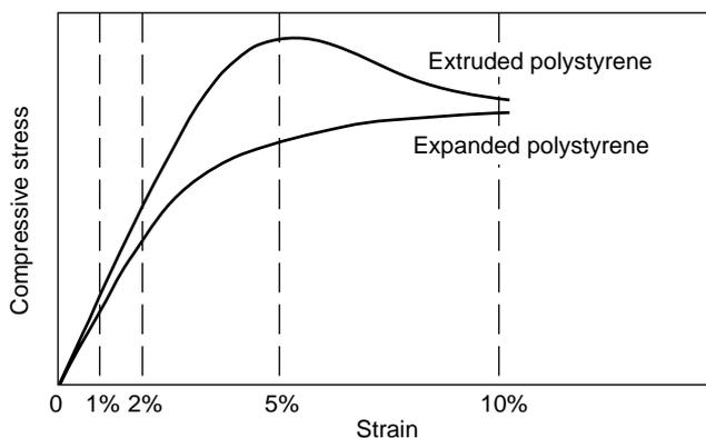
**Figure 7** Typical stress-strain curves for expanded and extruded polystyrene (Sanders and Seedhouse, 1994)
