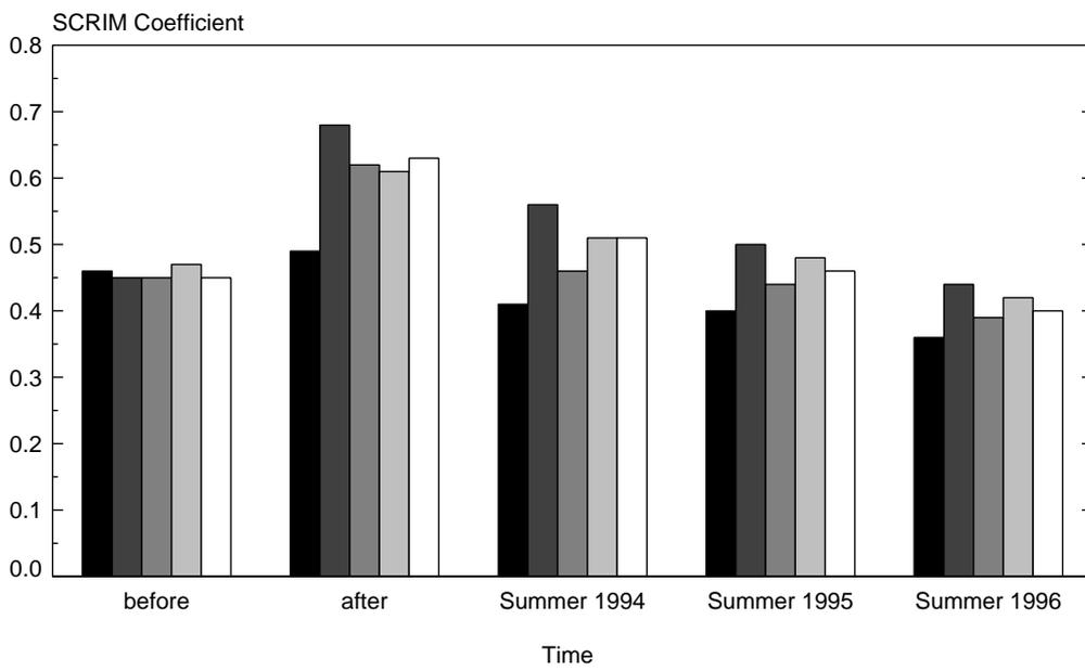
control      scabbling      bush hammering      orthogonal grooving      shot blasting
