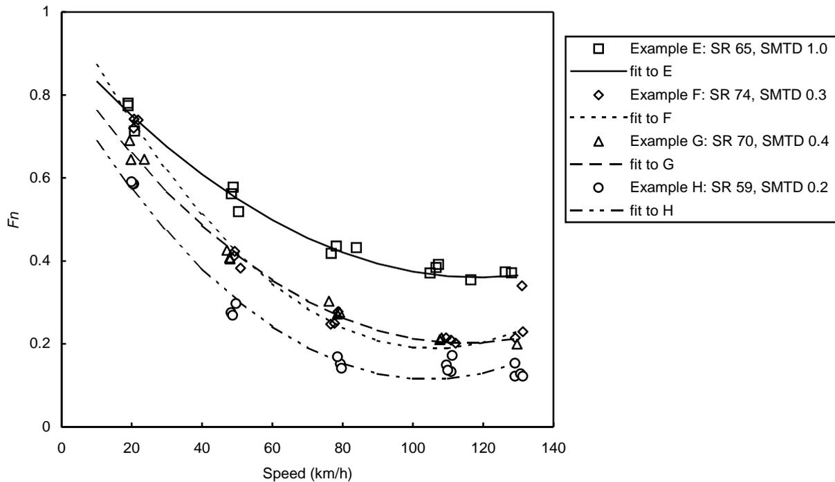
**Figure 6** Examples of friction versus speed curves from transverse-textured surfacings
