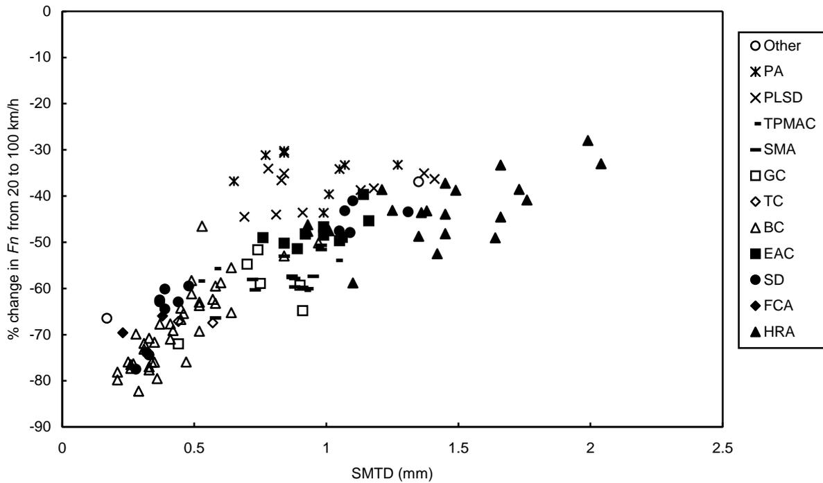
**Figure 13** The effect of texture on the relative change in friction between 20 and 100km/h
