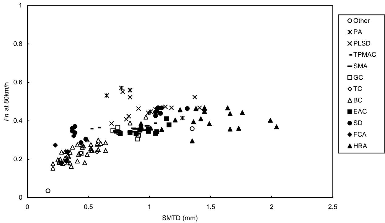
**Figure 10** Relationship between locked-wheel friction and texture depth at 80km/h
