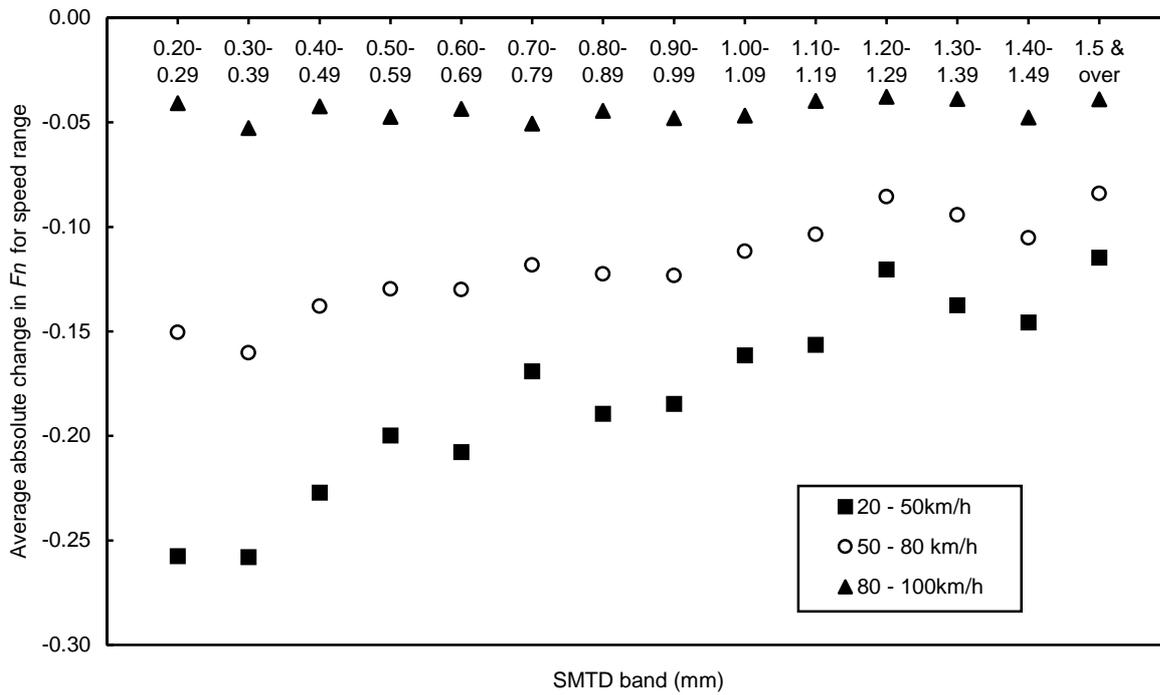
Figure 15 Effect of texture depth on absolute change in friction as speed is increased
