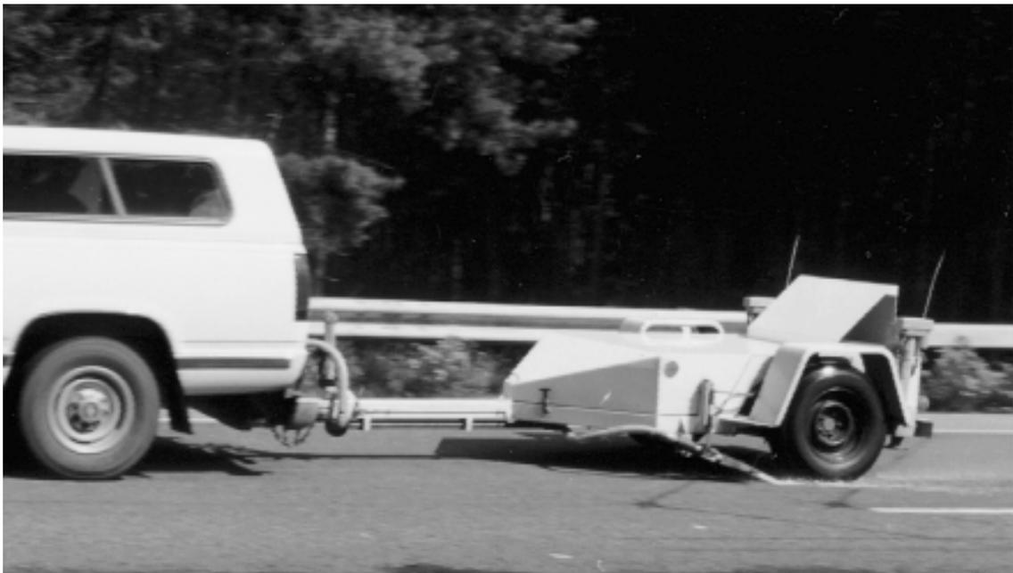
b Side view, carrying-out a wet locked-wheel test (trailer wheel not rotating while vehicle is moving)
