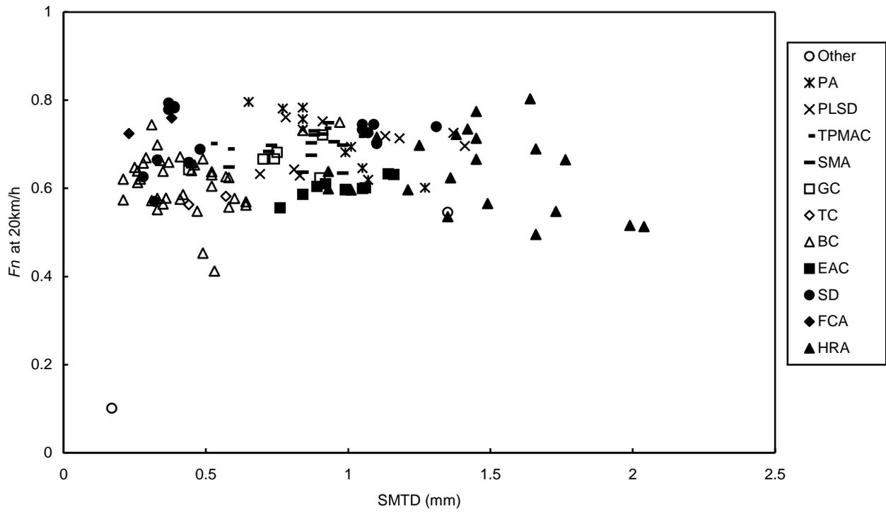
**Figure 8** Relationship between locked-wheel friction and texture depth at 20km/h
