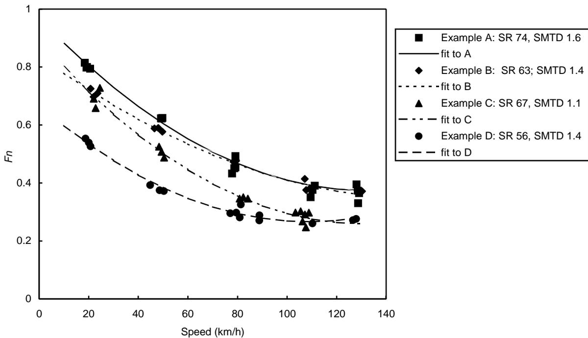
**Figure 5** Examples of friction versus speed curves from random-textured surfacings
