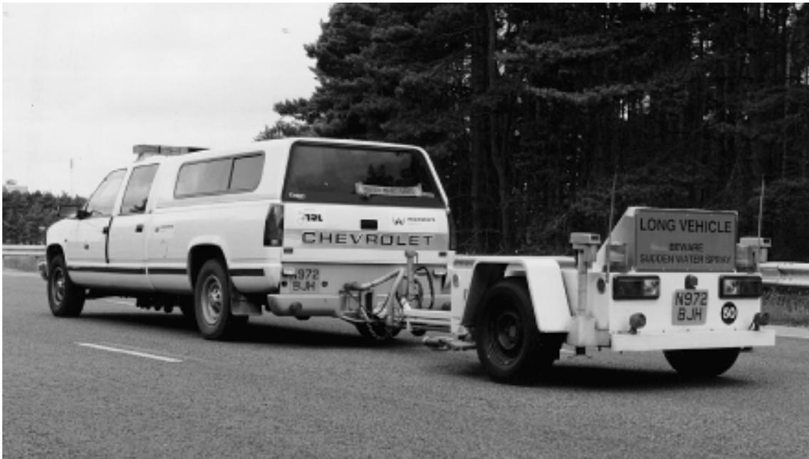
a Rear view showing trailer with water nozzle in 'parked' position
