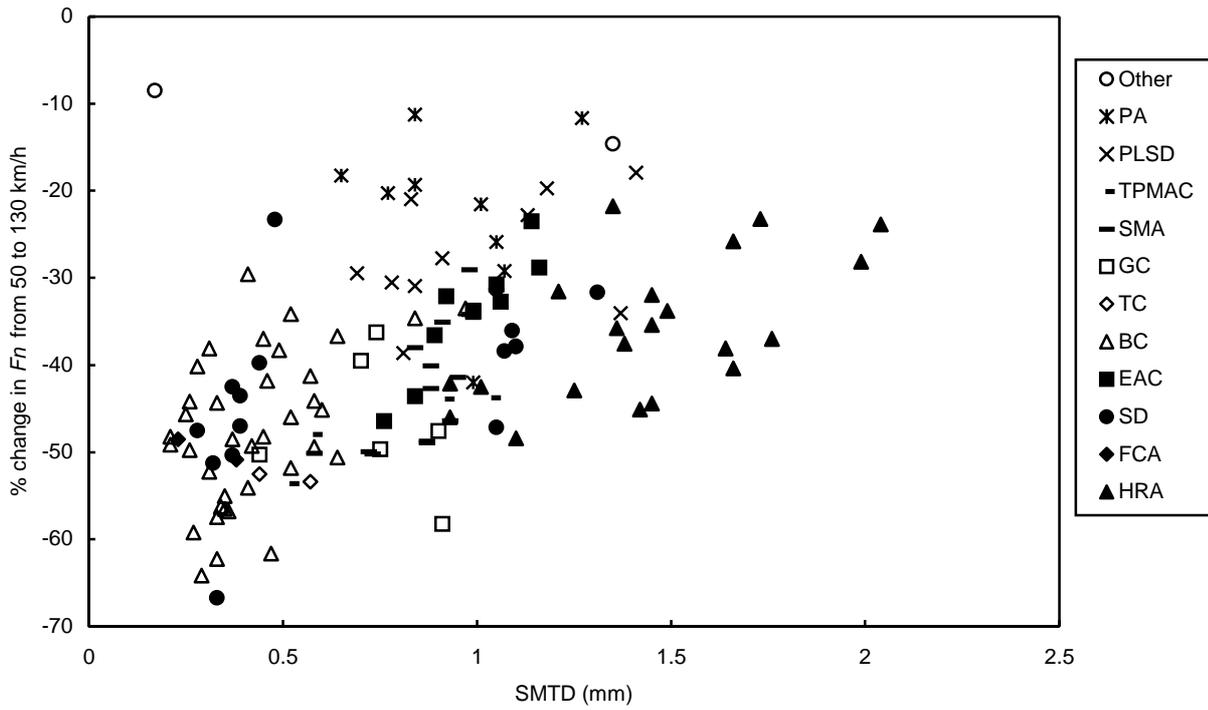
**Figure 12** The effect of texture on the relative change in friction between 50 and 130km/h
