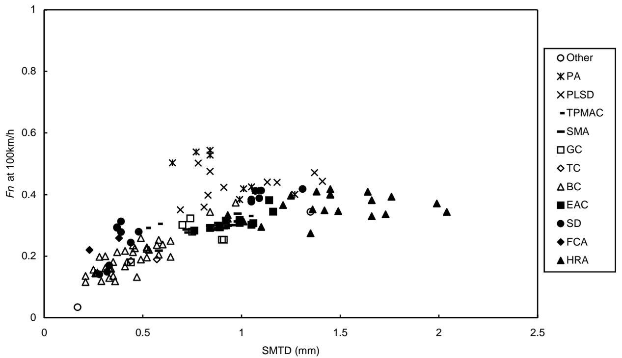
**Figure 11** Relationship between locked-wheel friction and texture depth at 100km/h
