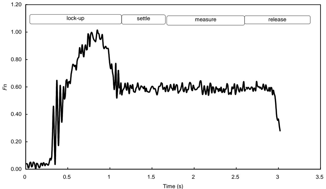
**Figure 2** Graphical representation of the results from a typical locked-wheel braking cycle
