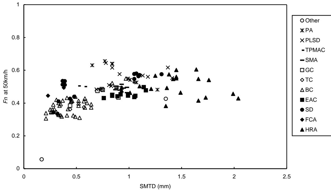
**Figure 9** Relationship between locked-wheel friction and texture depth at 50km/h
