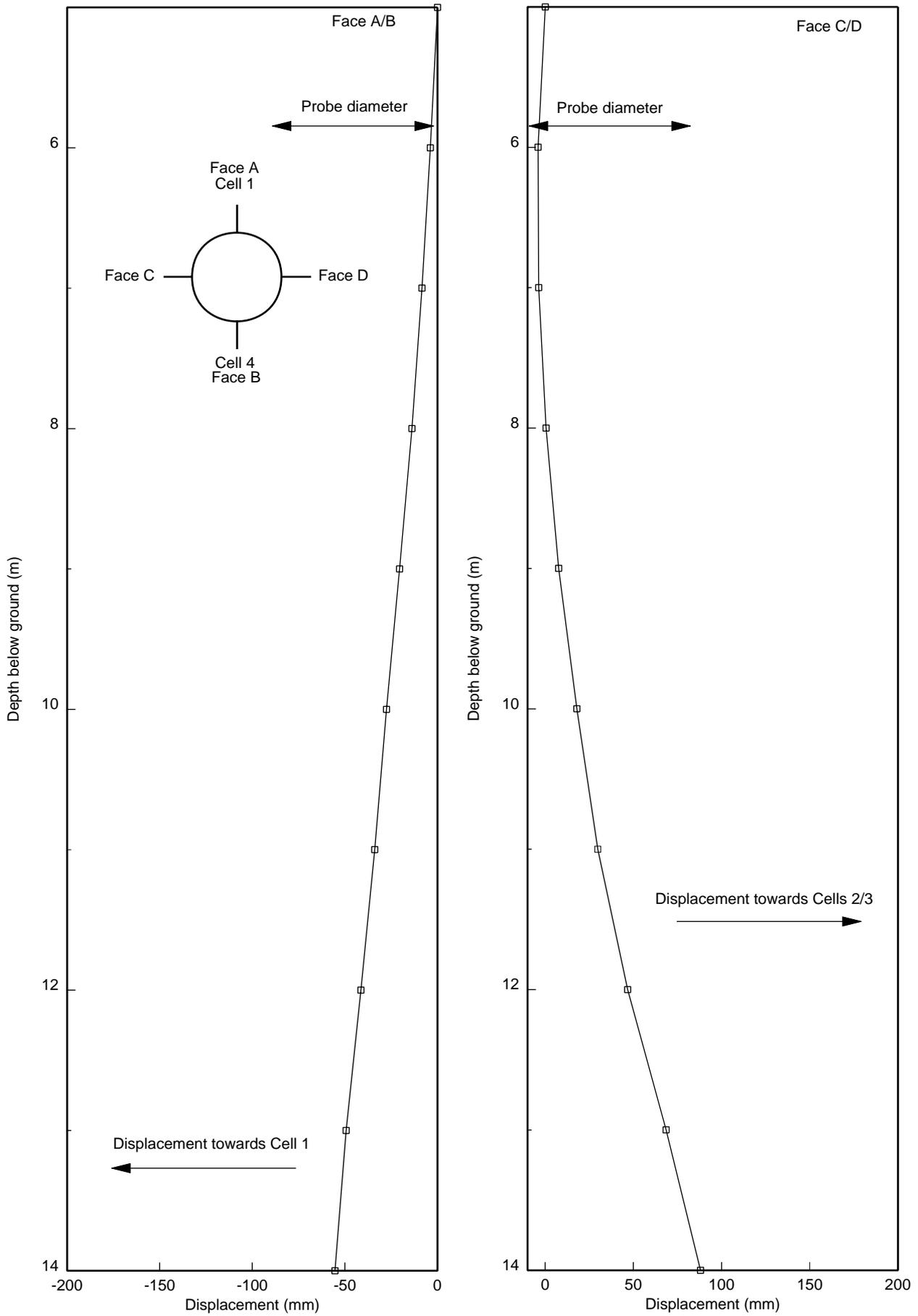
**Figure 2** Lateral displacement profiles of test hole
