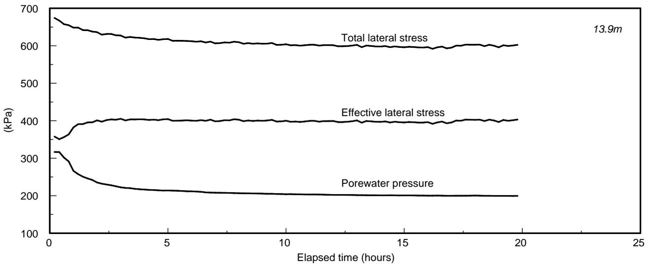
**Figure 3(c)** Test results at 11.9m, 12.9m, 13.9m below ground level
