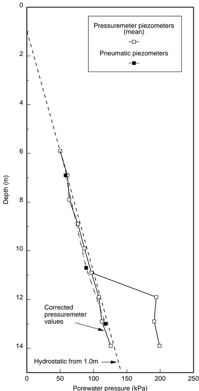
**Figure 6** Profiles of porewater pressure with depth
