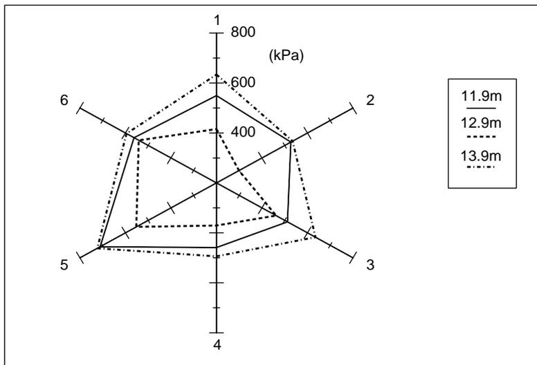
**Figure 5** Total lateral stress distribution around the probe
