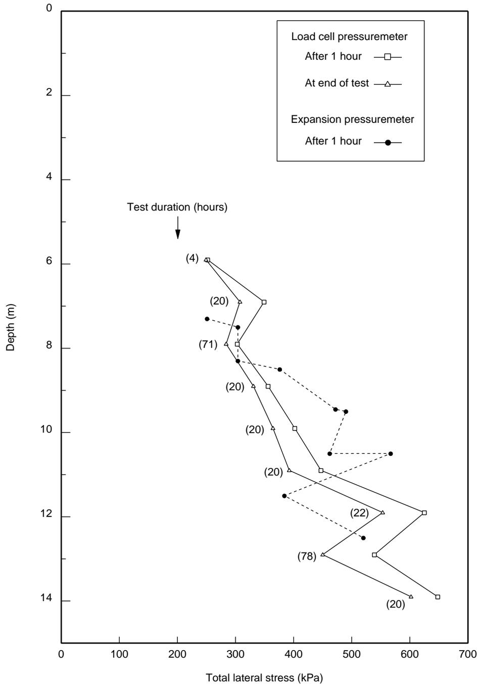
**Figure 4** Profiles of lateral stress with depth
