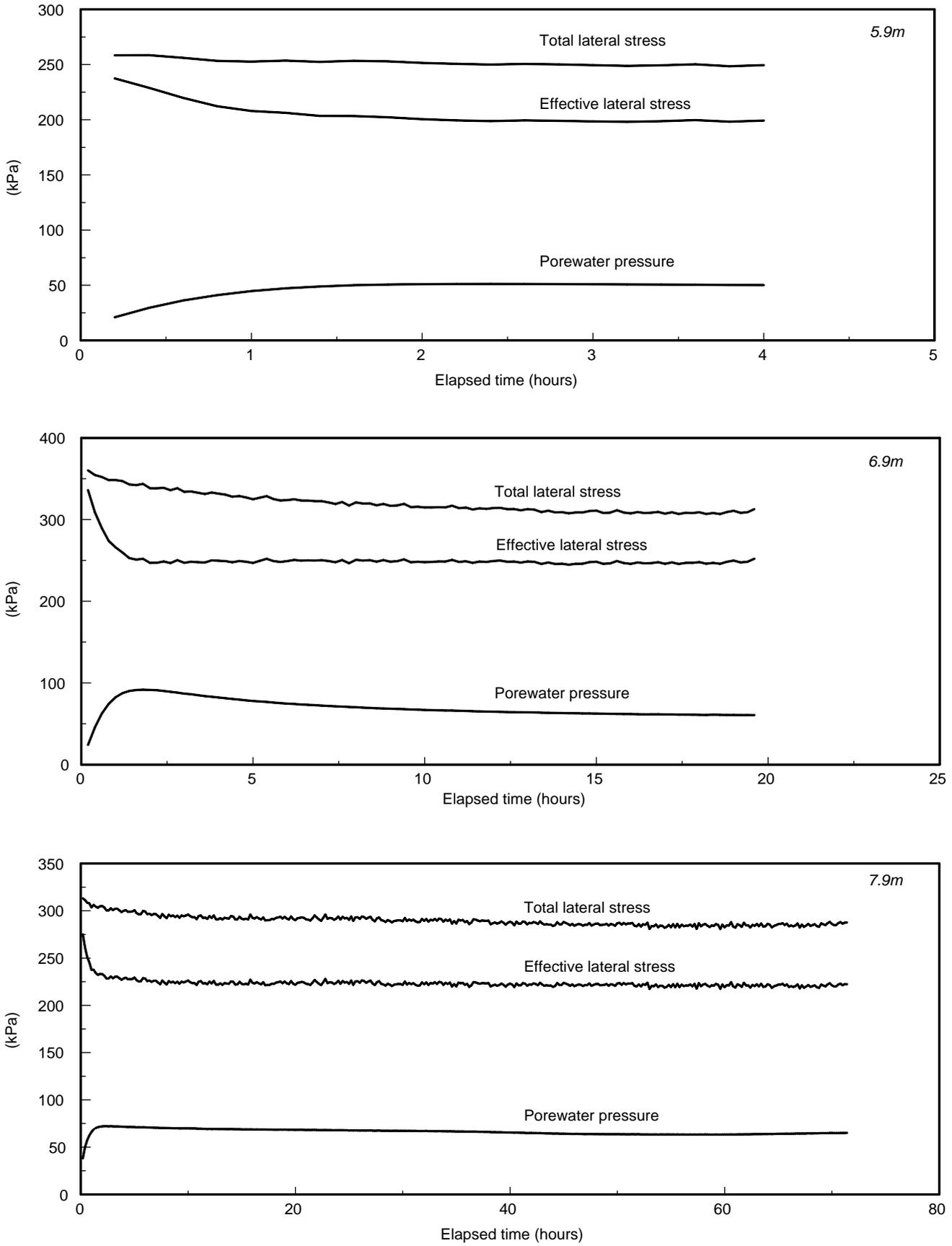
**Figure 3(a)** Test results at 5.9m, 6.9m, 7.9m below ground level
