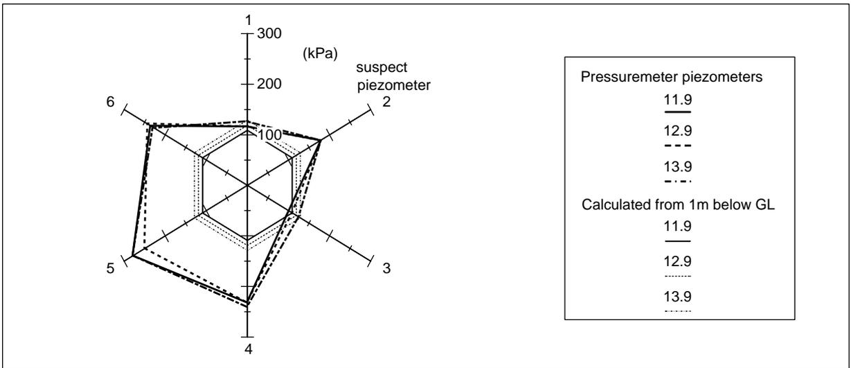
Figure 7 Porewater pressure distribution around the probe
