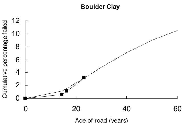
**Figure A12** Boulder Clay slope failures in cutting
