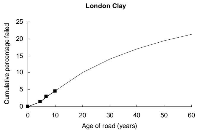
**Figure A24** London Clay on embankment
