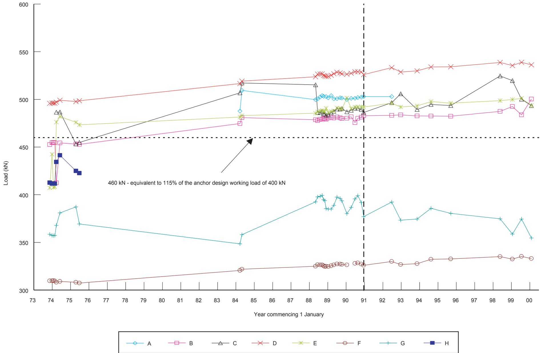
Figure 14 Variation of measured loads in ground anchorages
