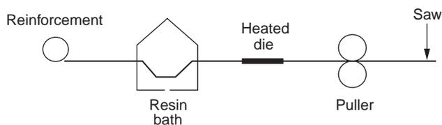
**Figure 2** Illustration of the pultrusion process
