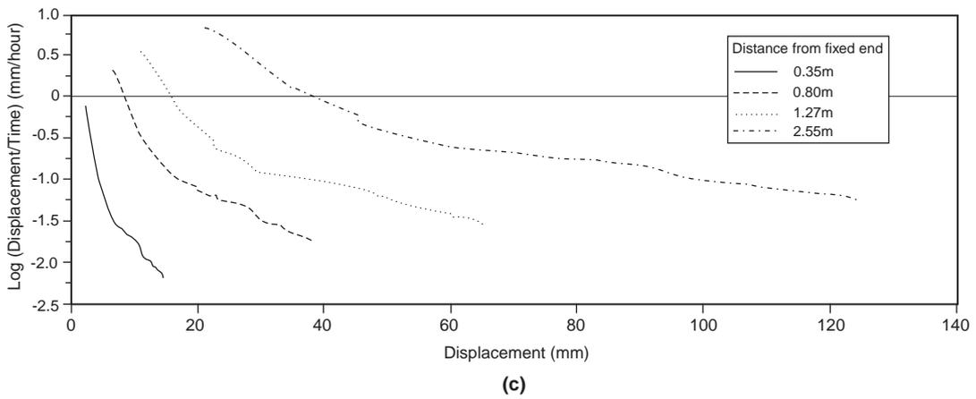
**Figure 11** Creep under sustained load equivalent to 2.55m of cohesive backfill
