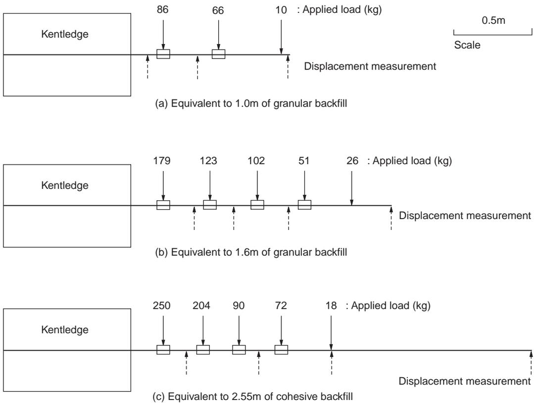
**Figure 8** Loading arrangement for creep tests
