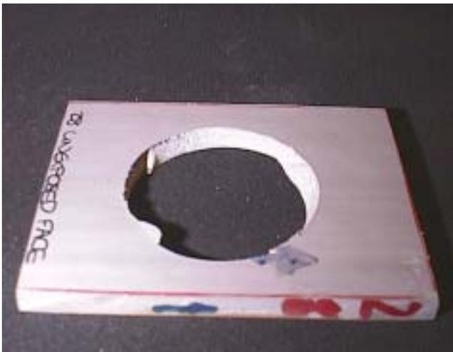
**Figure 5** 4000 hour sample showing brittle impact failure
