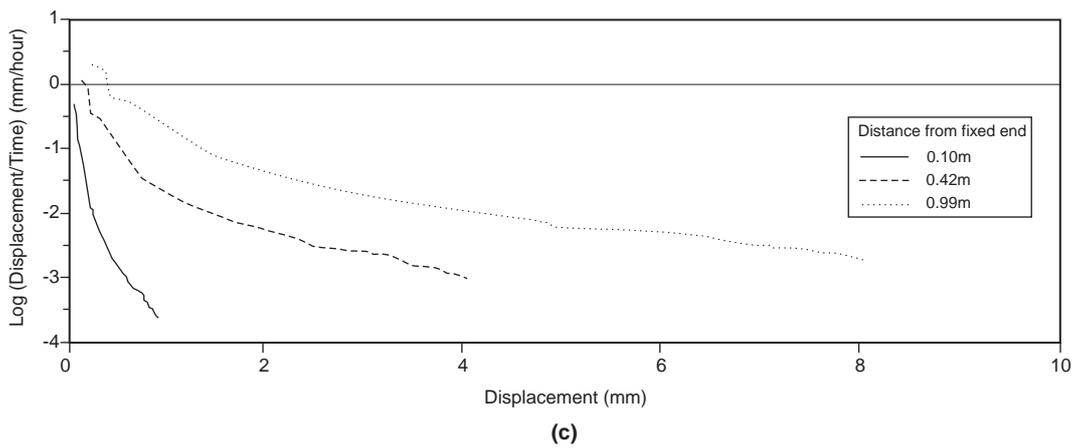
**Figure 9** Creep under sustained load equivalent to 1.0m of granular backfill
