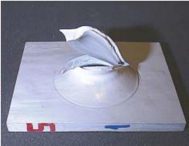
**Figure 4** Un-aged sample showing ductile impact failure
