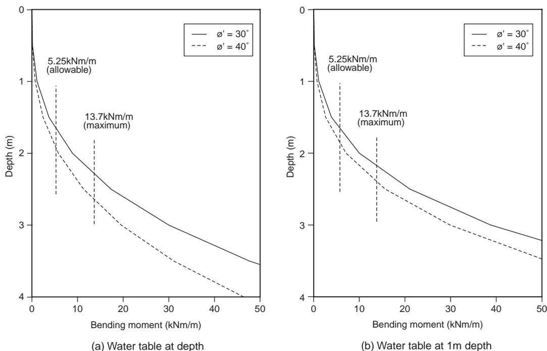
**Figure 6** Bending moment in granular soil
