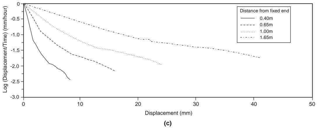
**Figure 10** Creep under sustained load equivalent to 1.6m of granular backfill
