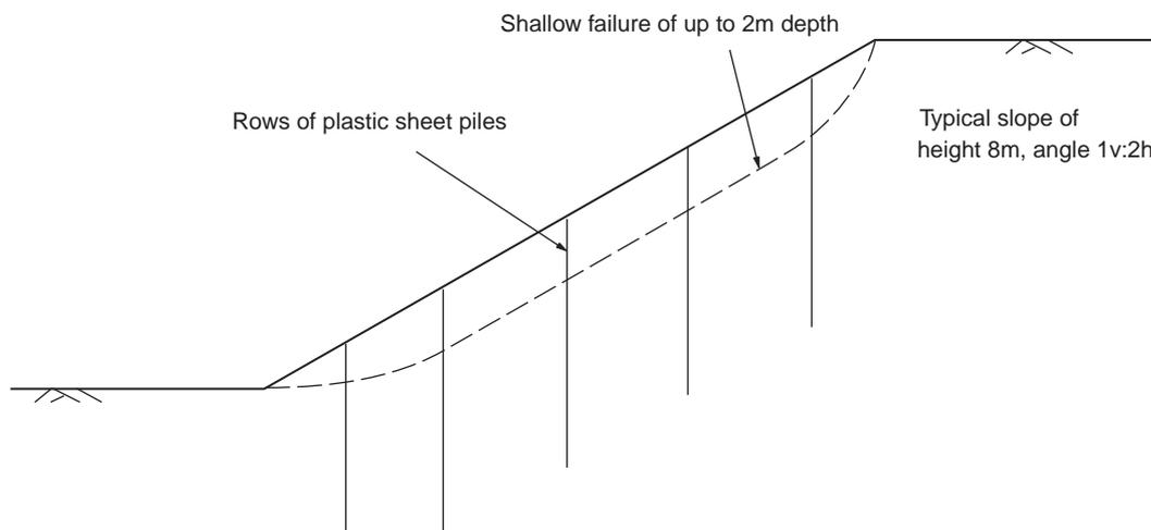
Figure 14 Stabilising a clay slope against shallow failure
