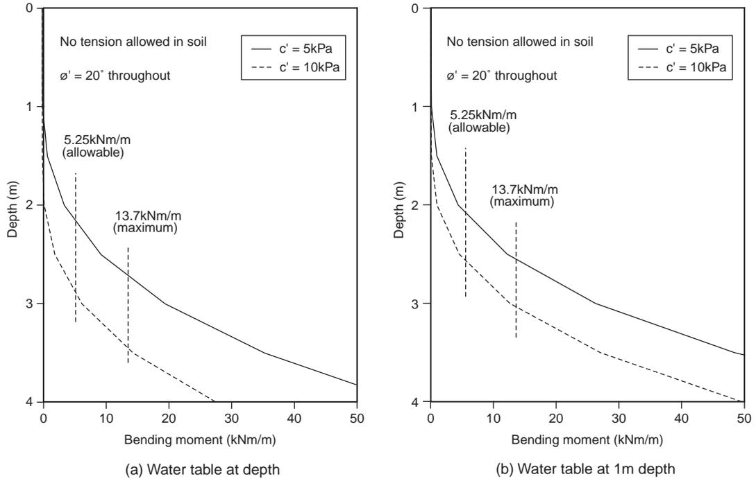
**Figure 7** Bending moment in cohesive soil
