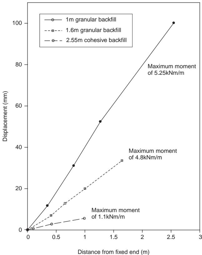
**Figure 12** Comparison of creep test results at 1000 hours
