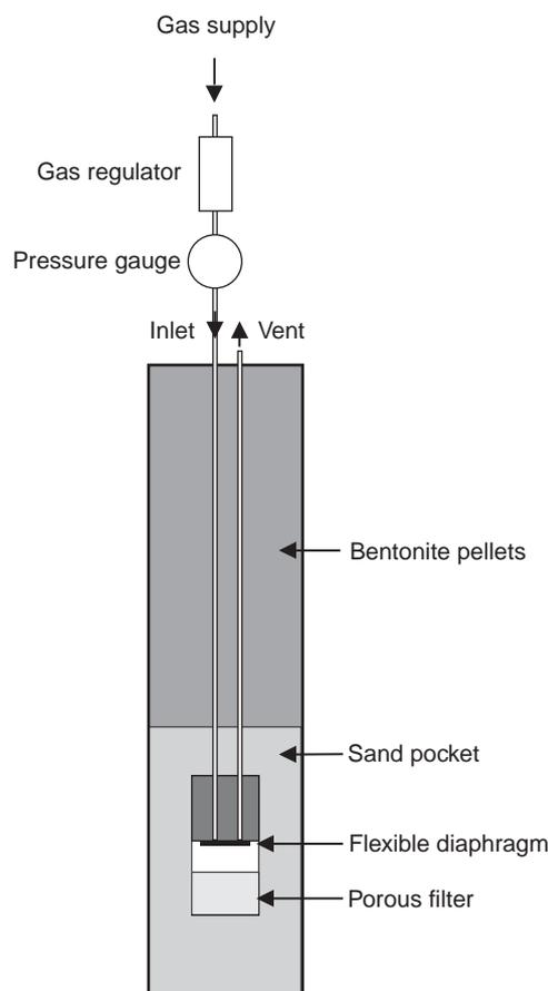
**Figure 13** Arrangement of a pneumatic piezometer
