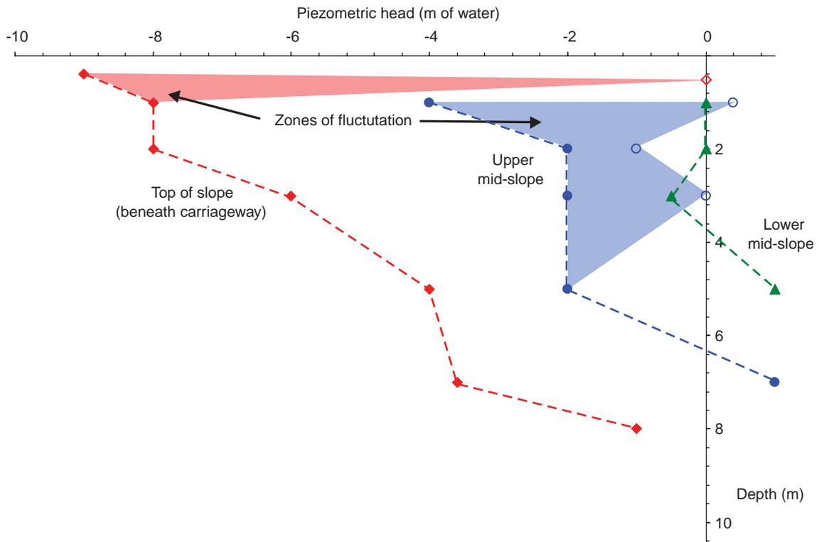
**Figure 8** Pore water pressures measured at Cambridge Northern Bypass
