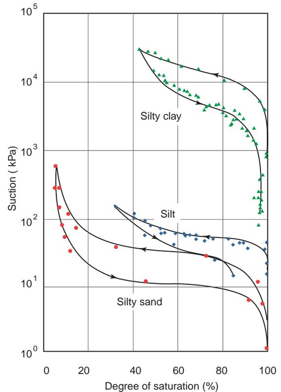
**Figure 4** Typical soil-water characteristic curves
