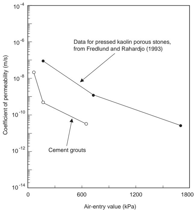
**Figure 28** Data on the air entry values of ceramic filters and cement grouts
