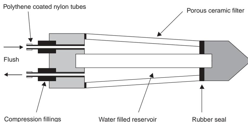
**Figure 10** Twin-tub piezometer
