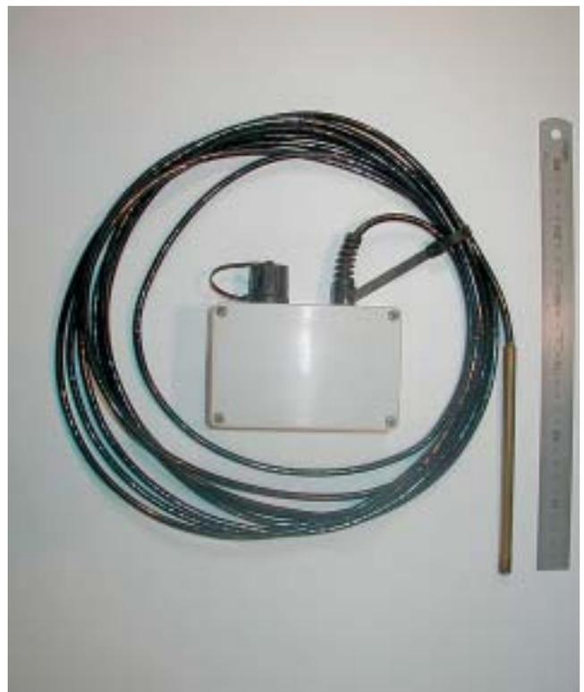
**Figure 30** Water level recorder
