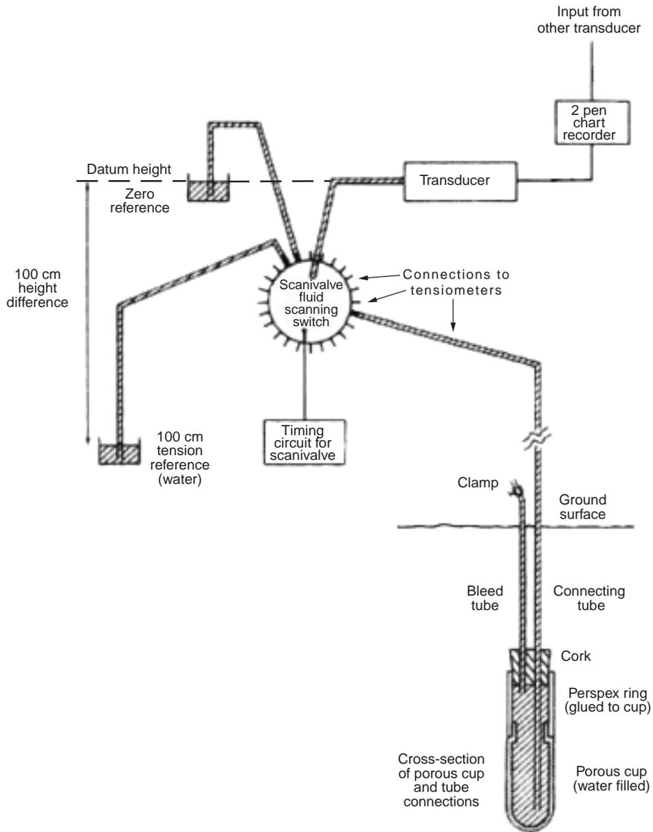
**Figure 11** Scanivalve system for reading an array of hydraulic piezometers (after Anderson and Burt, 1977)
