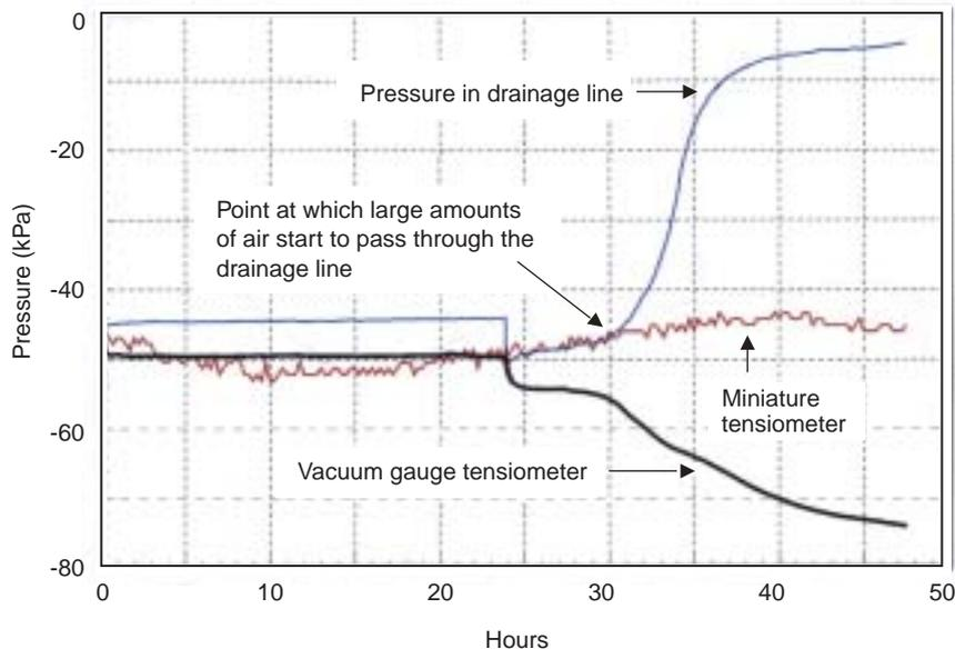
**Figure 24** Comparison of pressures measured by a vacuum gauge tensiometer and miniature tensiometer
