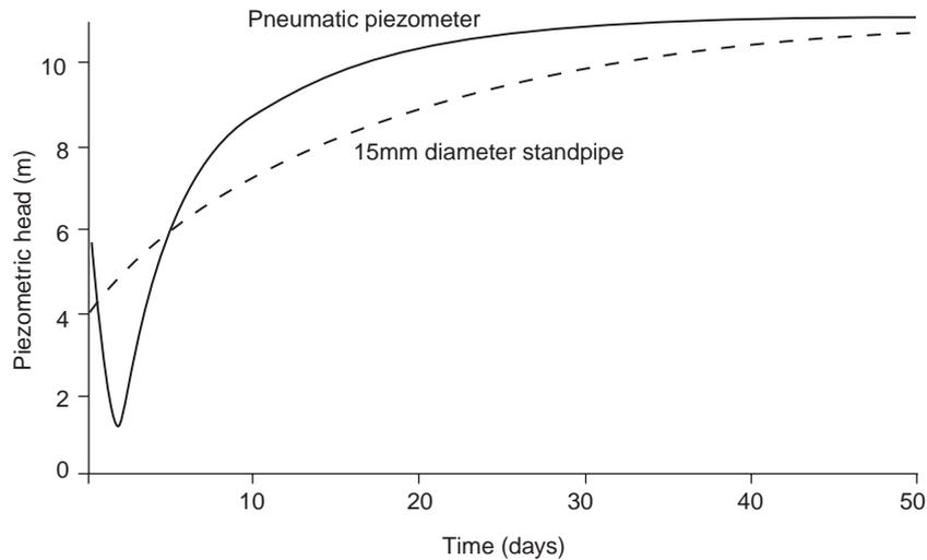
**Figure A4** Equalisation of piezometers with different hydraulic response times (after Vaughan, 1973)
