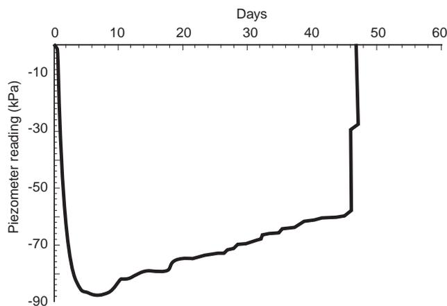
**Figure A6** The response of a piezometer to a pore water suction in excess of the air-entry value of the piezometer filter
