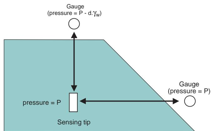
**Figure 12** Limitation on measurement range due to difference in elevation
