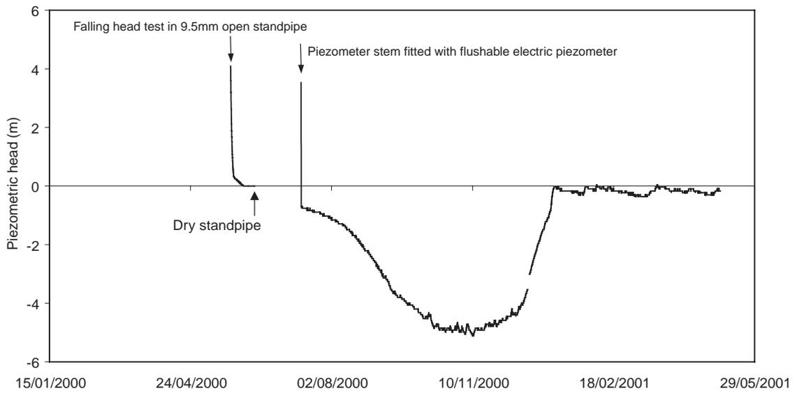
**Figure 33** Monitoring using a Type II piezometer stem
