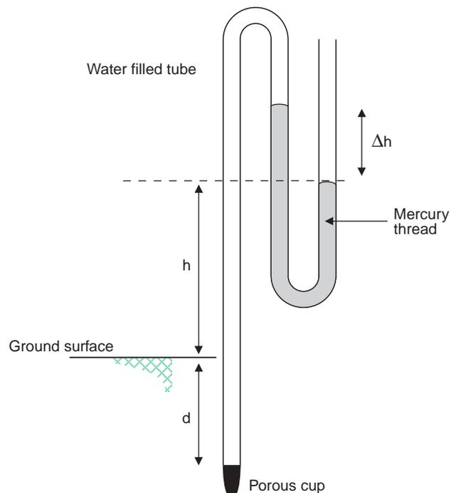
**Figure 16** Arrangement of a manometer tensiometer
