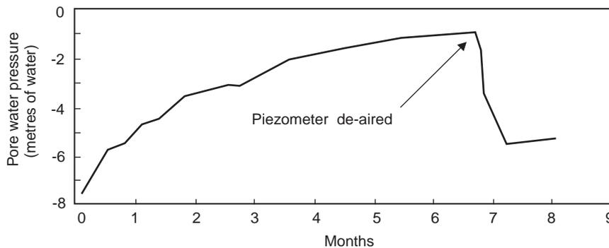
**Figure A8** Pore pressure measured in a mudstone fill by a hydraulic piezometer with a high air-entry filter (after Bishop *et al.*, 1964)
