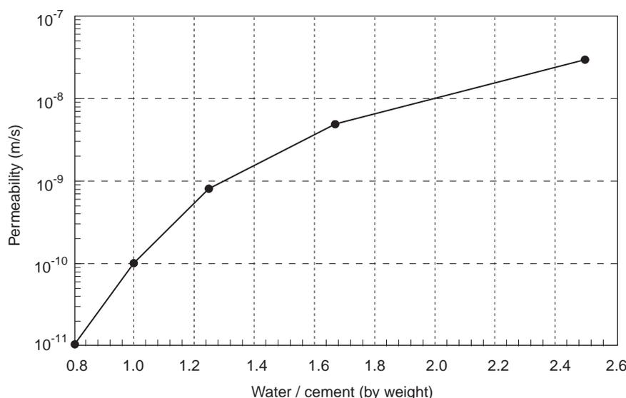
Figure A1 Permeability of cement grouts (data from Littlejohn, 1982)
