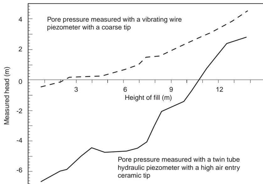
**Figure A10** Measurements of pore pressures during the placement of compacted fill (after Penman, 1978)
