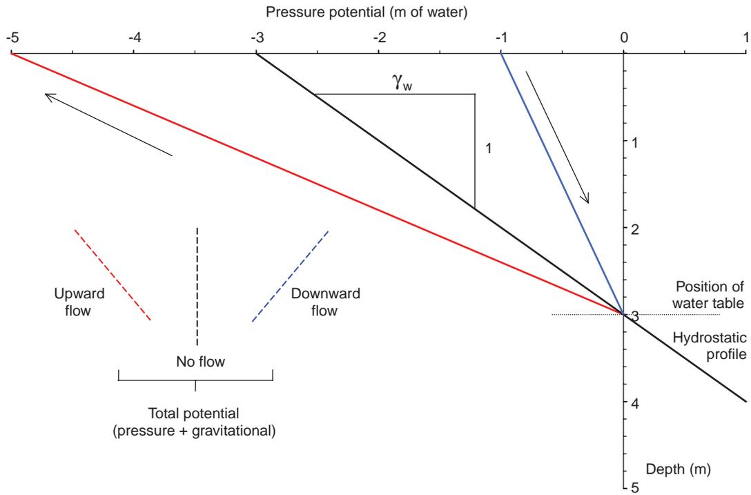
**Figure 1** Pore water pressure profiles in terms of pressure and total potential
