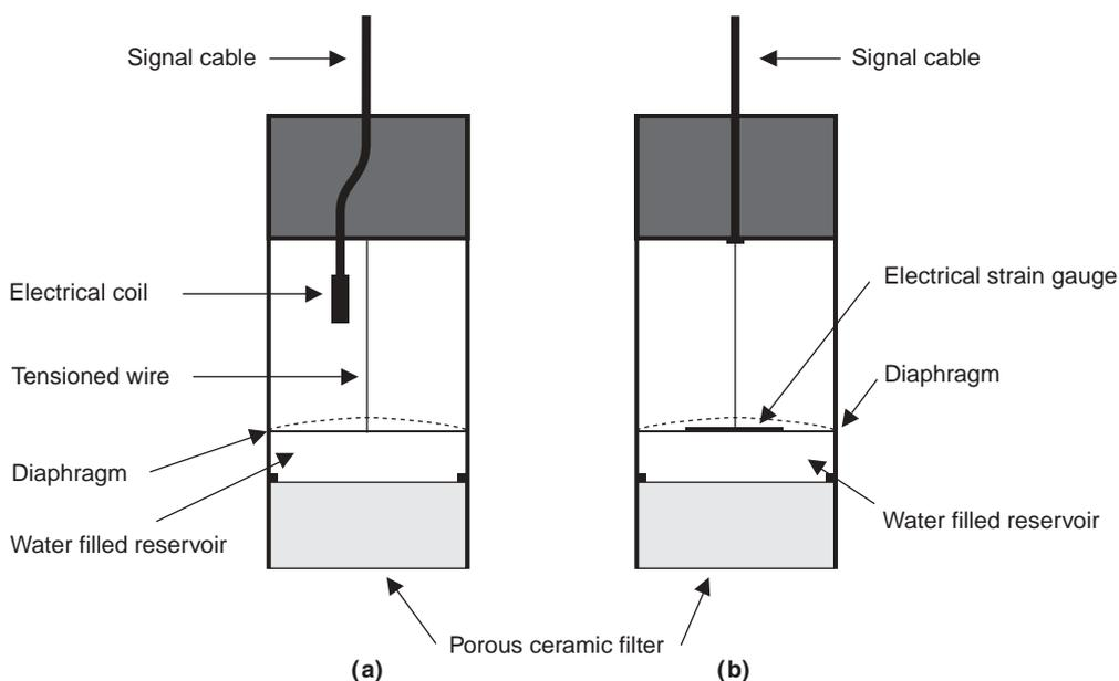
**Figure 14** Vibrating wire and electrical resistance piezometers
