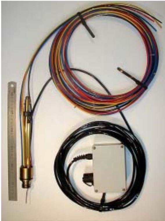
**Figure 31** Flushable electric piezometer
