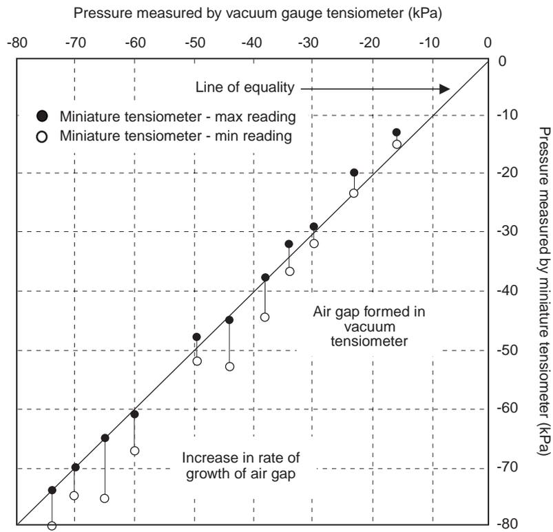
**Figure 23** Data from vacuum gauge tensiometer and miniature tensiometer
