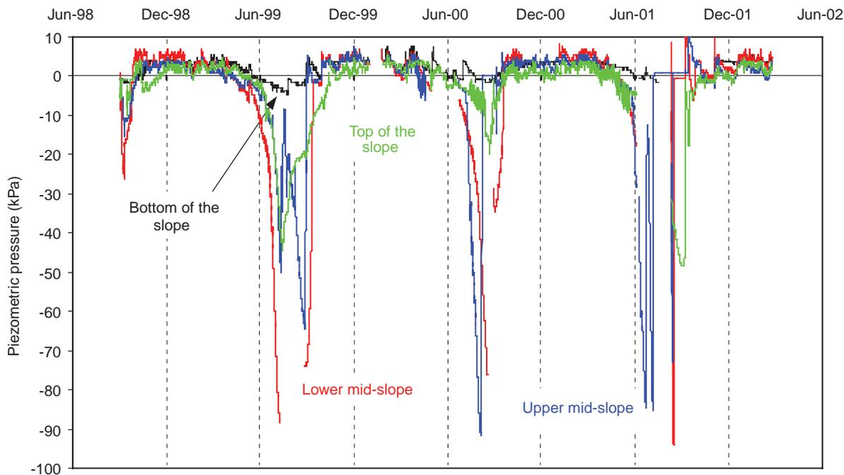
**Figure 35** Suction measurements using a Type I piezometer stem
