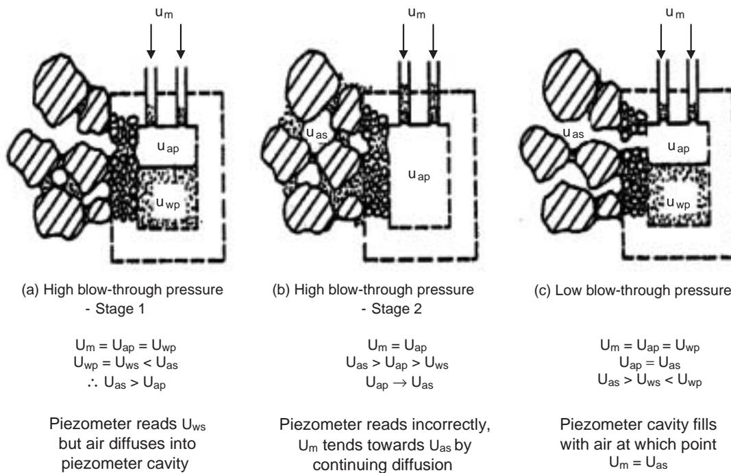
**Figure A7** Entry of air into a piezometer cavity
