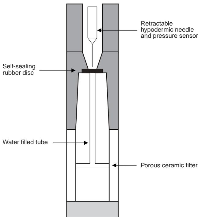
**Figure 15** Essential features of the BAT piezometer (after Torstensson, 1984)
