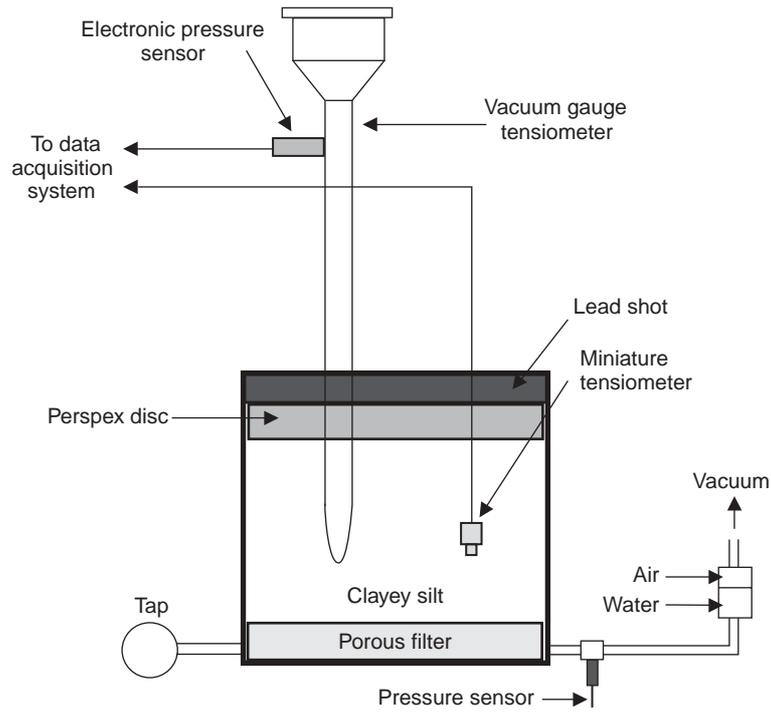
**Figure 22** Arrangement for comparing the readings from a vacuum gauge tensiometer and a miniature tensiometer
