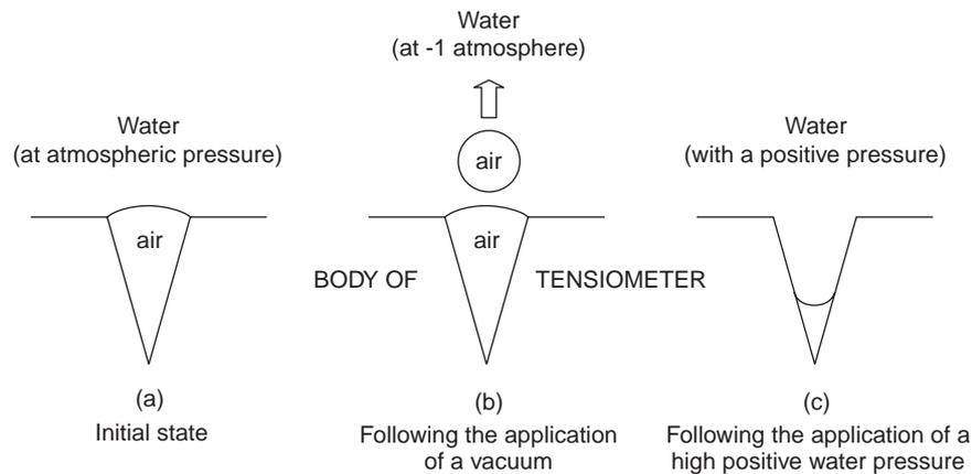
**Figure 20** The crevice model for explaining 'cavitation'
