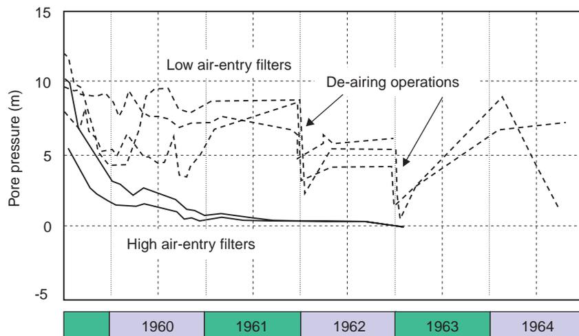
**Figure A9** Pore pressures measured by hydraulic piezometers at Selsset Dam (after Bishop *et al.*, 1964)
