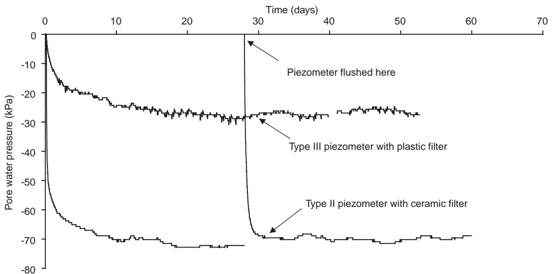
**Figure 34** Suction measurement using flushable electric piezometers
