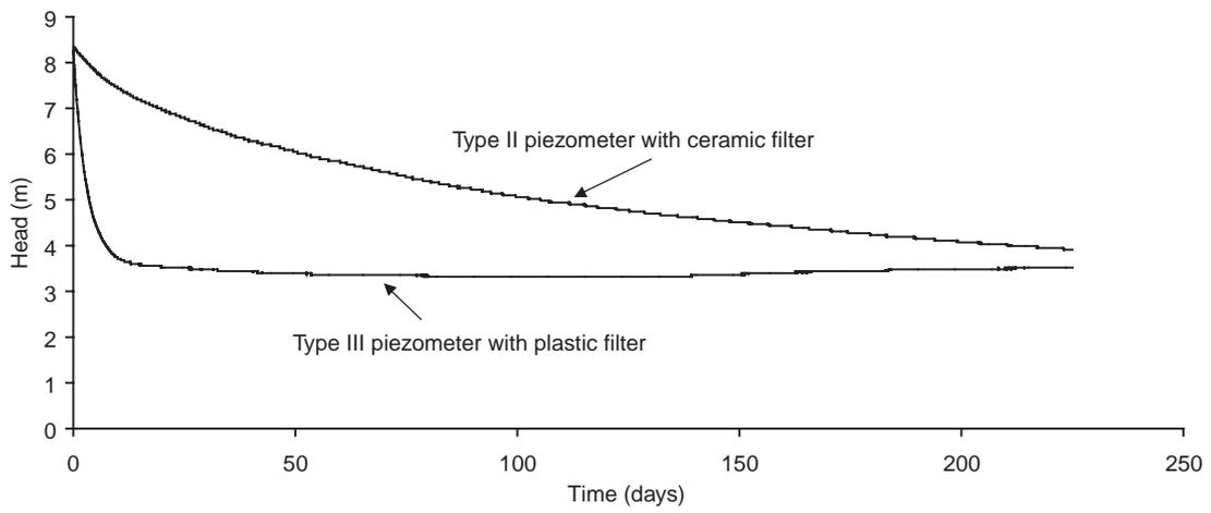
**Figure 32** Falling head tests
