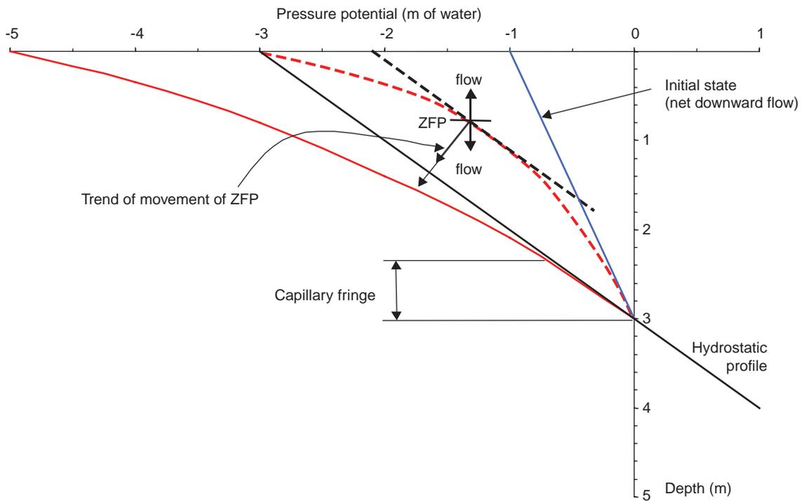
**Figure 2** Pore water pressure profile generated by evaporation from a horizontal surface
