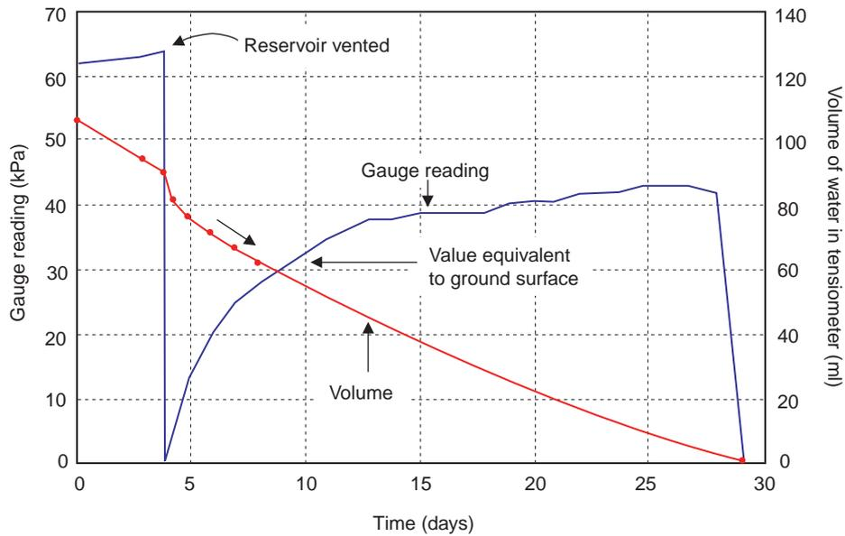
**Figure 25** Response of a vacuum gauge tensiometer in a high suction environment
