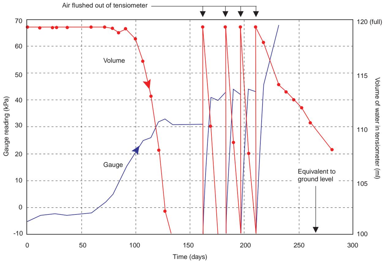
**Figure 21** Field measurements using a vacuum gauge tensiometer
