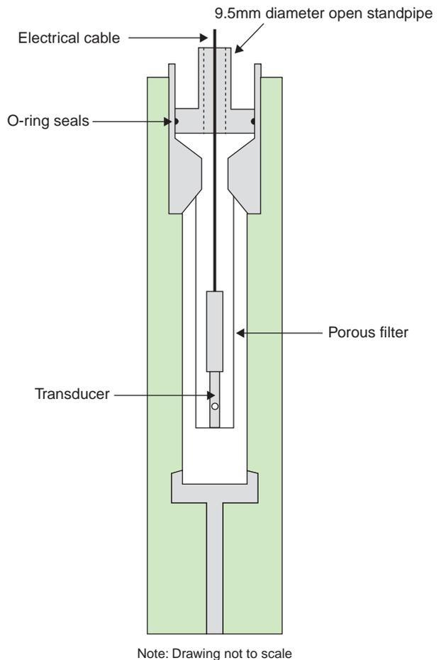
**Figure 29** Piezometer stem with open standpipe and water level recorder
