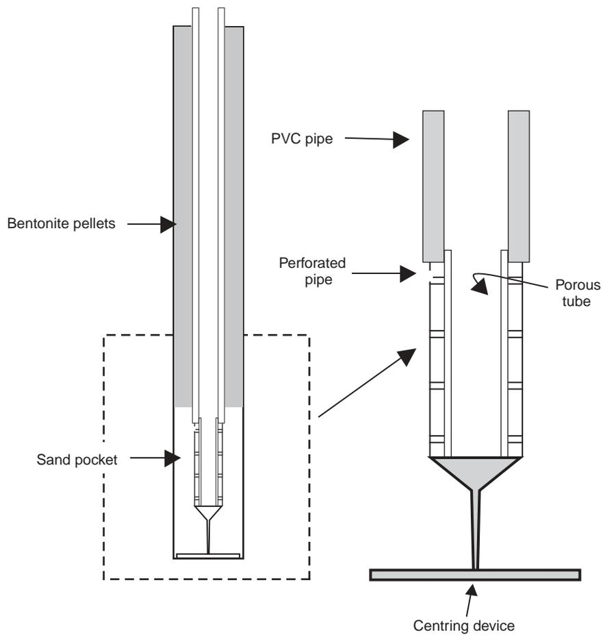
**Figure 9** Open standpipe piezometer
