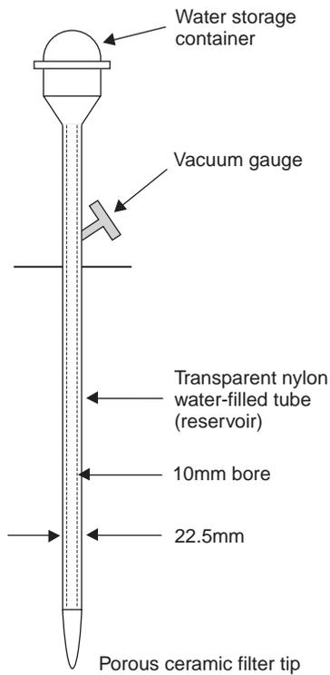
**Figure 18** Arrangement of a gauge tensiometer with 'jet-fill' reservoir
