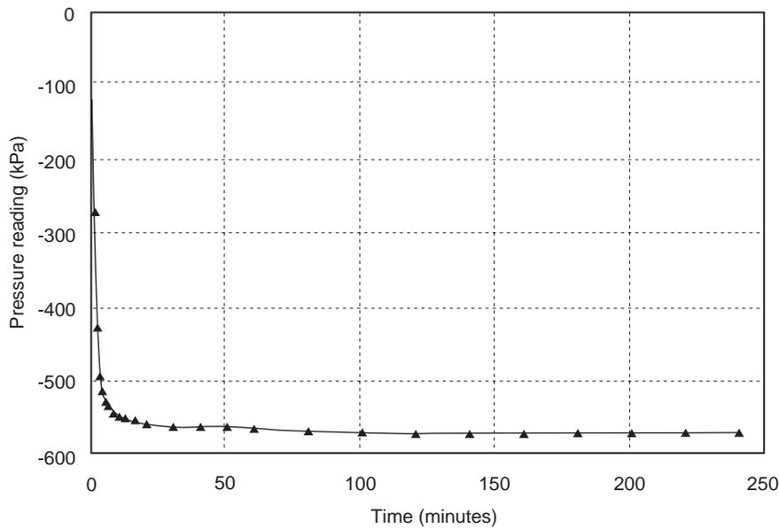
**Figure 26** Response of a miniature tensiometer in a compacted clay fill
