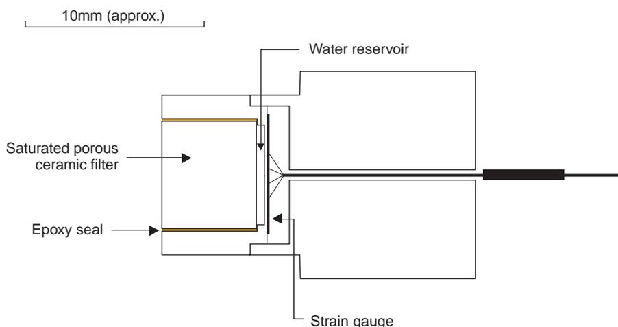
**Figure 19** The Imperial College miniature tensiometer (the 'suction probe')
