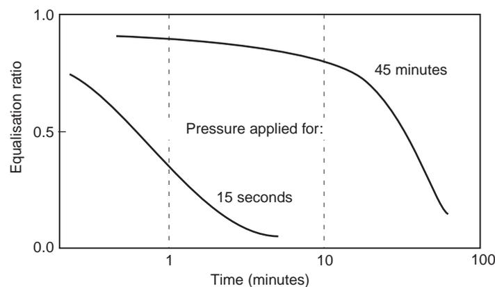
**Figure A5** Equalisation of a piezometer (with the intake factor,  $F = 13\text{cm}$ ) following application of a constant out-of-balance pressure (after Vaughan, 1973)
