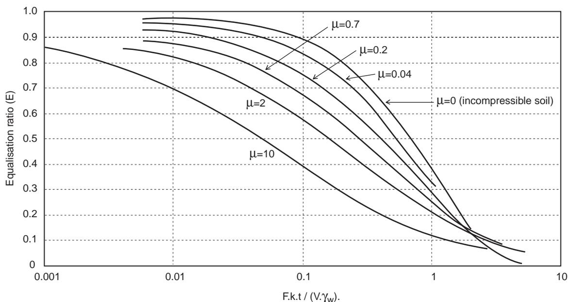
**Figure A2** The hydraulic response of a piezometer (after Hvorslev, 1951 and Gibson, 1963)
