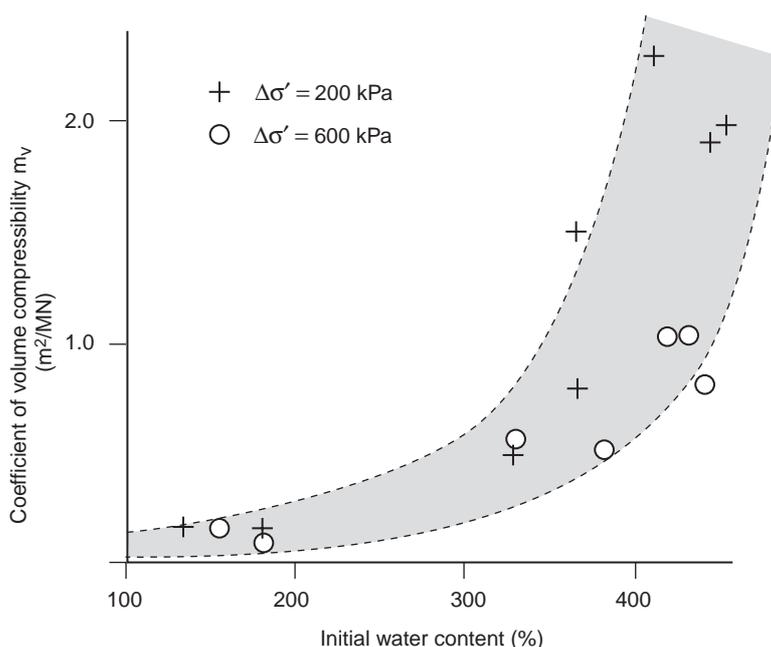
**Figure A3** Stiffness of cement-bentonite grouts measured in one-dimensional compression
