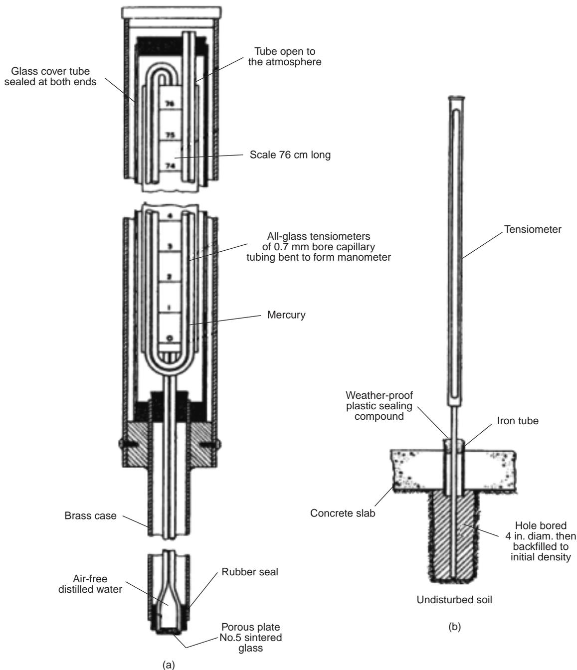
**Figure 17** Arrangement of a mercury manometer tensiometer (after Black *et al.*, 1958)
