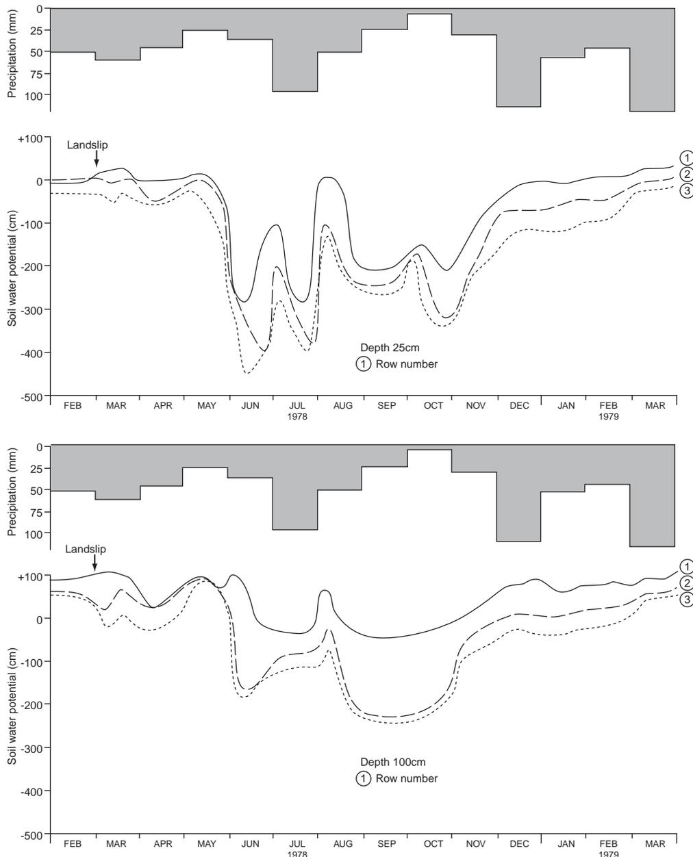
**Figure 7** Relation between pore water pressures and precipitation for a site on the M4 near Swindon (after Anderson and Kneale, 1980)
