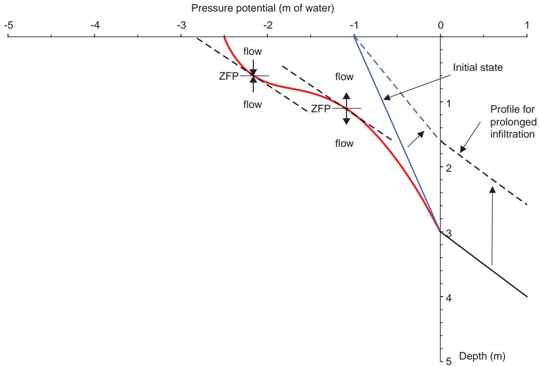
**Figure 3** Pore water pressure profile generated by infiltration into a horizontal surface
