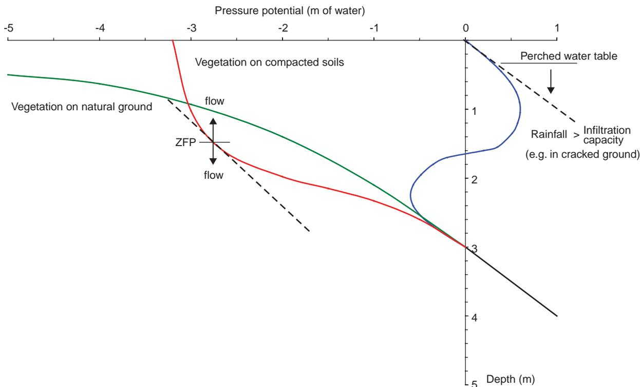
**Figure 5** Pore water pressure profiles generated by vegetation and surface cracking
