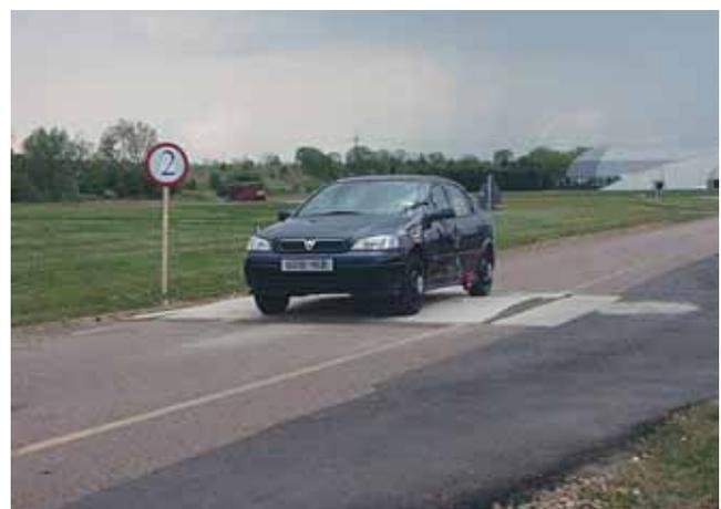
**Figure 8 Sinusoidal hump**
