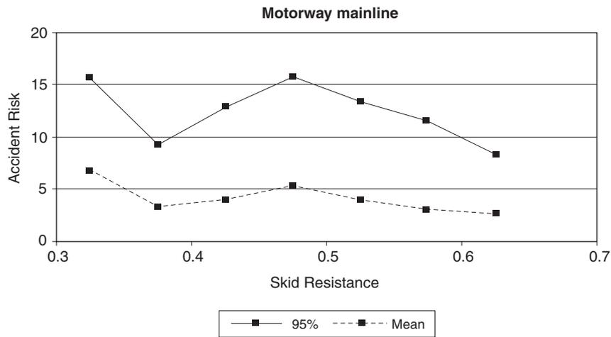
Figure 4 Mean and 95<sup>th</sup> percentile all-accident risk for motorways
