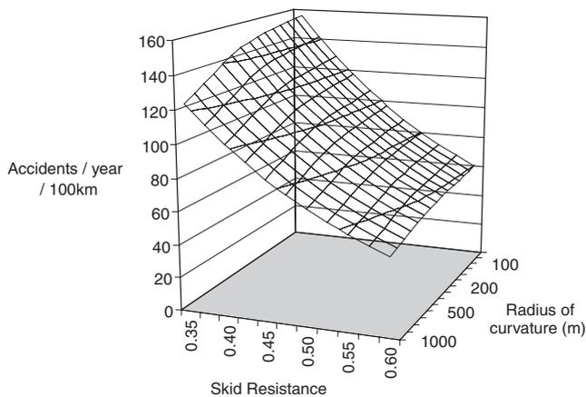
**Figure 12** Mean predicted all-accident rate by skid resistance and radius of curvature for single carriageways with moderate traffic flow
