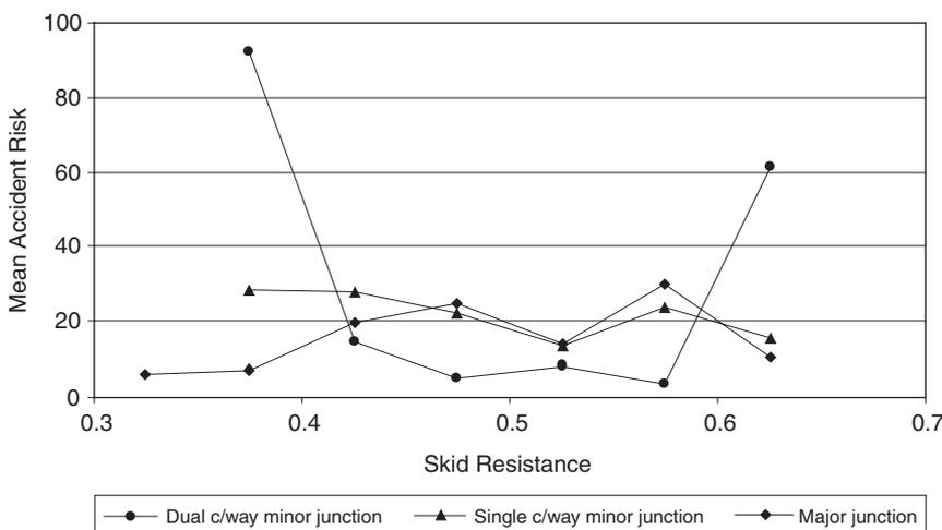
Figure 9 Mean all-accident risk by skid resistance for junctions
