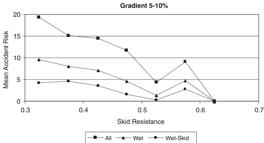
**Figure 13** Mean accident risk by skid resistance for gradients 5-10%
