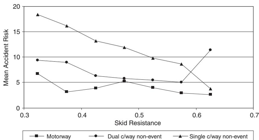
Figure 1 Mean all-accident risk by skid resistance for non-event lengths
