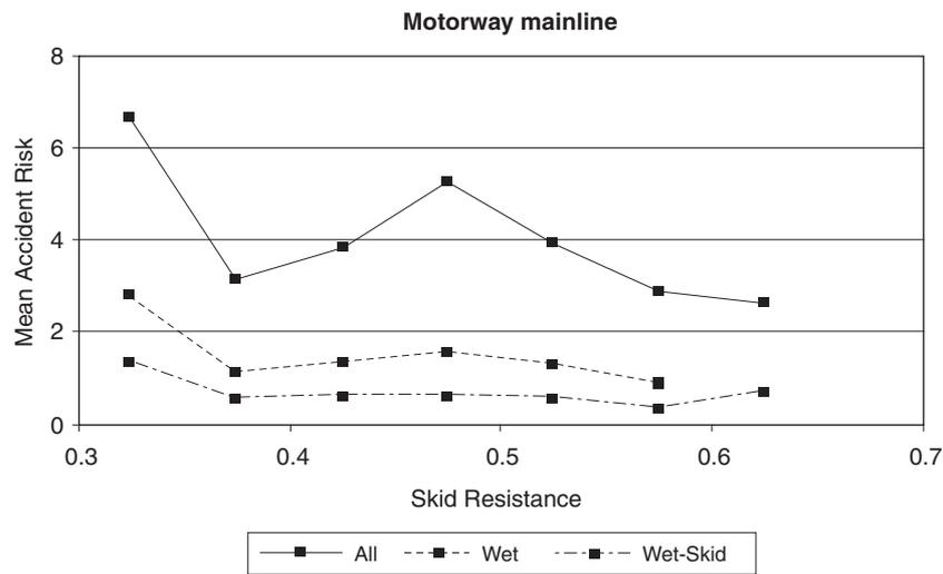
Figure 2 Mean accident risk by skid resistance for motorways
