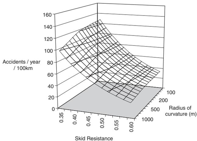
**Figure 11** Mean predicted all-accident rate by skid resistance and radius of curvature for dual carriageways with moderate traffic flow
