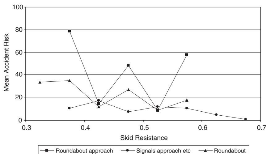
Figure 10 Mean all-accident risk by skid resistance for approaches and roundabouts
