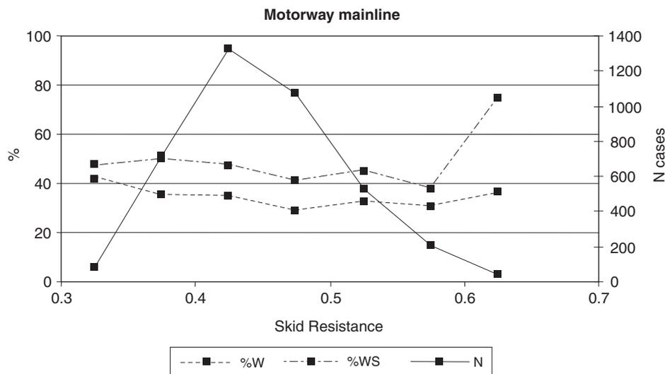
Figure 3 Accident ratios and numbers by skid resistance for motorways
