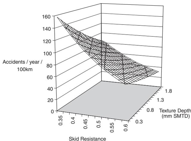
**Figure 14** Mean predicted all-accident rate by skid resistance and texture depth for single carriageways
