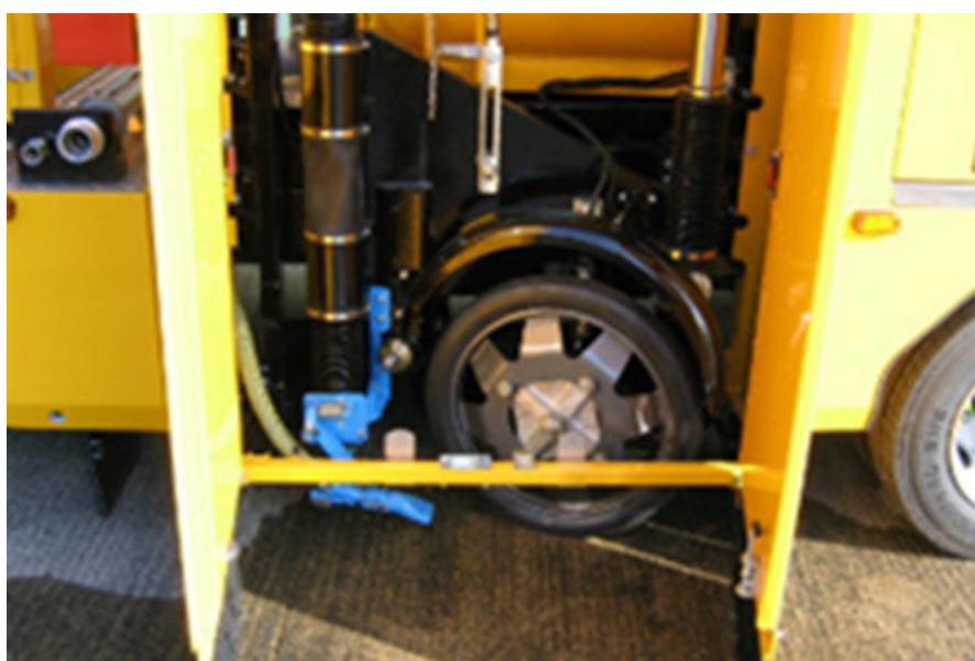
Figure 2-2: Test wheel within the SCRIM survey vehicle
