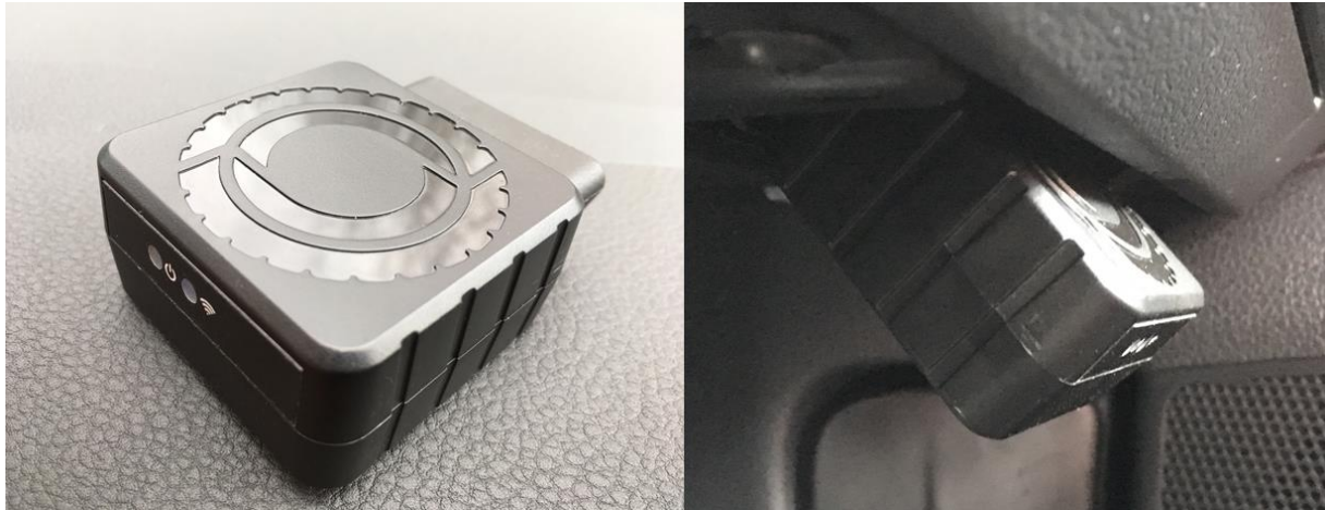
Figure 12: FleetCarma 'C2' telematics dongle (left) and in situ in vehicle (right)
