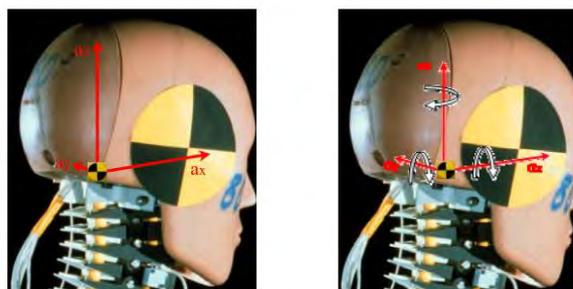
Fig. 2. Translational acceleration. Note Fig. 3. Rotational acceleration. that there was no neck in the tests.
