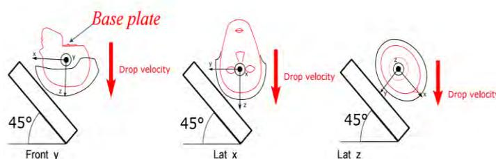
Figure 1 : Illustration of the tangential helmet test impact conditions.
