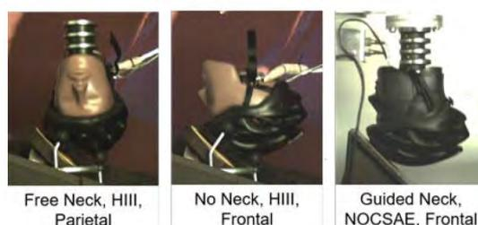
Figure 1: Example configurations demonstrating the two headforms, three neck conditions, and two locations.
