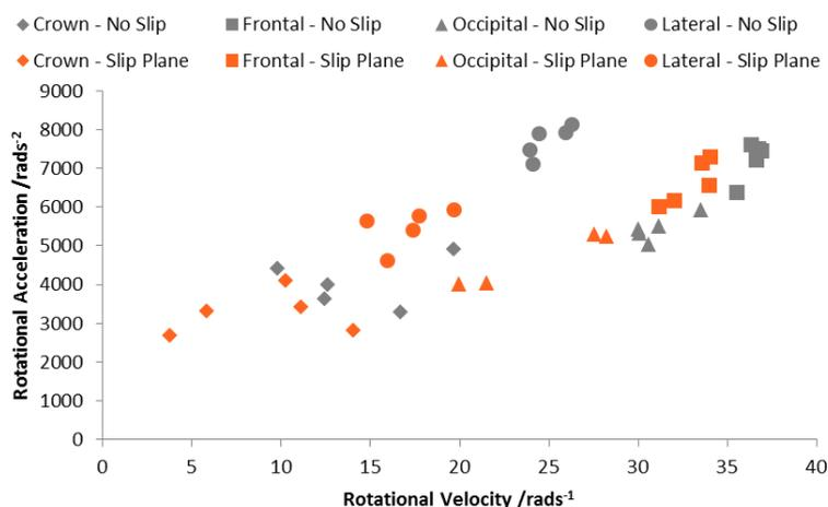
Figure 2: Comparison of rotational velocity and rotational accelerations for each impact location and each slip plane case
