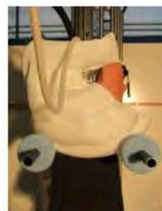
Fig. 7. The Hövding 2.0 and the larger anvil.
