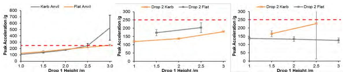
Figure 2: Mean peak linear headform accelerations for (a) the first impact (Drop 1) against both the flat and kerbstone anvils and the compound impact (Drop 2) against both the flat and kerbstone anvils when compared to the drop height of the first impact (Drop 1) against the (b) flat and (c) kerbstone anvils
