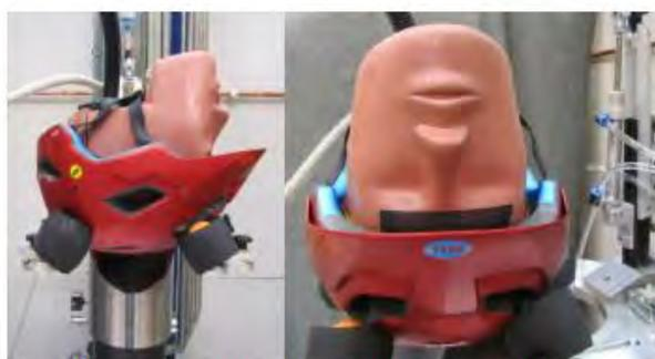
Fig. 4. The oblique test A with rotation around X-axis.
