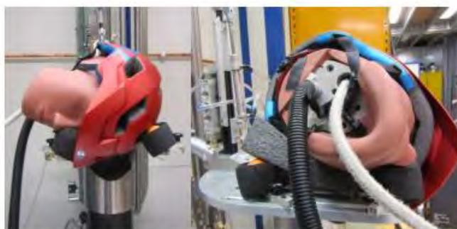
Fig. 6. The oblique test C with rotation around Z-axis (pre-positioned 20° in X and 35° in Z).
