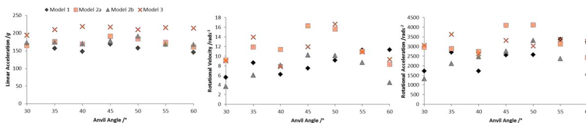
Figure 3: Peak (a) linear accelerations, (b) rotational velocities and (c) rotational accelerations experienced by four different helmet models when impacted against a range of different anvil angles
