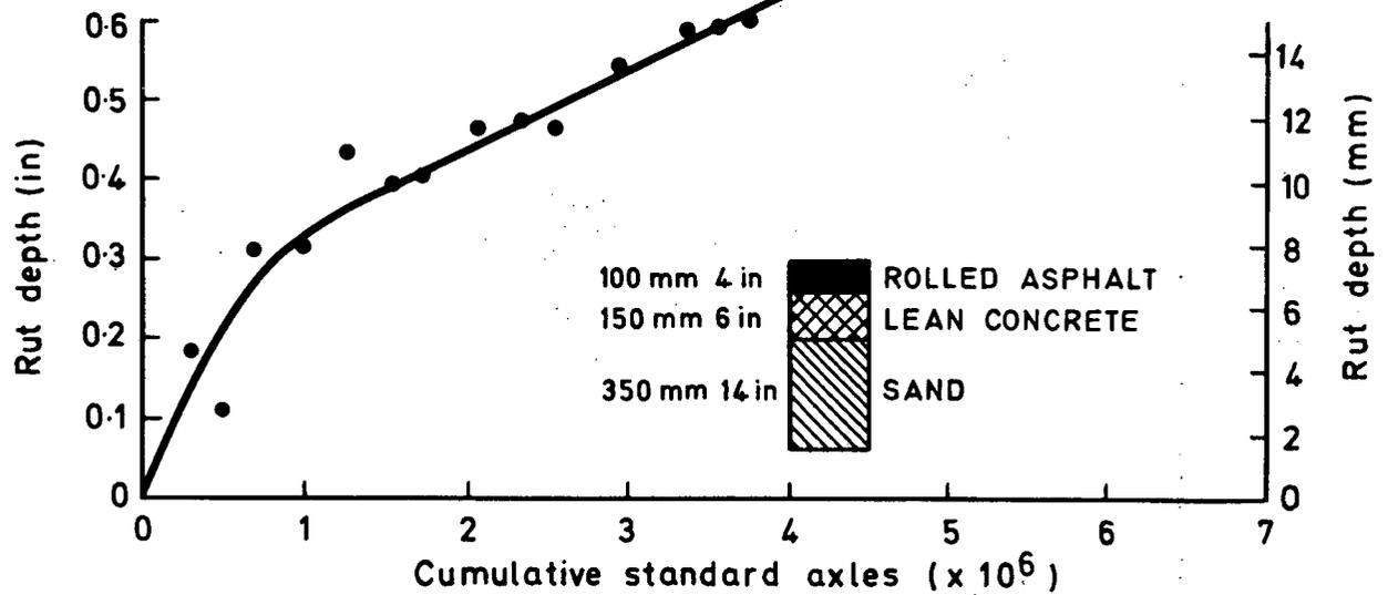
Fig.8. TYPICAL RELATIONS BETWEEN RUT DEPTH AND CUMULATIVE TOTAL OF STANDARD AXLES
