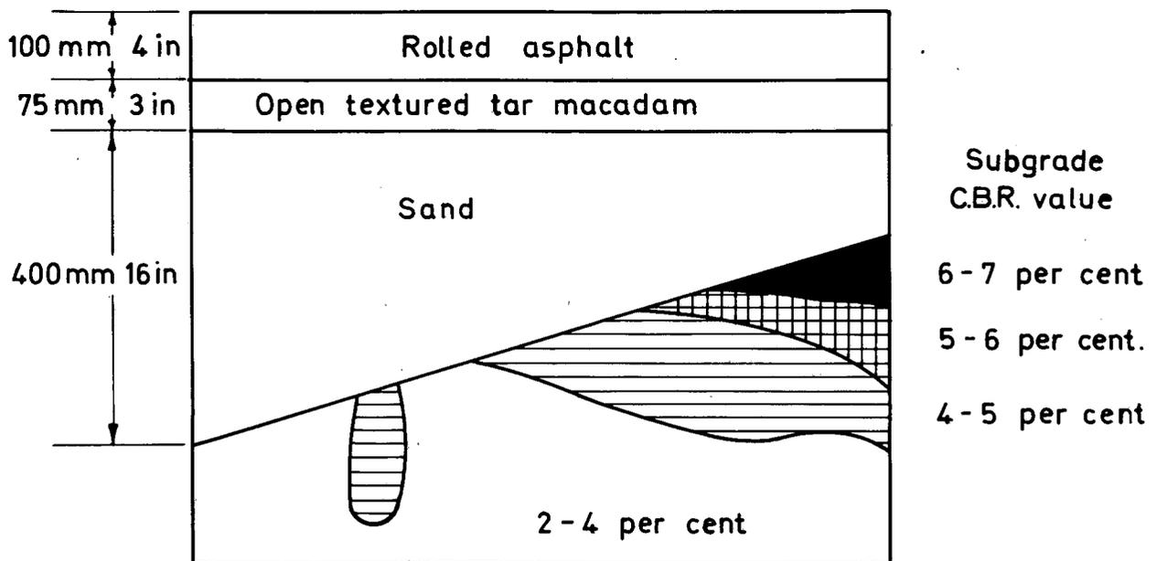
Fig.11. VARIATION OF SUB - GRADE STRENGTH UNDER SECTION 41.
