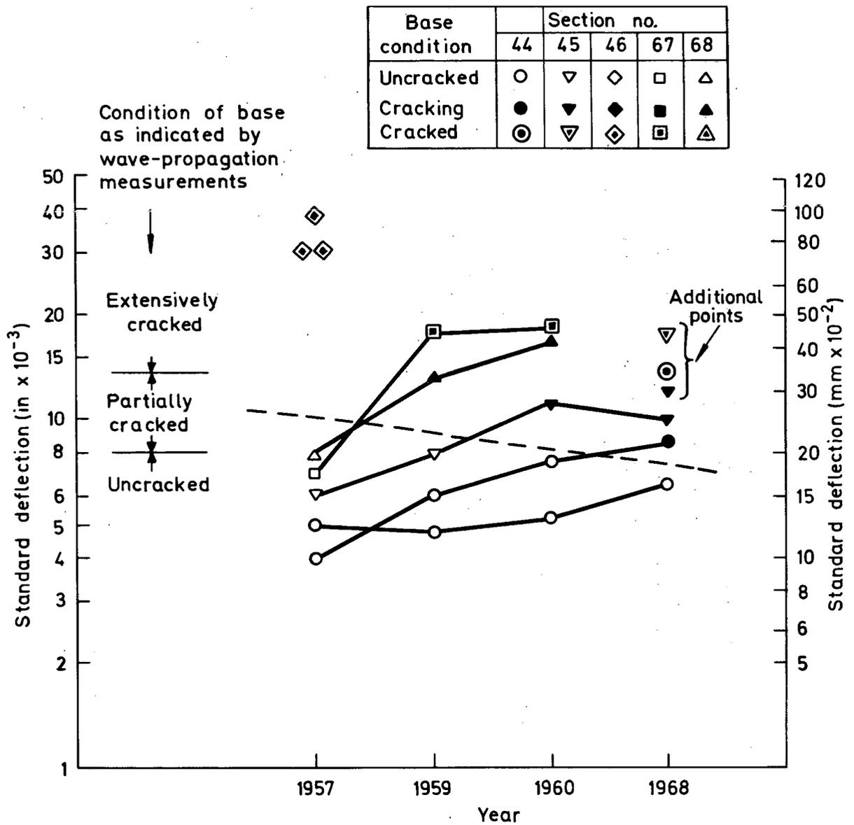
Fig.25. RELATION BETWEEN DEFLECTION AND THE CONDITION OF THE LEAN CONCRETE BASES
