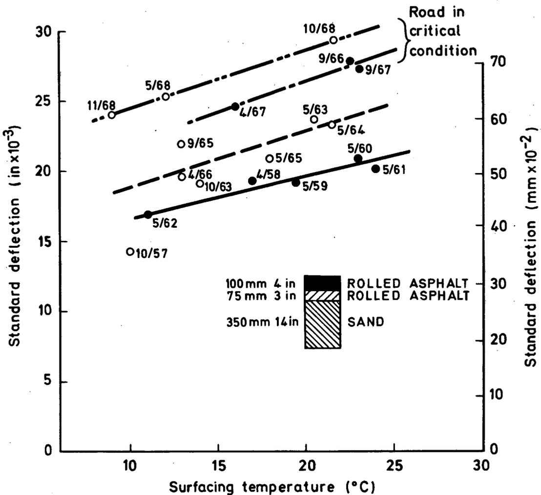
Fig. 7. TEMPERATURE SUSCEPTIBILITY FOR SECTION WITH DETERIORATING STRUCTURAL STIFFNESS
