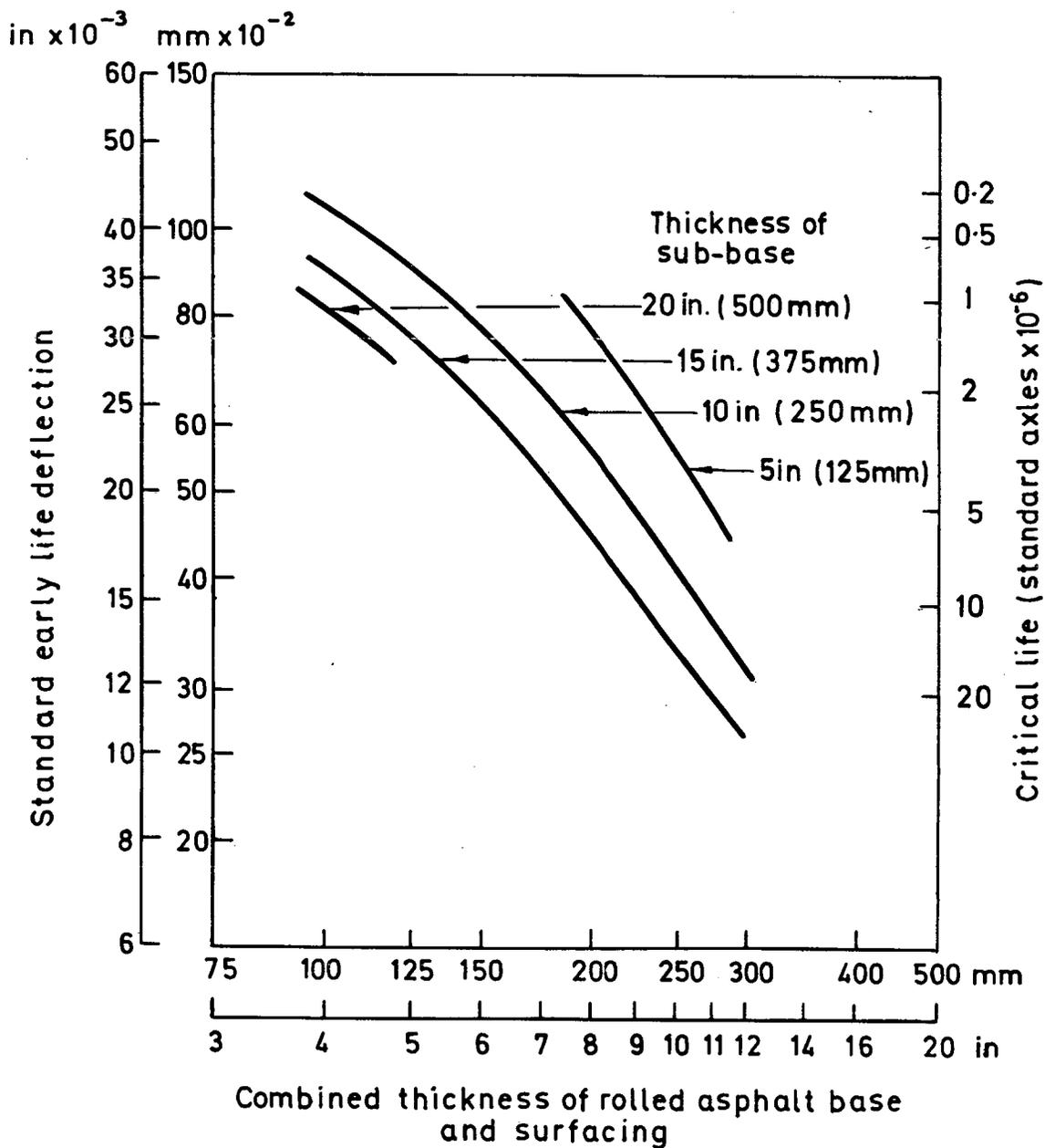
Fig.31 RELATION BETWEEN DEFLECTION, CRITICAL LIFE AND THICKNESS FOR PAVEMENTS WITH ROLLED ASPHALT BASES AT ALCONBURY HILL
