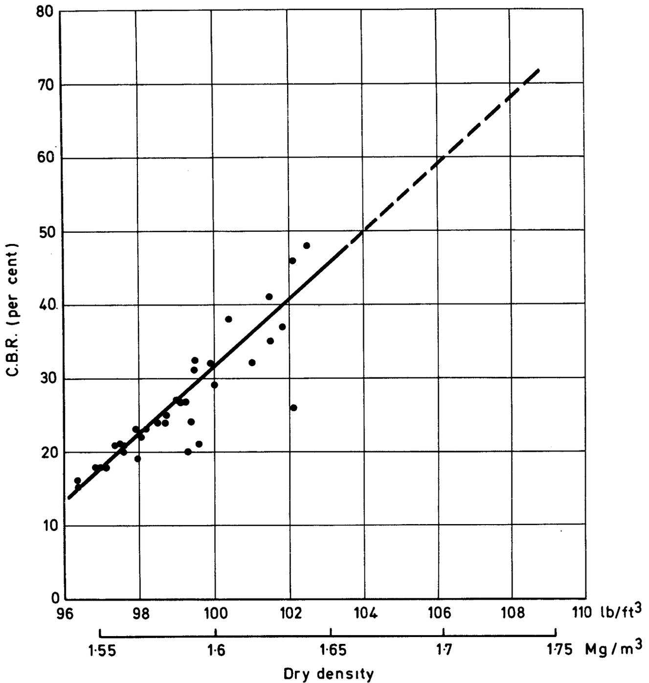
Fig. 12. RELATION BETWEEN IN-SITU C.B.R. AND DRY DENSITY OF THE SAND SUB-BASE AT ALCONBURY HILL
