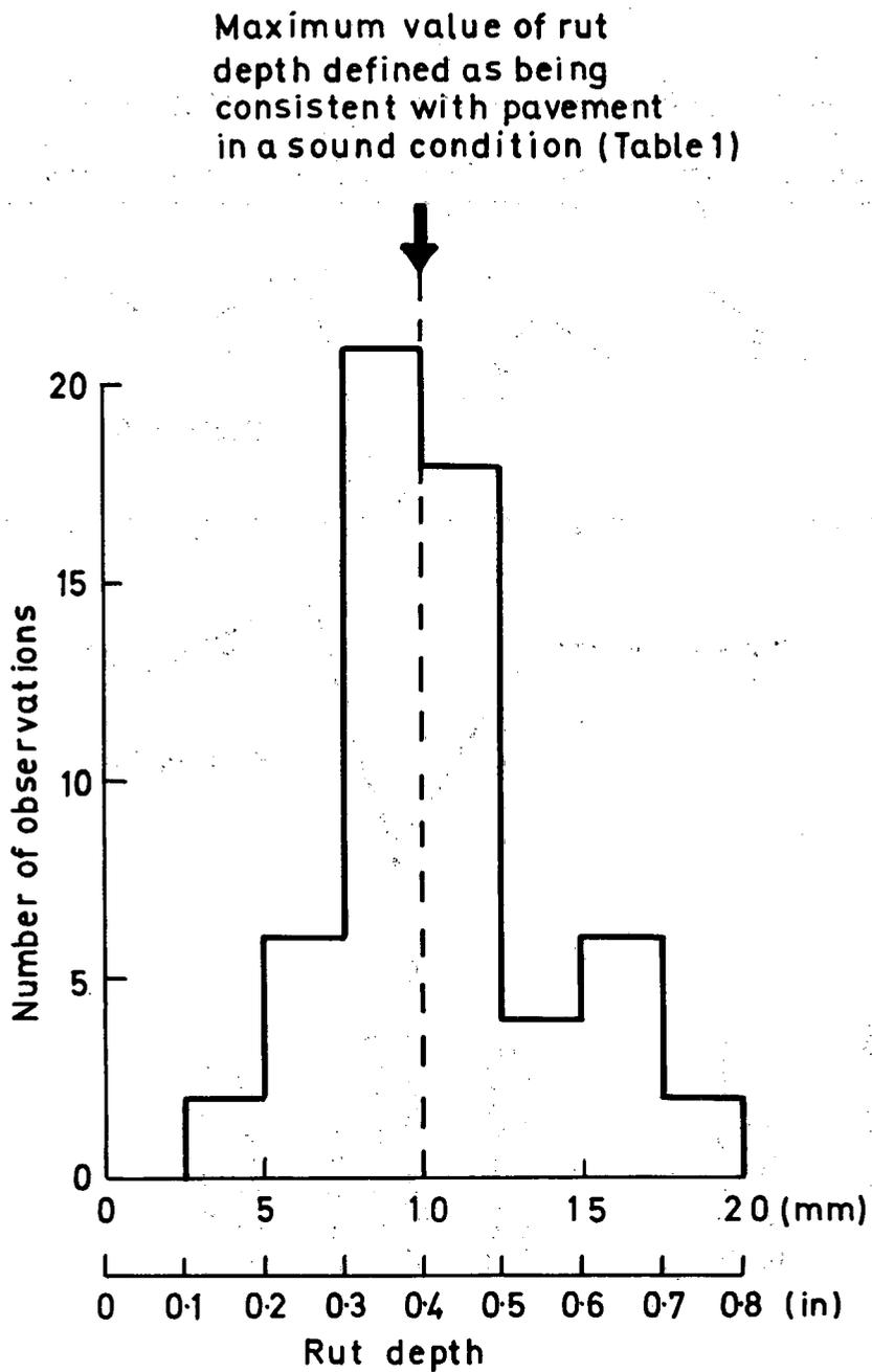
**Fig.9. DISTRIBUTION OF RUT DEPTHS IN THE NEAR SIDE WHEELPATH AT WHICH SIGNIFICANT CRACKING OF THE SURFACING COMMENCED**
