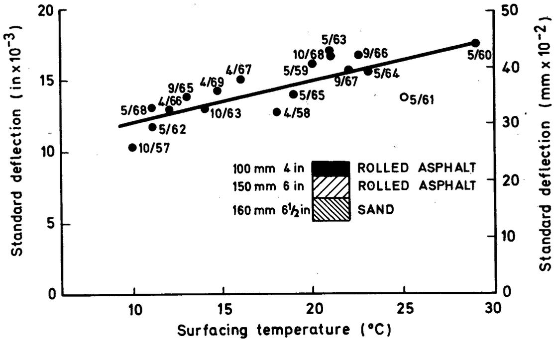
Fig.6 TEMPERATURE SUSCEPTIBILITY FOR SECTION OF VIRTUALLY CONSTANT STRUCTURAL STIFFNESS
