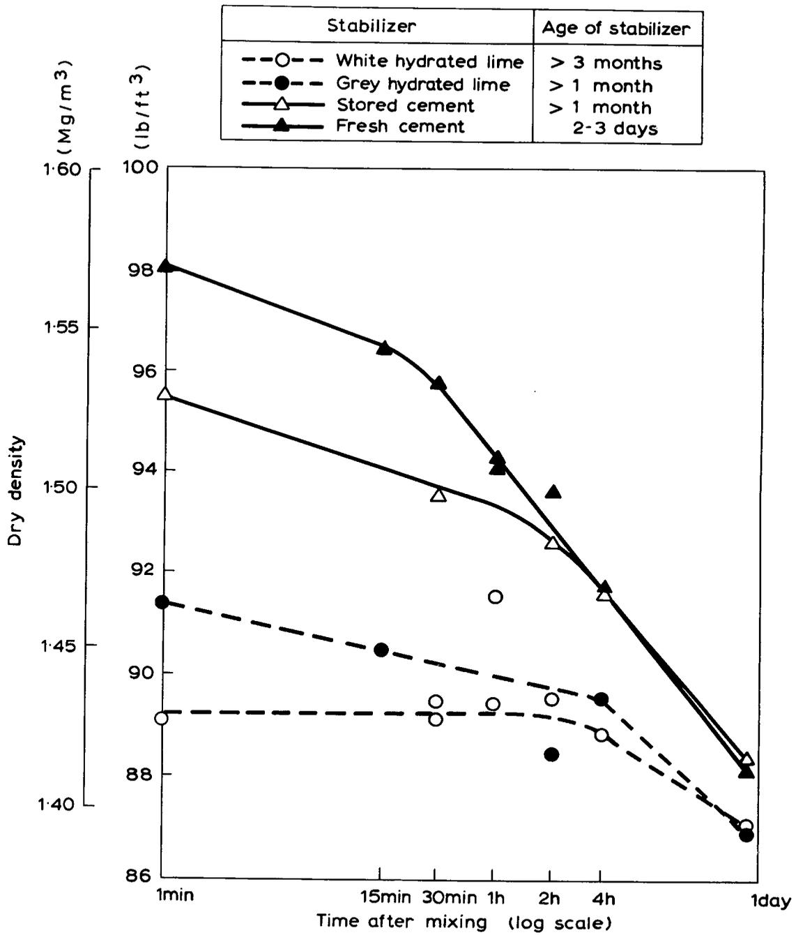
Fig.12. THE EFFECT OF A LAPSE OF TIME BETWEEN MIXING AND COMPACTION ON THE DRY DENSITY ATTAINED FOR SOIL FROM SCHEME No.8 WITH 5 PER CENT STABILIZER
