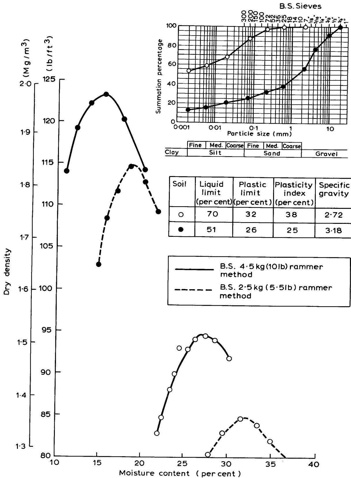
Fig. 8. CLASSIFICATION AND COMPACTION DATA FOR TYPICAL SOIL SAMPLES FROM SCHEME No. 7
