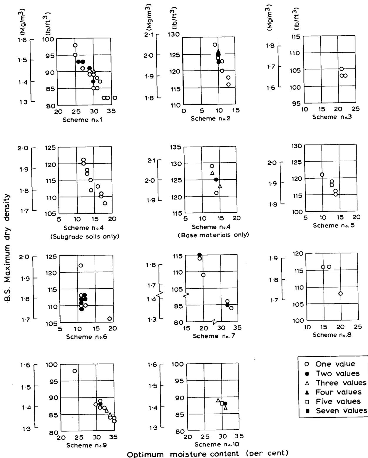
Fig.1. B.S. COMPACTION TEST DATA. (2.5 kg (5.5lb) RAMMER METHOD)
