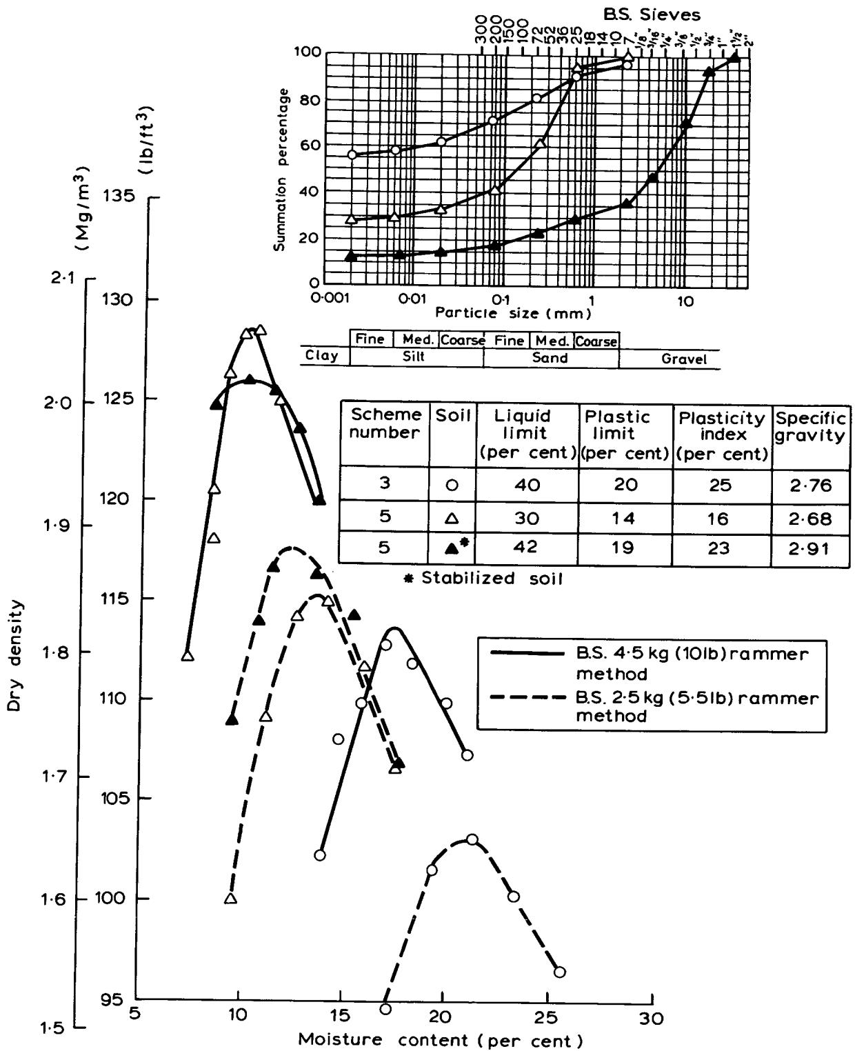
Fig. 4 CLASSIFICATION AND COMPACTION DATA FOR TYPICAL SOIL SAMPLES FROM SCHEMES Nos. 3 AND 5
