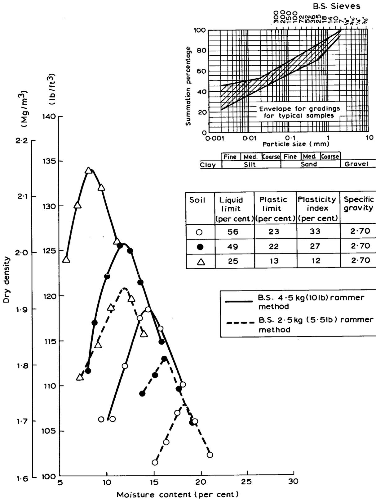
Fig. 5. CLASSIFICATION AND COMPACTION DATA FOR TYPICAL SUBGRADE SOIL SAMPLES FROM SCHEME No. 4
