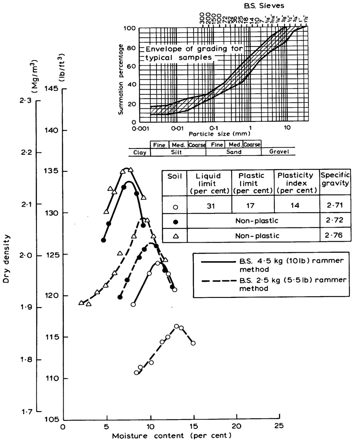
Fig. 3. CLASSIFICATION AND COMPACTION DATA FOR TYPICAL STABILIZED SOIL SAMPLES FROM SCHEME No. 2
