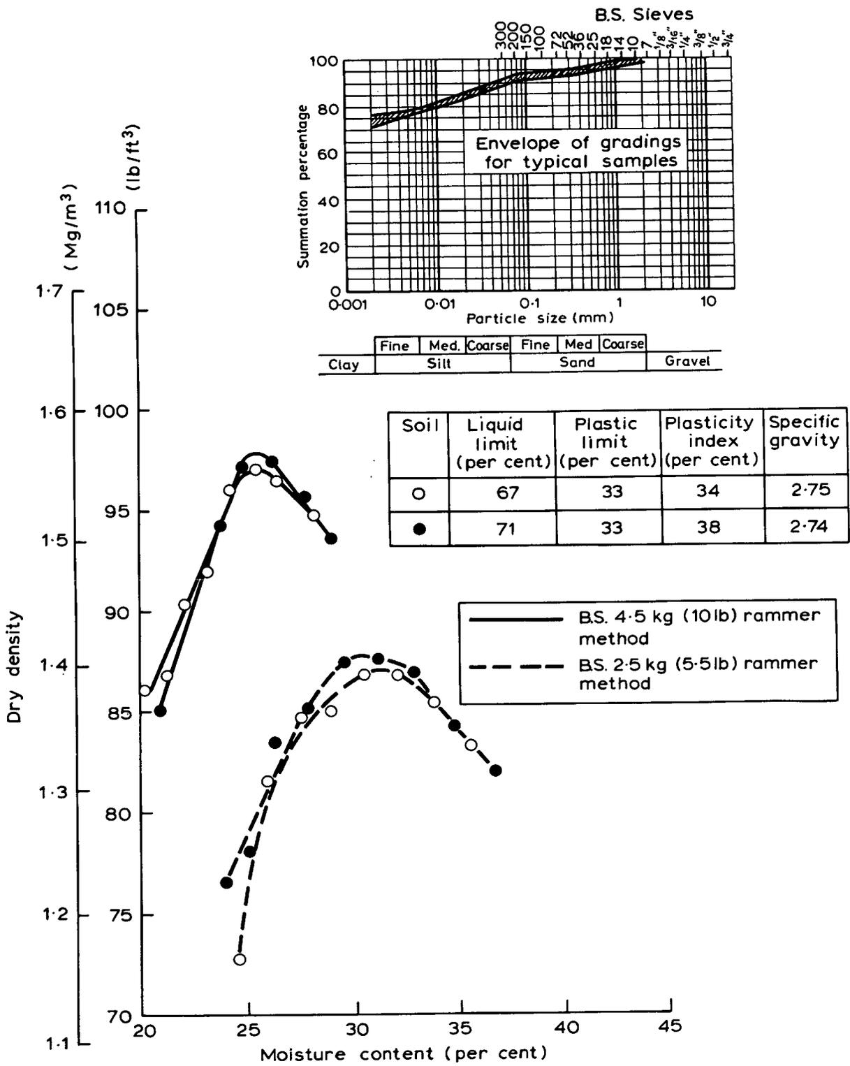
Fig. 11 CLASSIFICATION AND COMPACTION DATA FOR TYPICAL SOIL SAMPLES FROM SCHEME No. 10
