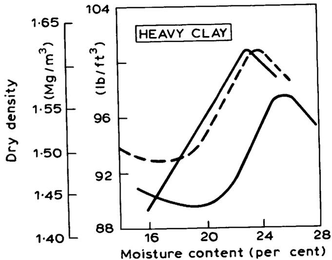
Fig. 22. TWO DRY DENSITY/MOISTURE CONTENT RELATIONS FOR A 12 Mg (12 tons) PNEUMATIC-TYRED ROLLER COMPACTING 23cm (9in) LOOSE LAYERS OF HEAVY CLAY SOIL
