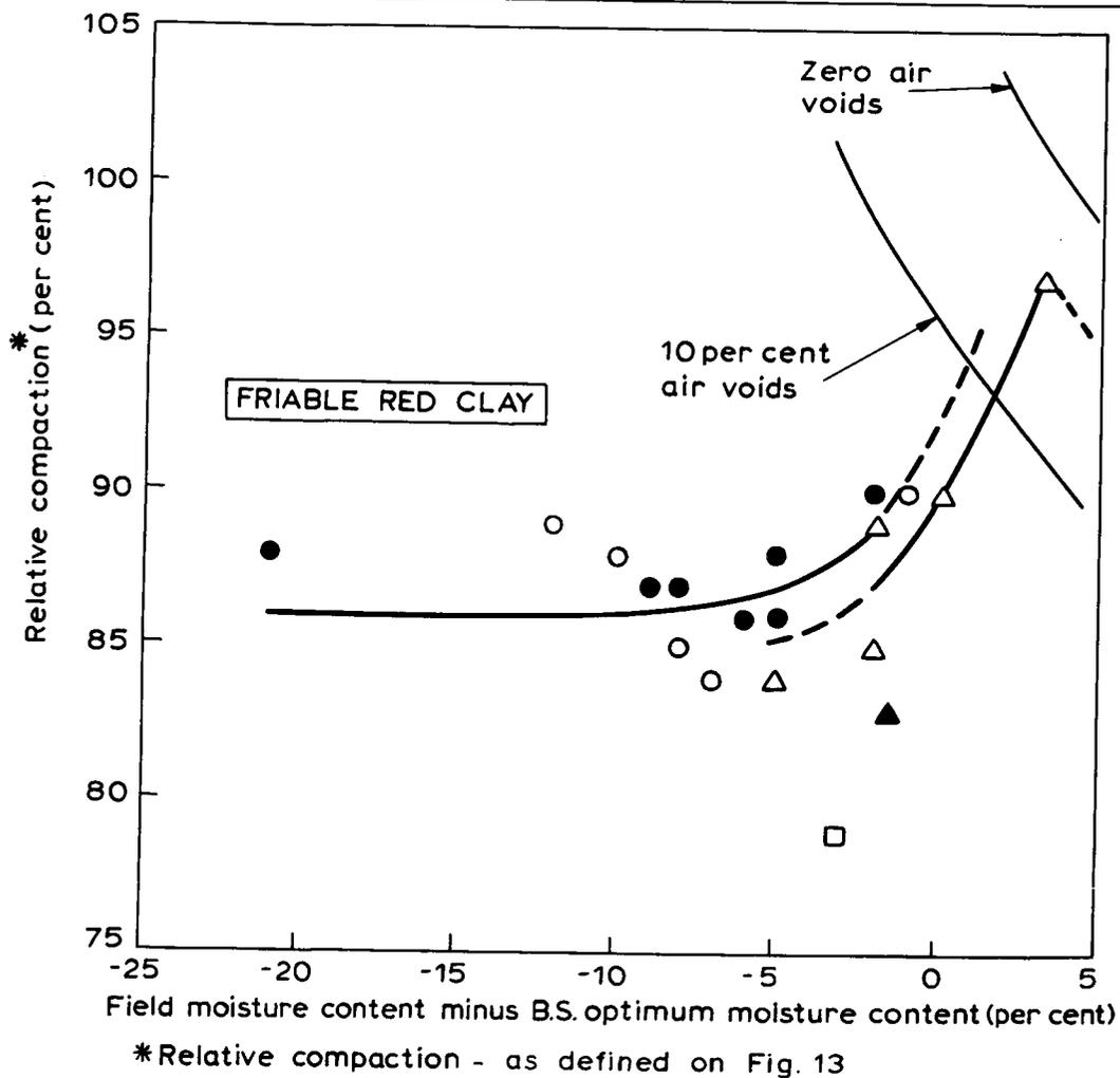
Fig. 14. RELATION BETWEEN RELATIVE COMPACTION AND MOISTURE CONDITIONS FOR THE TOP 15cm (6in) OF COMPACTED SOIL FOR 4 PASSES OF PNEUMATIC-TYRED WHEELS ON FRIABLE RED CLAY SOILS AT SCHEMES Nos 1,7, 9 AND 10
