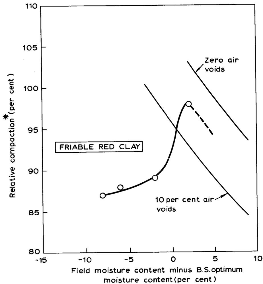
\*Relative compaction =  $\frac{\text{Field dry density} \times 100}{\text{Maximum dry density of B.S. compaction test 2.5kg (5.5lb) rammer method}}$  per cent
