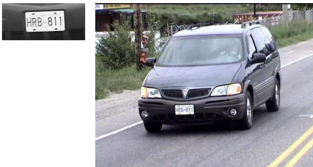
Figure 5: Plate patch (left) and overview (right) images from an ANPR camera
