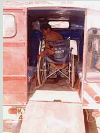
Figure 3.51 Side and rear view of a 3-wheeled motorcycle turned into a prototype accessible van (Courtesy of Wycliffe Kepha)
