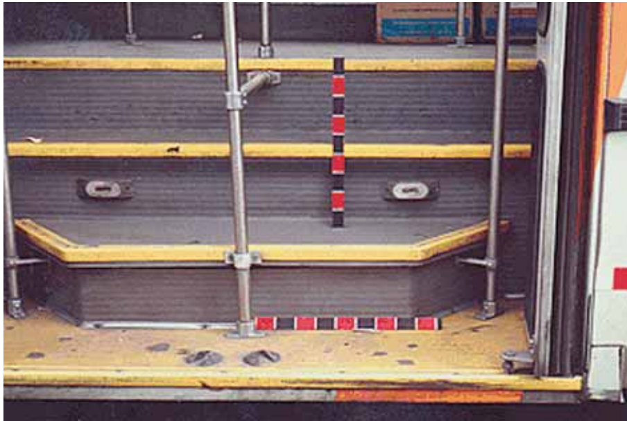
Figure 3.43 The rear entrance of newly deployed midibuses in Mexico City feature good colour contrast and wide doorways
