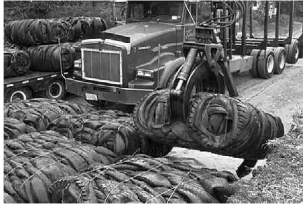
Figure 2. Use of a 'loggers-clam' to handle tyre bales.
