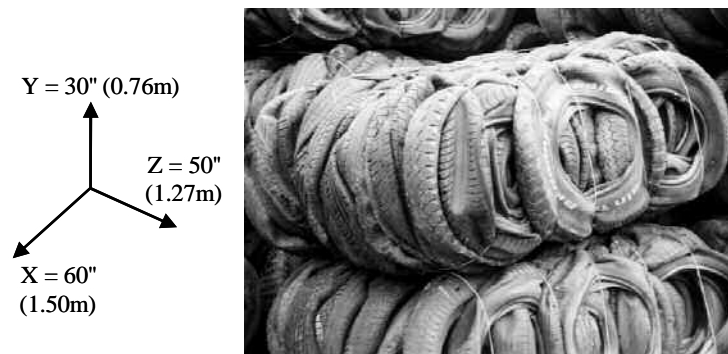
Figure 1. A typical tyre bale with dimensions.
