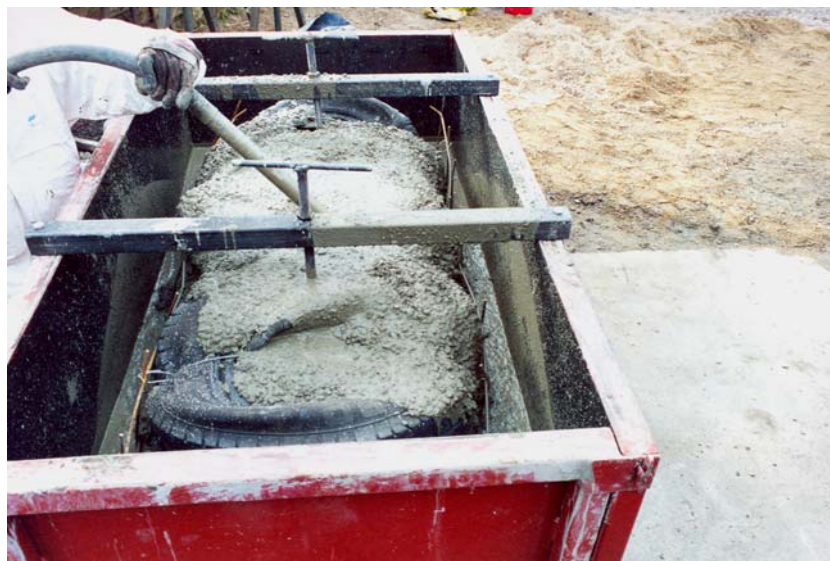
Figure 9.1 – Manufacture of the concrete blocks. (Photograph © Northern Tyre Recycling.)
