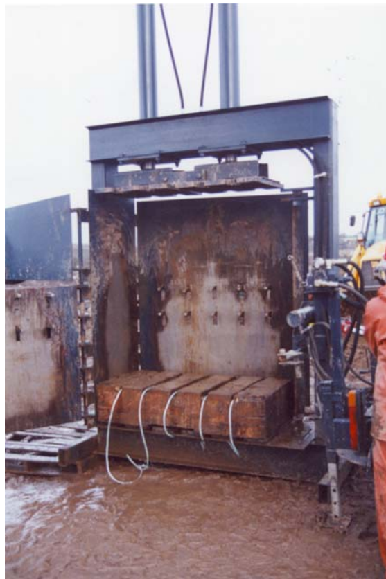
Figure B.18 – Spacers in the baler cavity allow the manufacture of non-standard bales.
