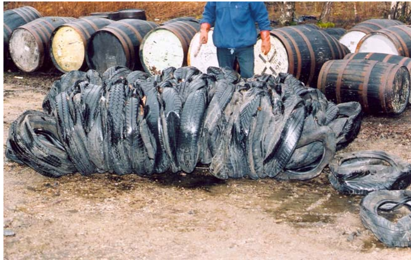
Figure B.15 – Tyre bale immediately after cutting the centre tie-wire.
