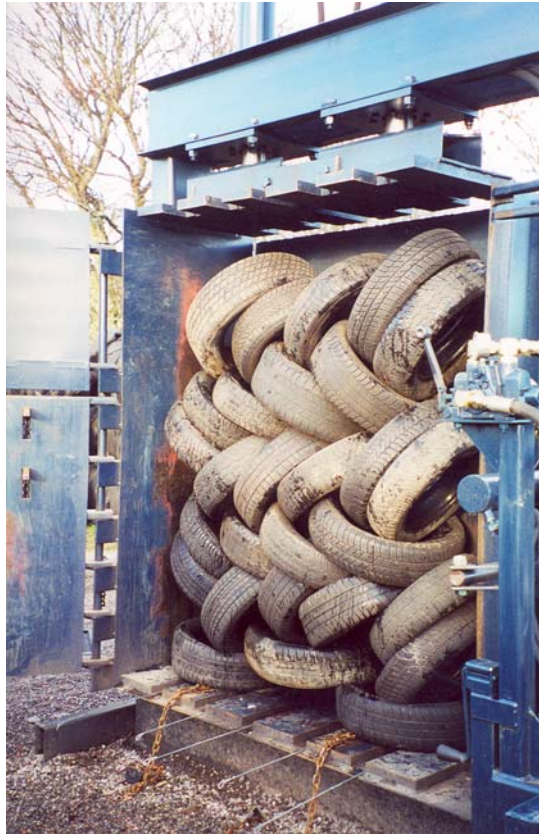
Figure B.1 – Filling the tyre baler, note the five tie-wires and two bale removal chains at the base of the baler. (Photograph © Northern Tyre Recycling Ltd.)
