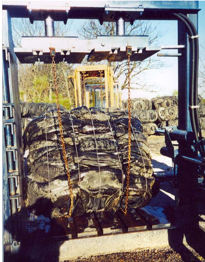
Figure B.8 – Removal of the bale. (Photograph © Northern Tyre Recycling Ltd.)
