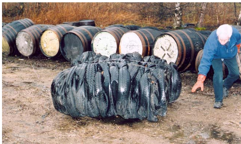
Figure B.13 – Tyre bale immediately after cutting the far inner tie-wire.
