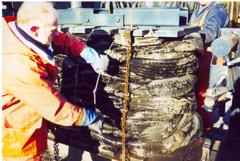
Figure B.6 – The fully compressed bale with ties wires in position and the bale removal chains secured to the front of the top platen. (Photograph © Northern Tyre Recycling Ltd.)
