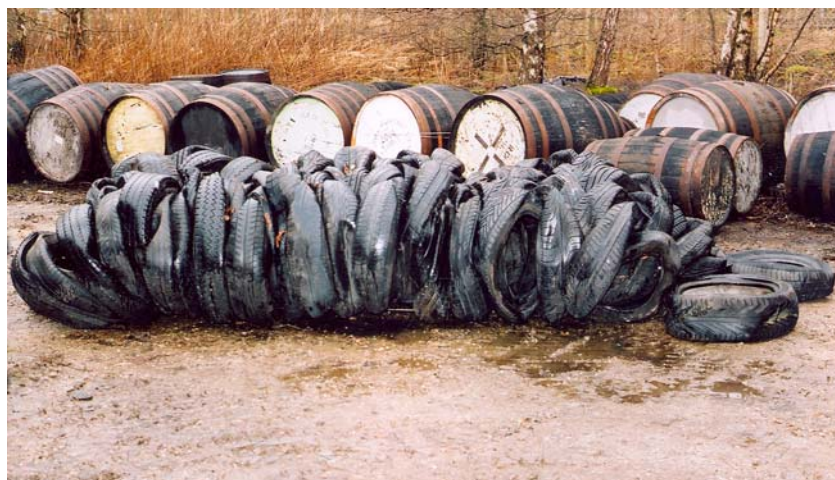
Figure B.17 – Tyre bale 1320 minutes (22 hours) after the tie-wires were cut.
