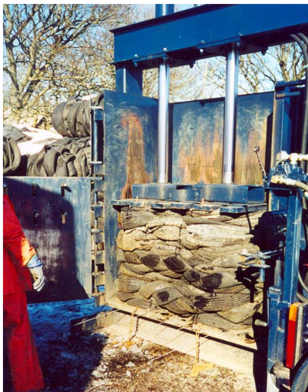
Figure B.2 – Tyres compressed to the first set of dog-levers. (Photograph © Northern Tyre Recycling Ltd.)
