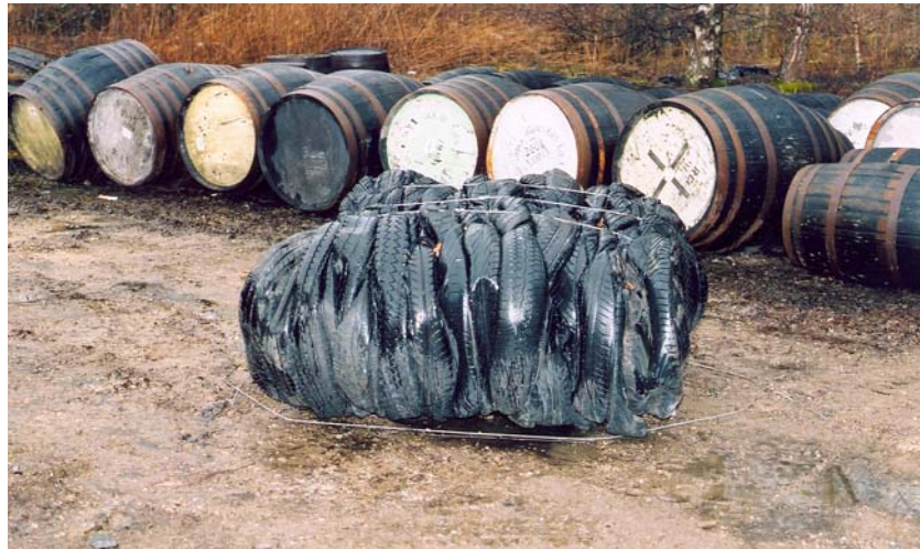
Figure B.12 – Tyre bale immediately after cutting the near outer tie-wire.
