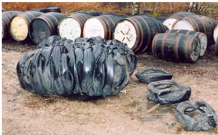
Figure B.14 – Tyre bale immediately after cutting the near inner tie-wire.
