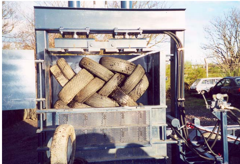
Figure B.3 – Further tyres added to the bale ready for further compression. (Photograph © Northern Tyre Recycling Ltd.)
