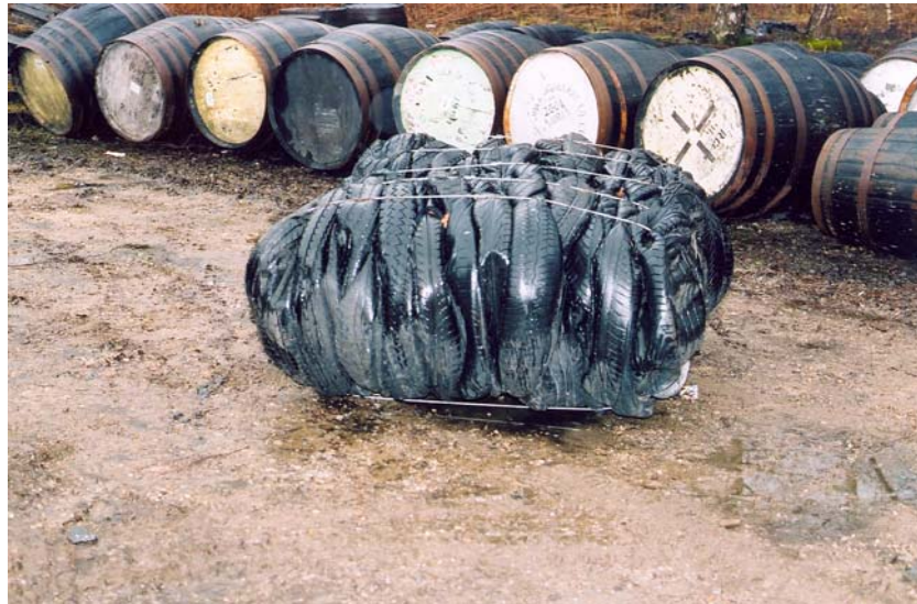
Figure B.10 – Tyre bale prior to cutting of the tie-wires.
