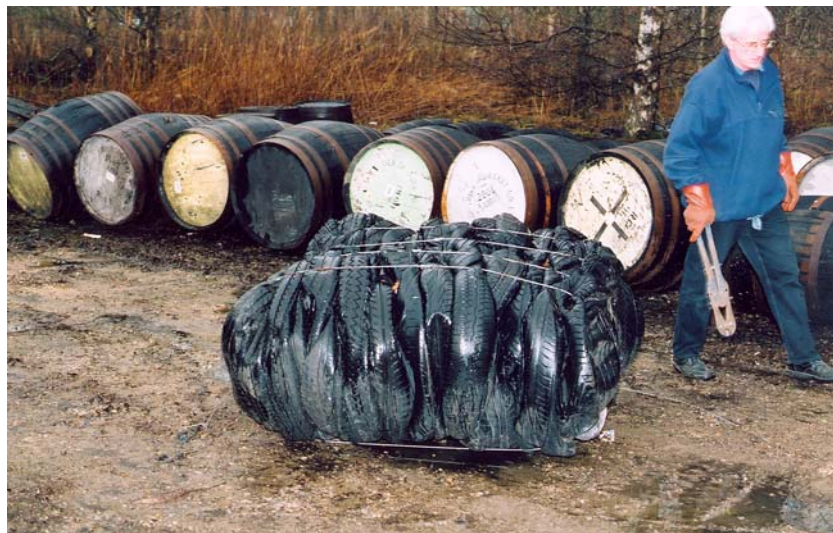
Figure B.11 – Tyre bale immediately after cutting the far outer tie-wire.
