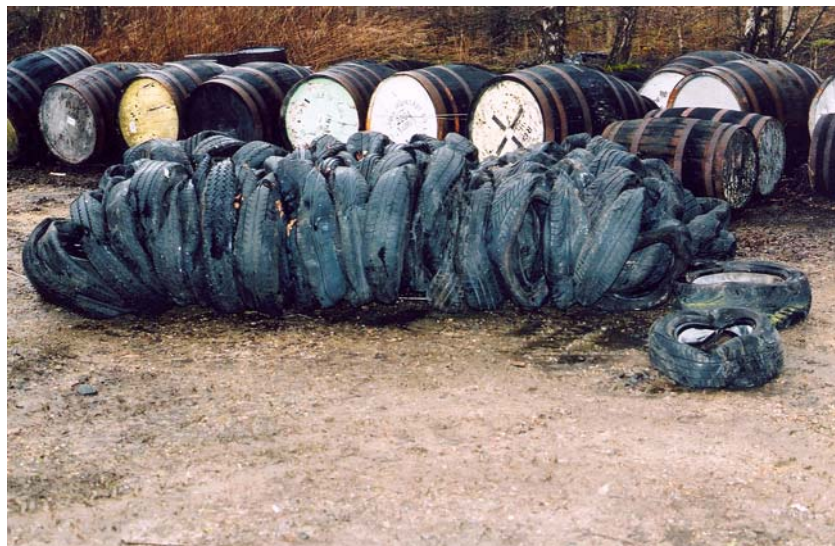
Figure B.16 – Tyre bale 300 minutes (5 hours) after the tie-wires were cut.
