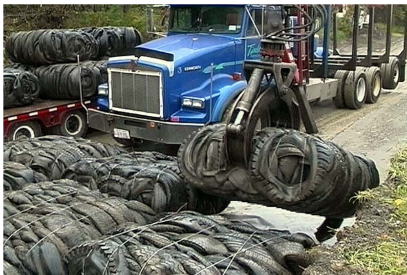
Figure 6.3 – Use of a ‘loggers’-clam’ to handle tyre bales.
