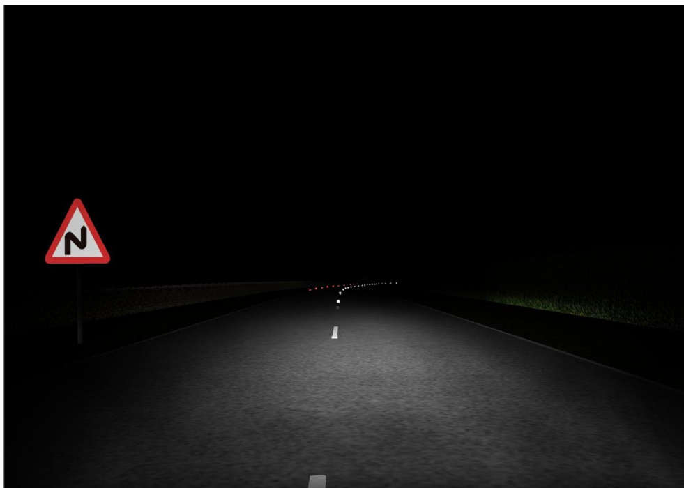
Figure C2. Picture 2 showed the road with Active road studs in place.
