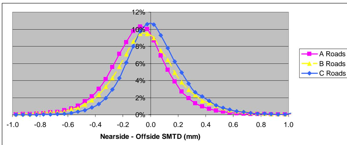
**Figure 3-4 Differences between nearside and offside wheelpath texture measurements**
