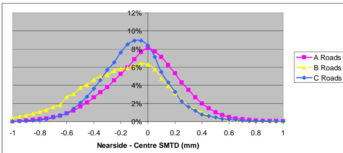
**Figure 3-5 Differences between nearside and centre-line wheelpath texture measurements**
