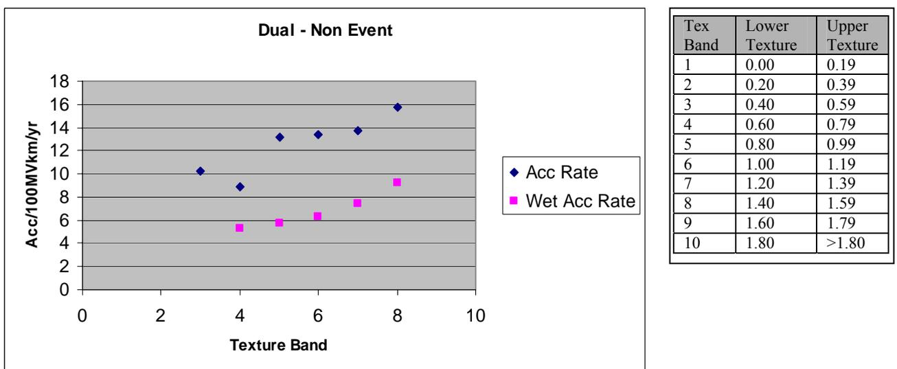
Figure B10 Accident Rate versus Texture for Dual non Event Site Below the IL
