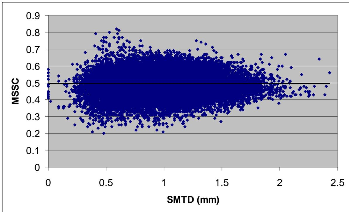
Figure 4-1 Relationship between skid resistance and texture depth – non-event lengths
