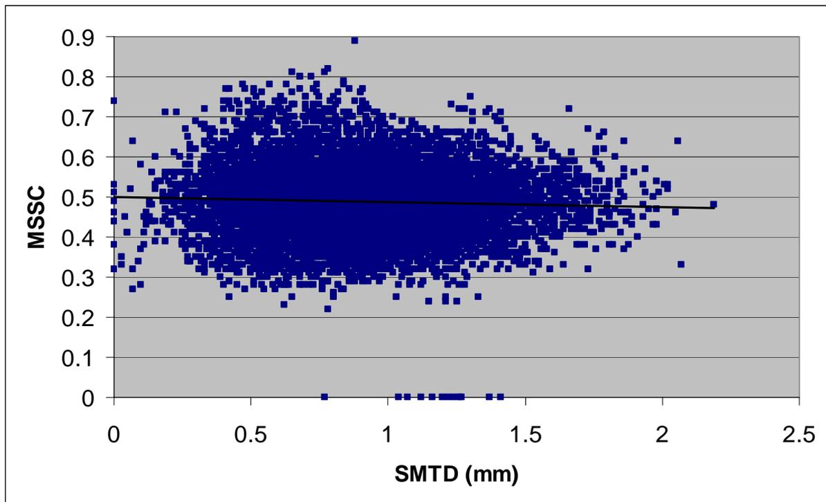
Figure 4-4 Relationship between skid resistance and texture depth – bends
