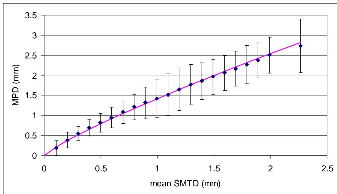
**Figure 3-3 Relationship between SMTD and MPD measures on a larger sample of local roads**
