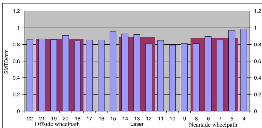
**Figure 5-8 Average texture depth measured by each laser for a section with no defects**
