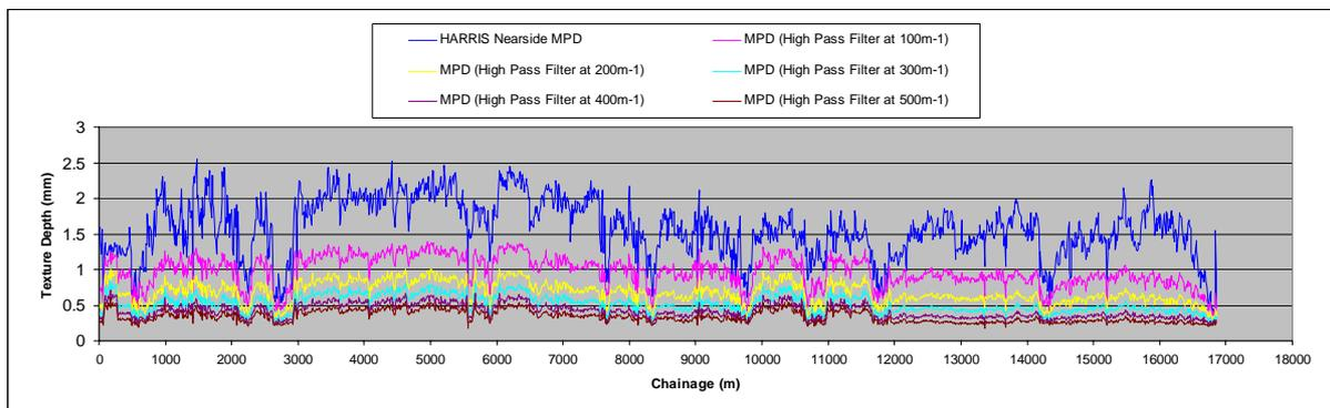
**Figure 4-8 MPD texture profile with standard and additional wavelength filters**
