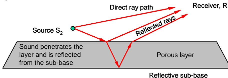
**Figure 6-1 Geometry for a source and receiver in the vicinity of a ground plane**
