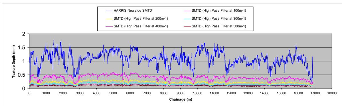
**Figure 4-9 SMTD texture profile with standard and additional wavelength filters**
