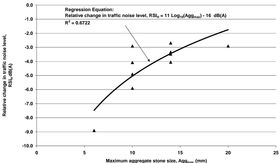
Figure 6-3 Relationship between the relative change in traffic noise and maximum aggregate stone size for high speed roads.
