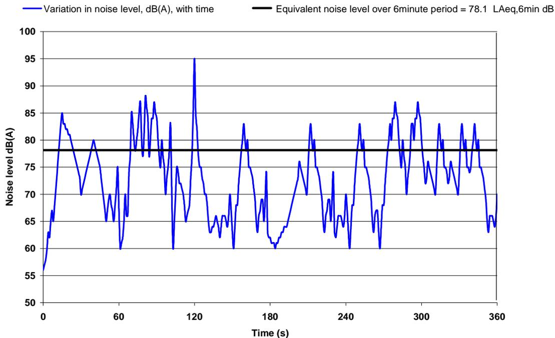
**Figure C3: Variation in traffic noise level and the equivalent noise level,  $L_{Aeq,T}$  dB**
