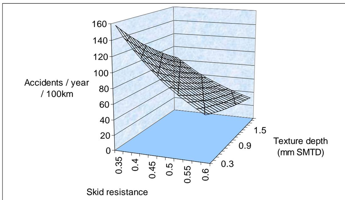
**Figure 4-11 Predicted all-accident rate by skid resistance and texture depth for single carriageway trunk roads in England (reproduced from Parry and Viner, 2005)**
