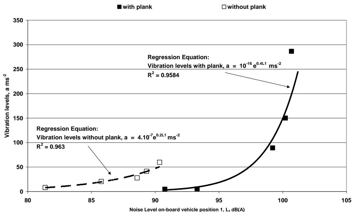
**Figure 6-7 Relationship between chassis vibration levels and on-board noise levels with and without plank**
