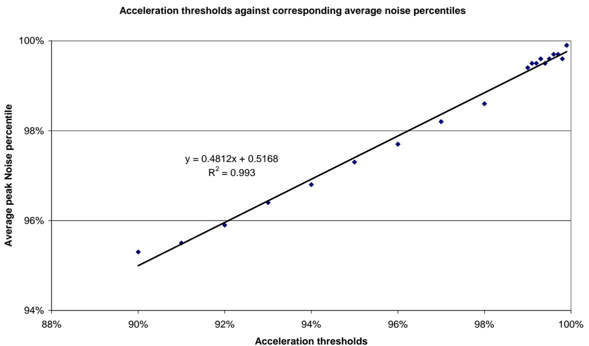
**Figure 6-11 Acceleration percentiles and corresponding average noise percentiles**
