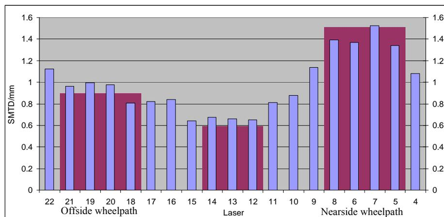
**Figure 5-12 Average texture depth measured by each laser for a section with aggregate loss**
