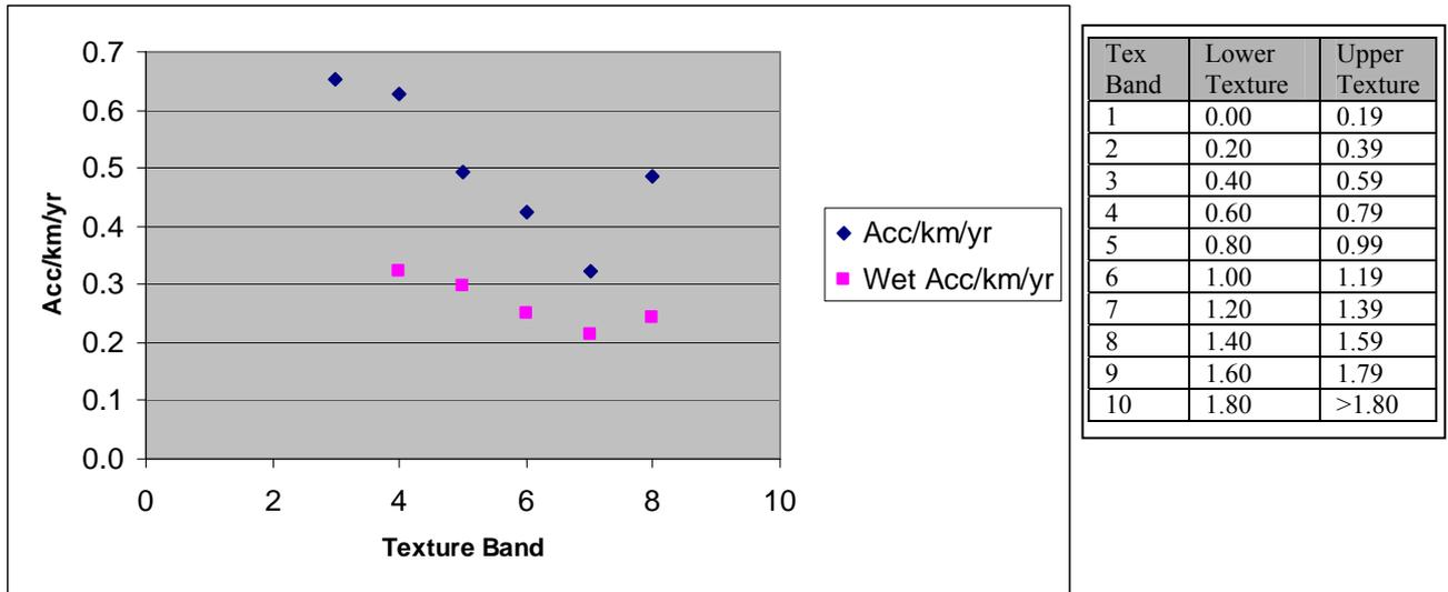
Figure B11 Accident Densities versus Texture for Gradients 5 to 10% Site below the IL
