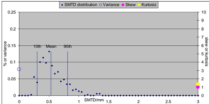
**Figure 5-9 Distribution of depth measurements for a section with fattening up**
