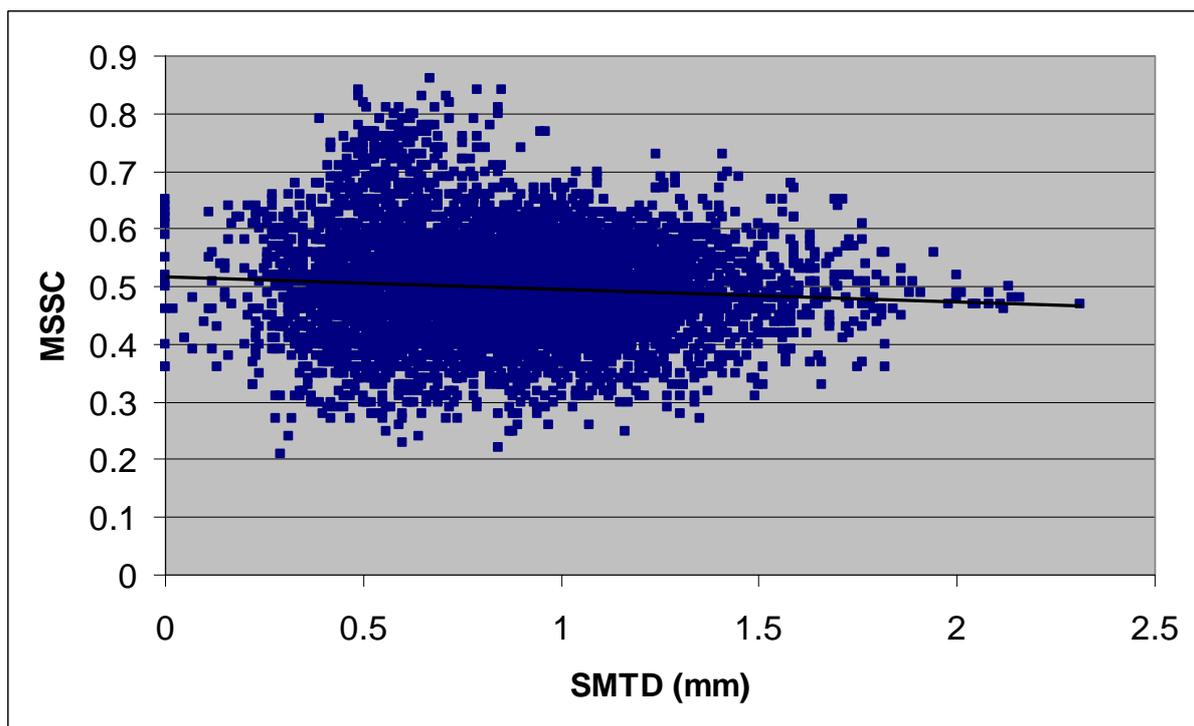
Figure 4-2 Relationship between skid resistance and texture depth – junction approaches
