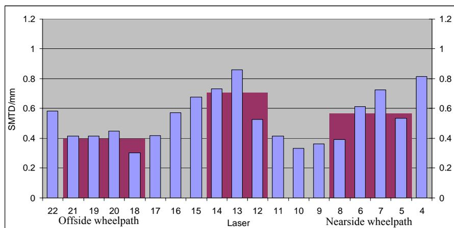
**Figure 5-10 Average texture depth measured by each laser for a section with fattening up**
