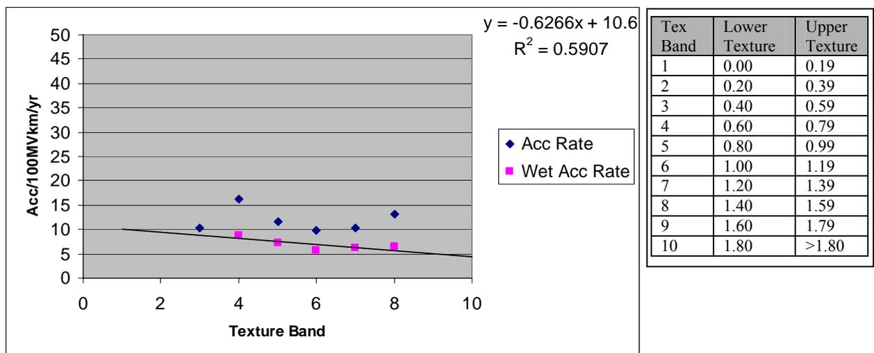
**Figure B14 Accident Rate versus Texture for Rural Gradients 5 to 10%**
