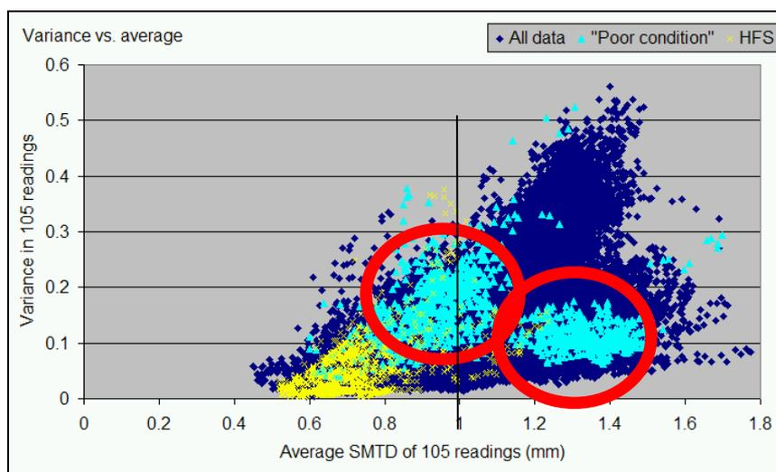
**Figure 5-6 Variance vs average of laser readings**
