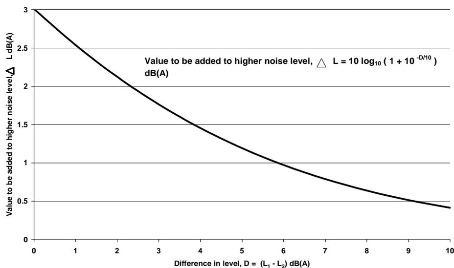
**Figure C1 Combining two noise levels,  $L_1$  and  $L_2$ : value to be added to the higher level,  $\Delta L$ , as a function of the difference in level,  $D = L_1 - L_2$**
