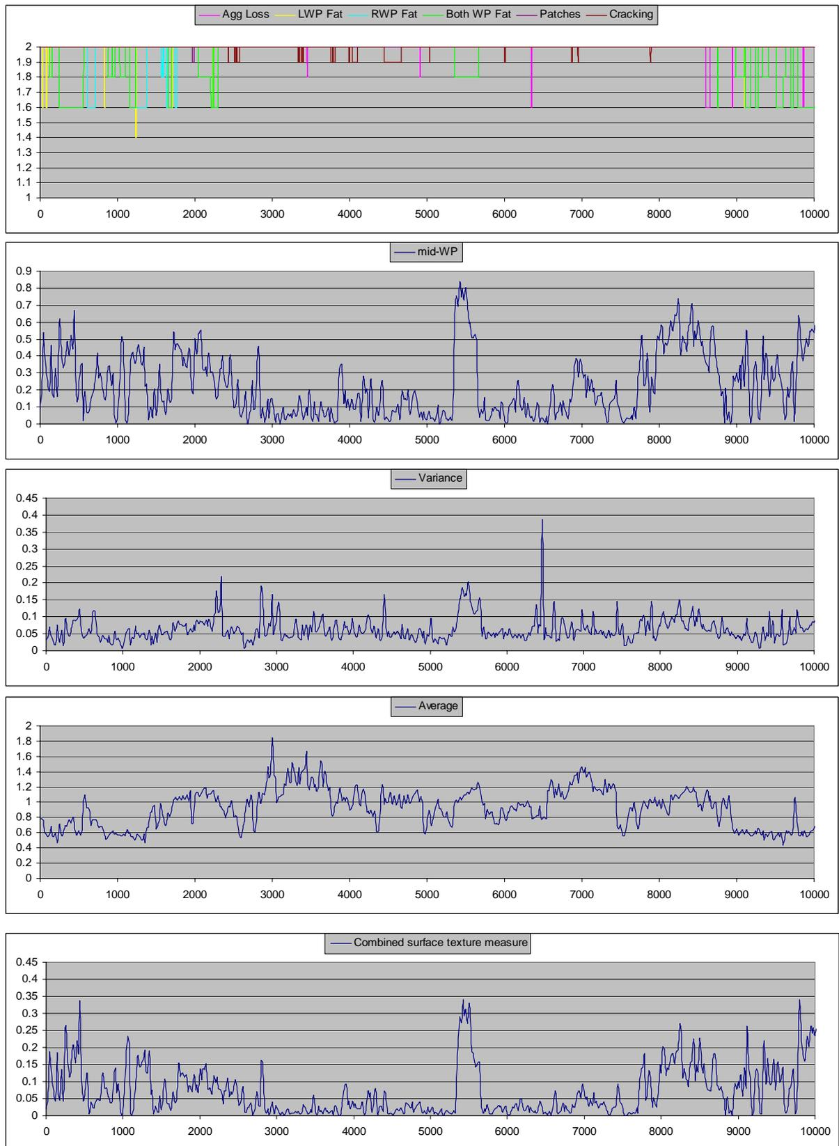
**Figure 5-13 Video inspection and texture measurements**
