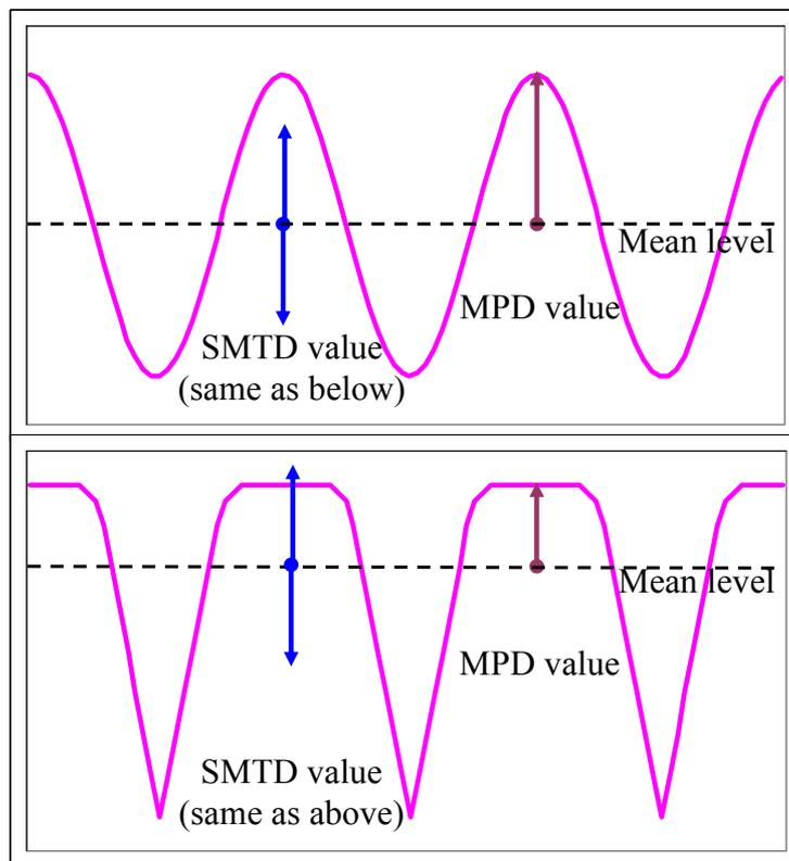
**Figure 3-1 Comparison of SMTD and MPD values for surfaces with different shapes**
