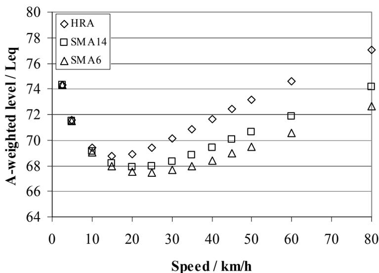
**Figure 6-4 Traffic noise variation with average vehicle speed**
