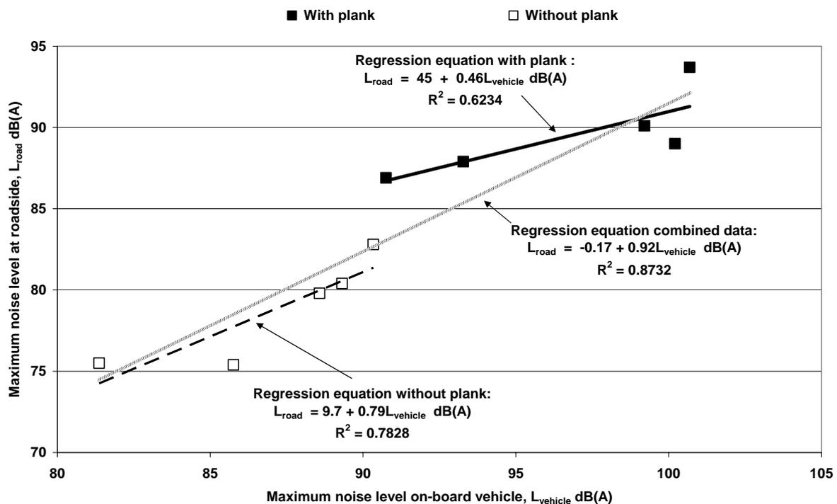
**Figure 6-6 Relationship between roadside noise levels and on-board noise position1, with and without plank**
