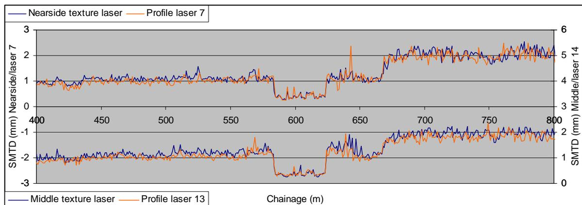
**Figure 5-2 Comparison of measurements using texture lasers and profile lasers**
