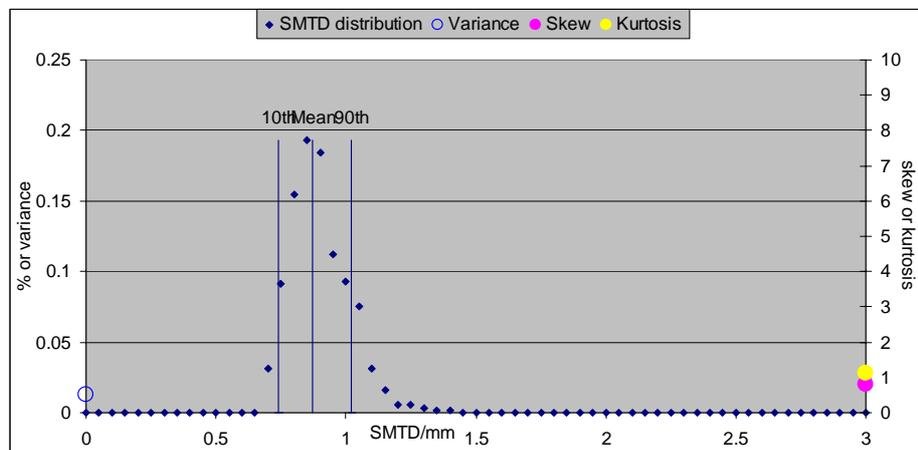
**Figure 5-7 Distribution of texture depth measurements for a section with no defects**
