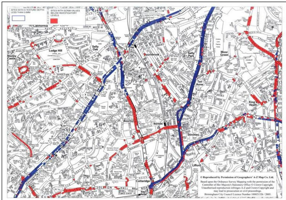
**Figure 4-5 Street map of Birmingham showing roads with texture depth less than 0.6mm (Blue) and skid resistance below the investigatory level (Red)**
