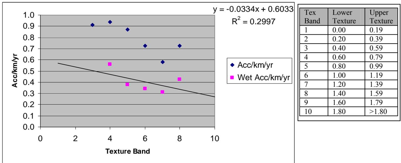
Figure B9 Accident Density versus Texture for Dual non Event Site below the IL
