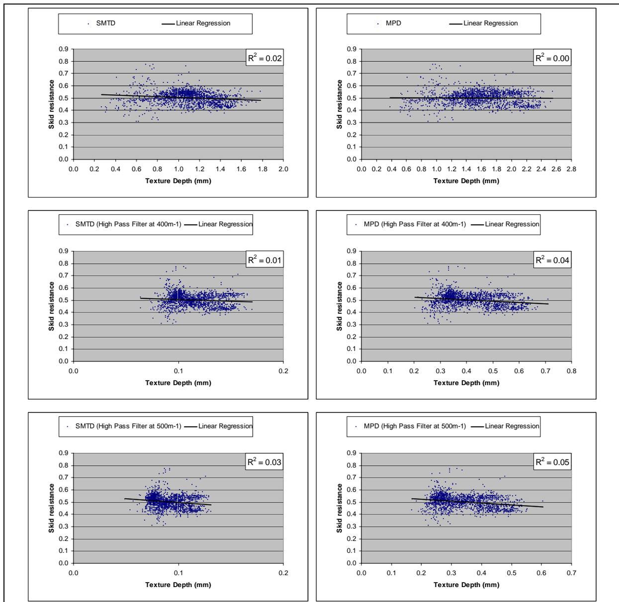
**Figure 4-10 Relationship between texture depth and SCRIM coefficient at a standard speed of 50km/h**
