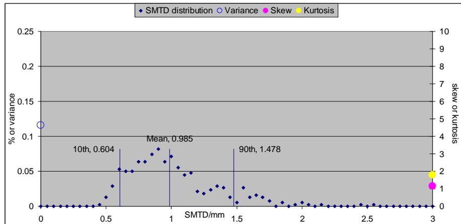
**Figure 5-11 Distribution of depth measurements for a section with aggregate loss**
