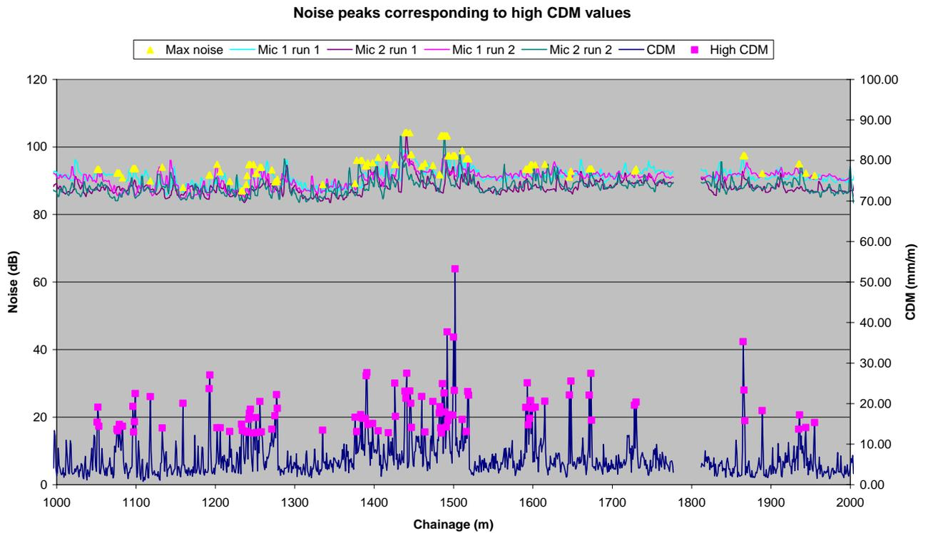
Figure 6-9 Location of CDM<sub>1</sub> values above the 95<sup>th</sup> percentile and the corresponding maximum noise peaks
