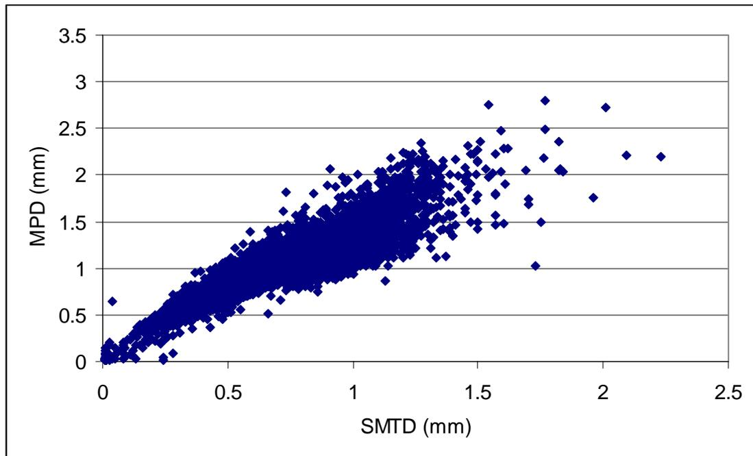
**Figure 3-2 Relationship between SMTD and MPD measures on a sample of local roads**
