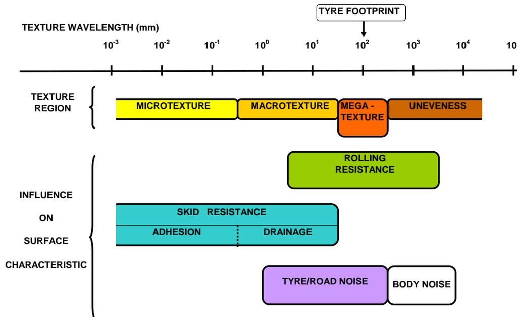
**Figure 6-2 Influence of surface texture on the characterisation of road surfaces**
