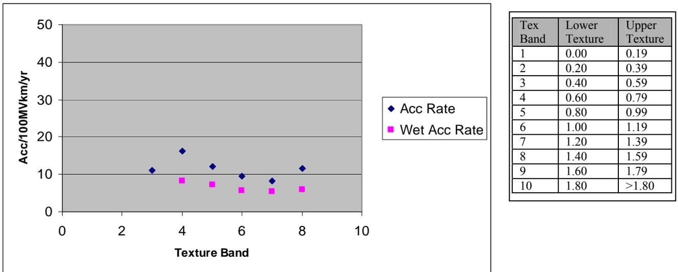
Figure B12 Accident Rate versus Texture for Gradients 5 to 10% Site below the IL
