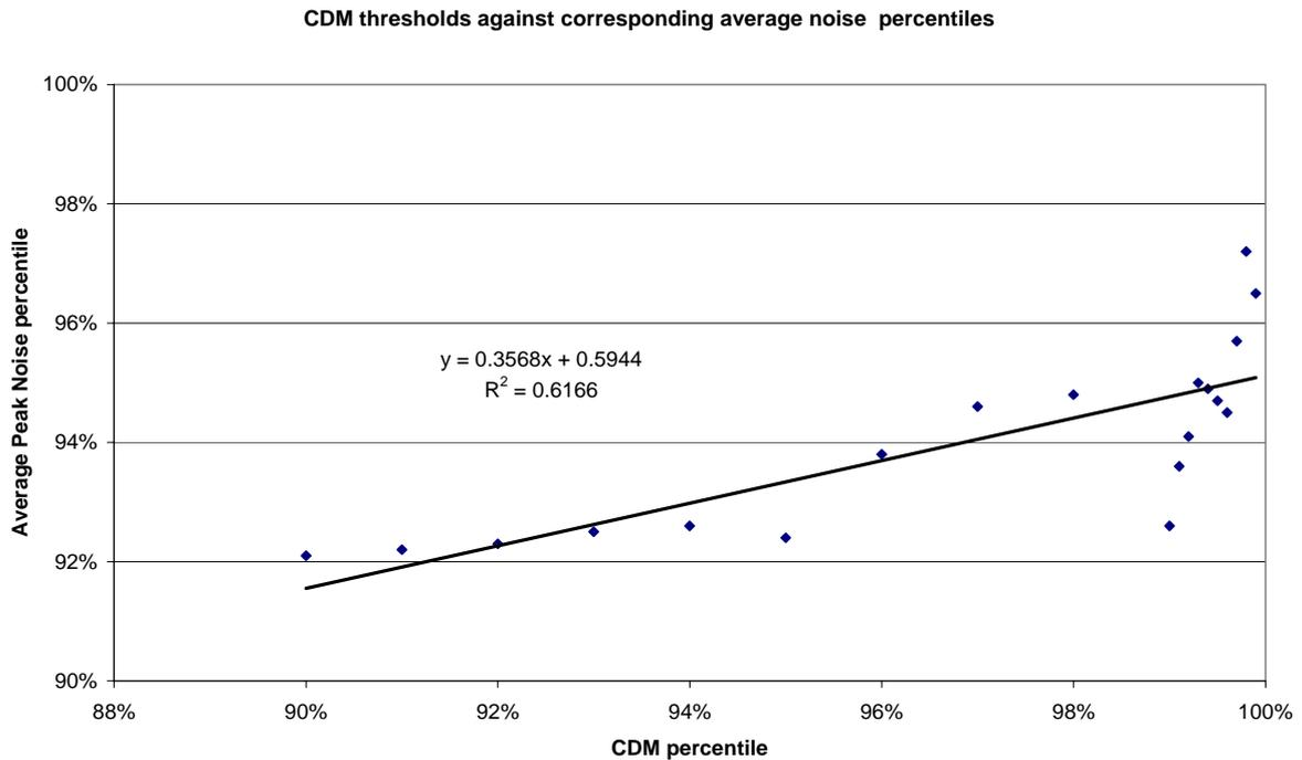
**Figure 6-10 Average noise level\*, as a percentile of all noise measurements, for locations with CDM<sub>1</sub> values above the indicated percentile of all CDM<sub>1</sub> measurements**
