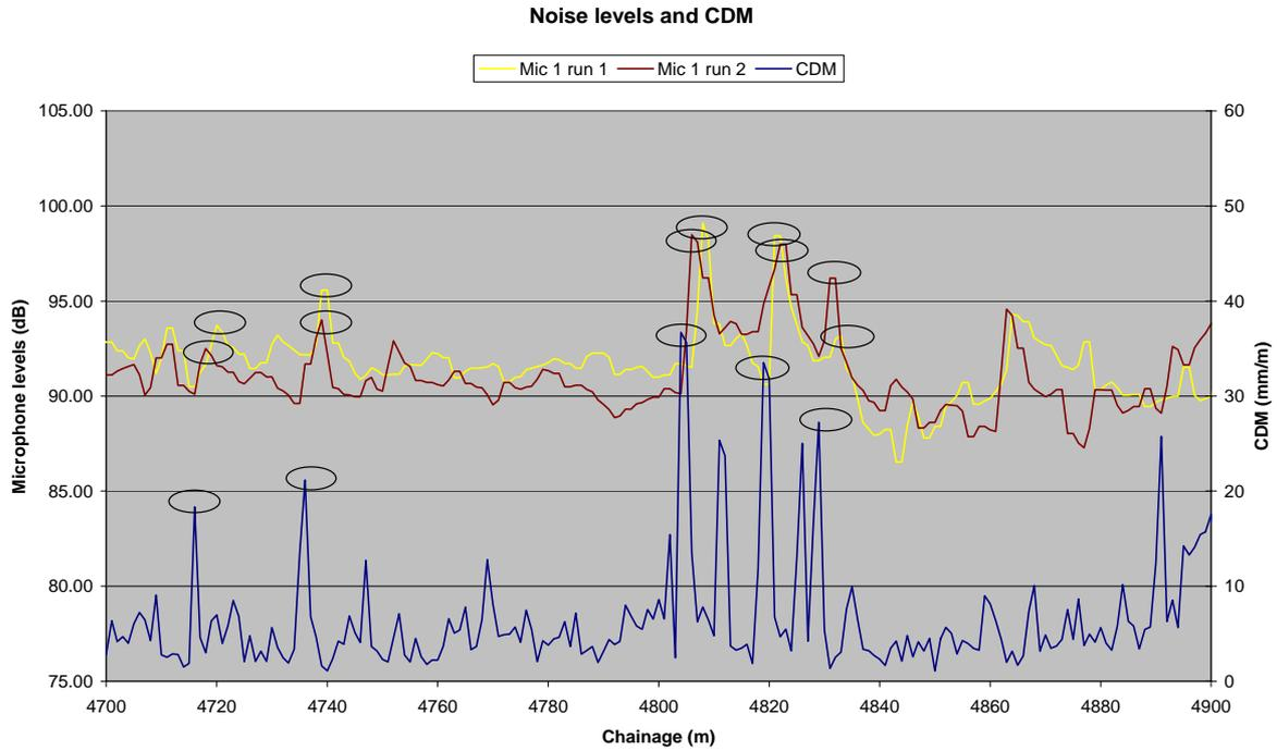
Figure 6-8 Comparison of 2 runs of noise data with the CDM<sub>1</sub> data over the same section of road
