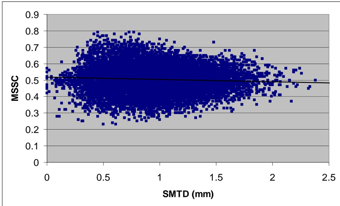
Figure 4-3 Relationship between skid resistance and texture depth – gradients
