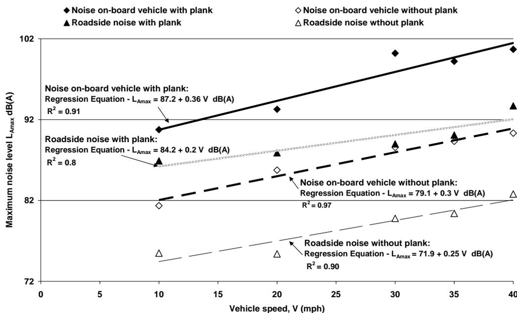
**Figure 6-5 Relationship between roadside noise and on-board noise levels position 1 with speed with and without plank**
