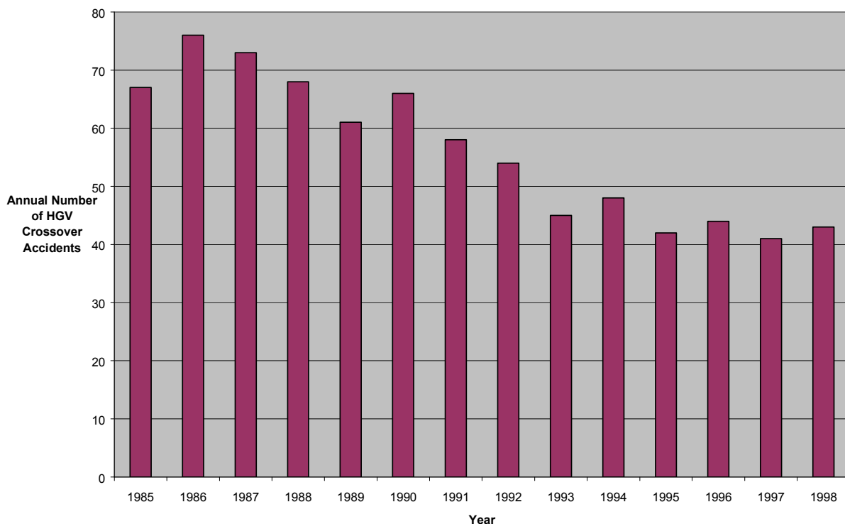
Figure 1: Annual Number of HGV Crossover Accidents on Motorways, A(M) and A roads in Great Britain (Of All Severity) (see Appendix C, Table C1)
