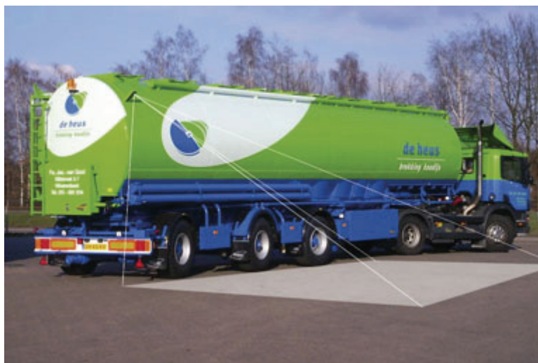
Figure 43: Field of view from camera mounted on the side of trailer (Orlaco, 2007)
