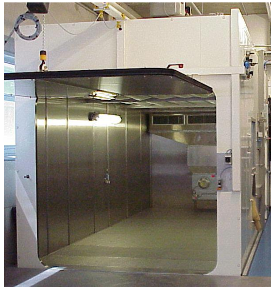
Figure B8-2: SHED facility at FH Joanneum GmbH Graz, Austria.
