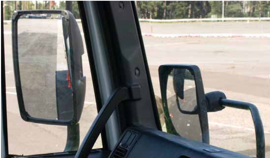
Figure 50: Example of potential blind spot behind nearside A-pillar on Iveco (Photo ref: P8017334).
