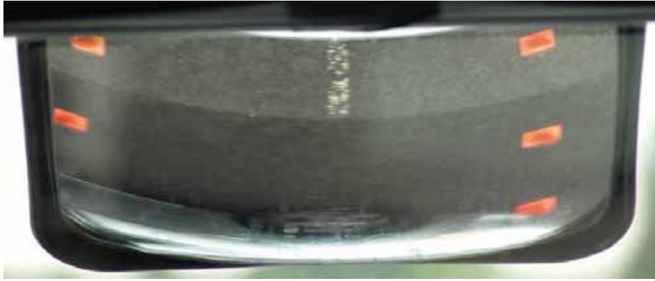
Figure 54: Passing car positioned in the centre of adjacent lane is just visible in correctly adjusted close proximity mirror meeting Directive 2003/97/EC.
