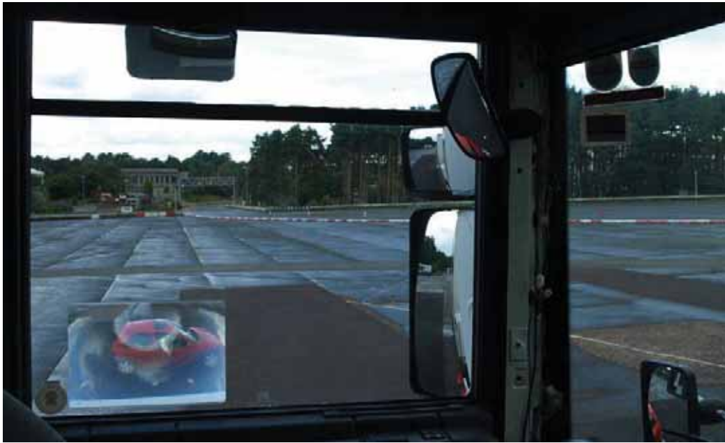
Figure 43: Small passenger car not visible through direct field of vision from the 5 th percentile driver of the Renault although it was clearly visible in the Fresnel lens (Photo ref: P8147890).
