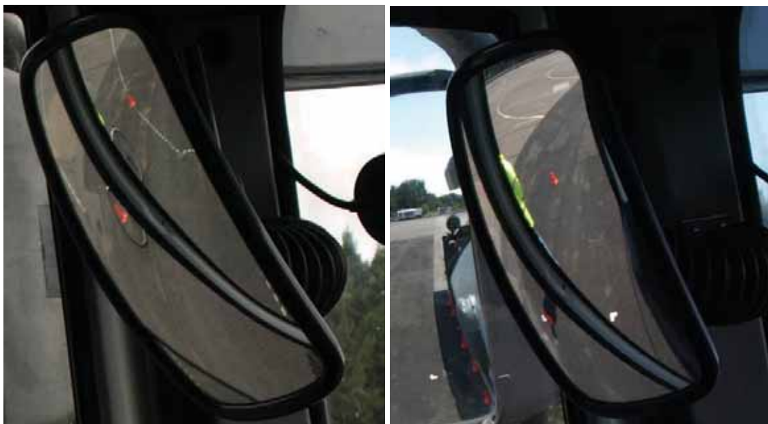
Figure 56: Cyclist and pedestrian partly hidden by the window frame visible in the BDS mirror.
