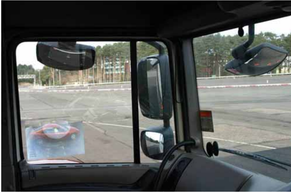
Figure 41: Direct visibility through passenger side window of DAF just shows roof of Mondeo which is clearly visible in Fresnel lens (Photo ref: P2119081).
