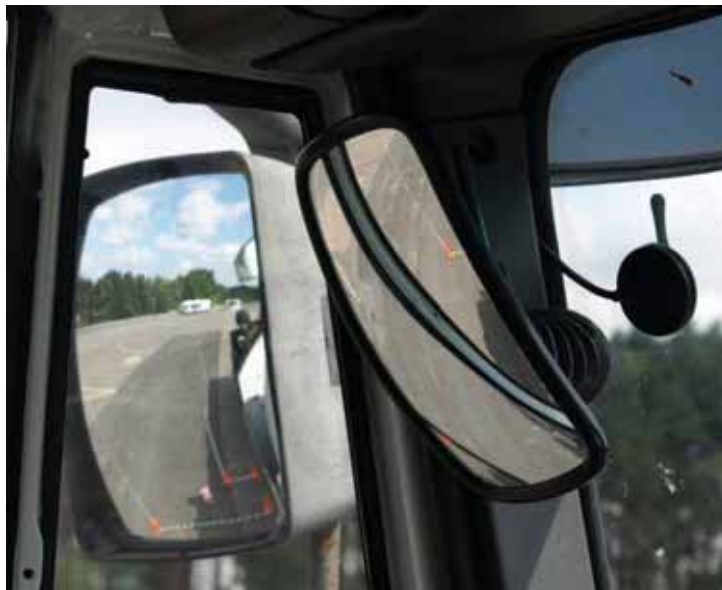
Figure 12: BDS Dead Angle Mirror System.
