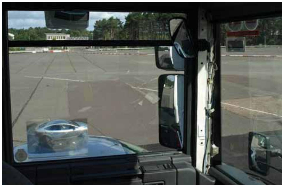
Figure 42: Direct visibility through passenger side window of Renault clearly shows Mondeo (Photo ref: P8147639).
