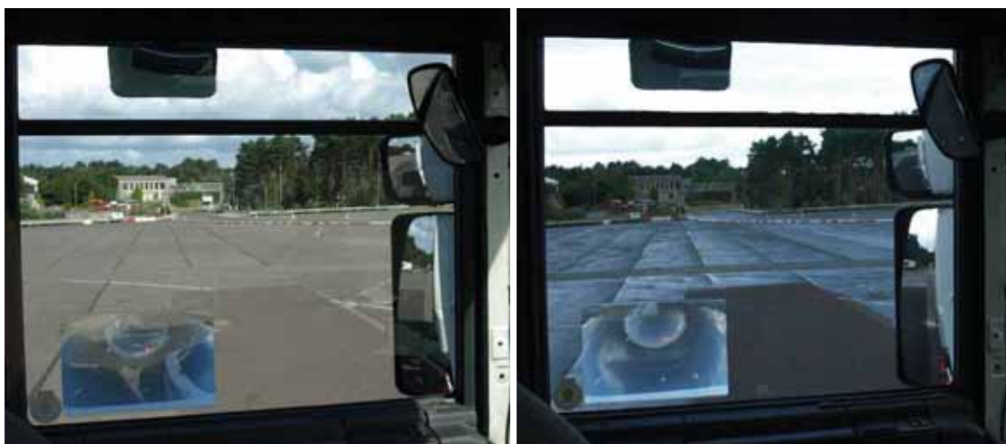
Figure 55: Example of large passenger car just visible in Fresnel lens (left), whilst the small passenger is not visible in the Fresnel lens (right)
