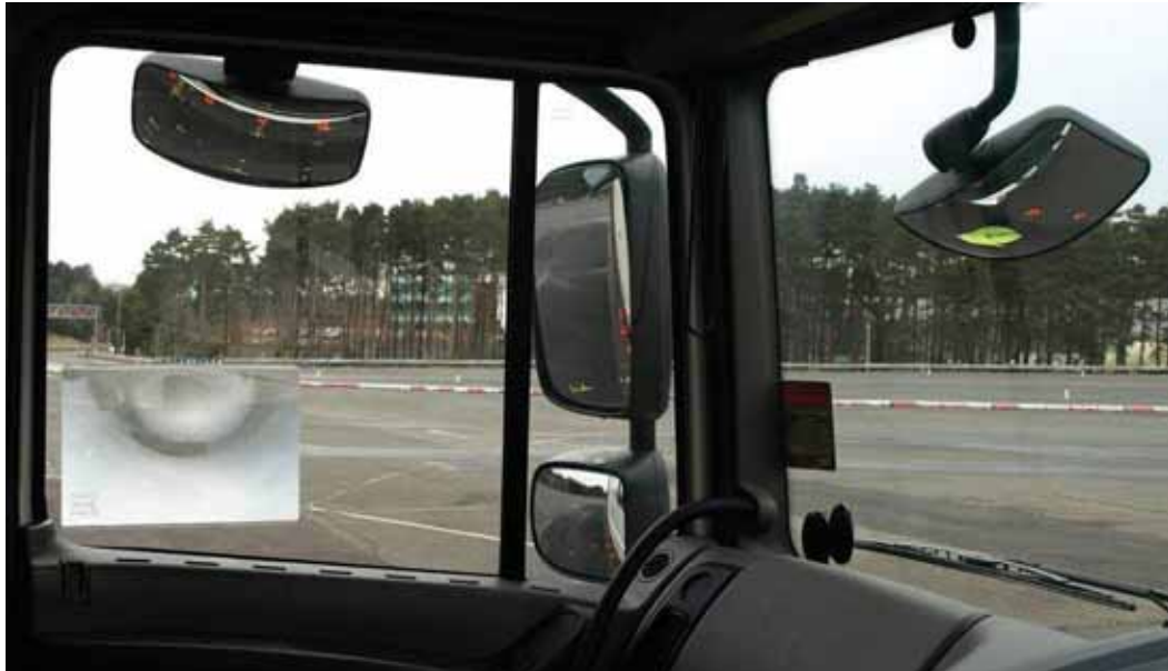
Figure 48: Pedestrian only visible in Class VI (front) mirror on the DAF vehicle when standing at the closest edge of the adjacent lane and two metres ahead of the driver's ocular point (Photo ref: P2129754).
