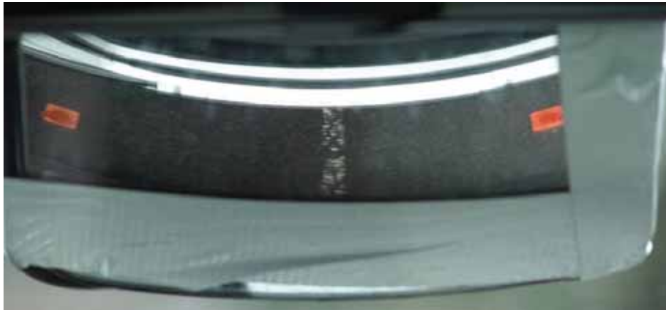
Figure 52: Passing car positioned the closest edge of adjacent lane is not visible in poorly adjusted close proximity mirror meeting Directive 71/127/EEC.
