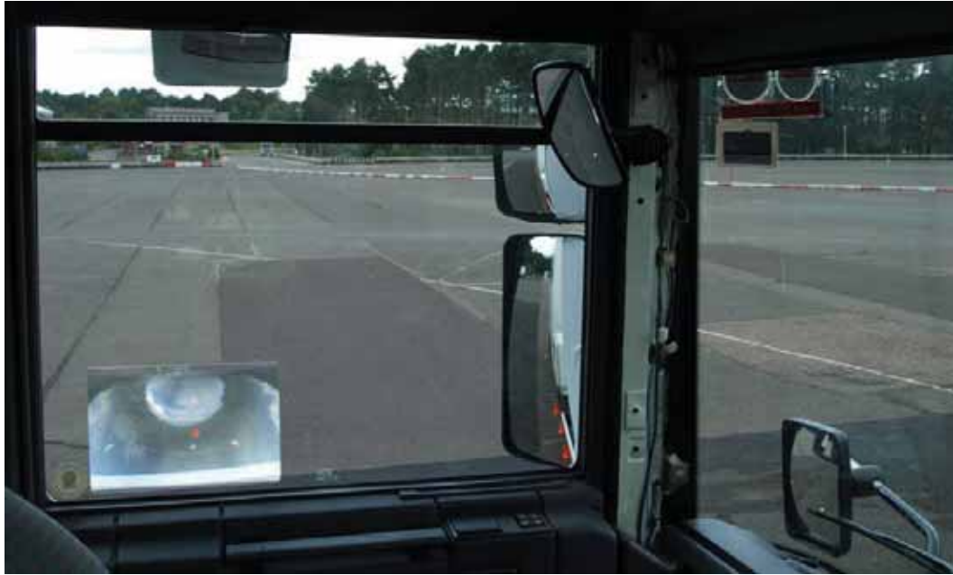
Figure 46: Pedal cyclist in blind spot of Renault test vehicle (Photo ref: P8147725).
