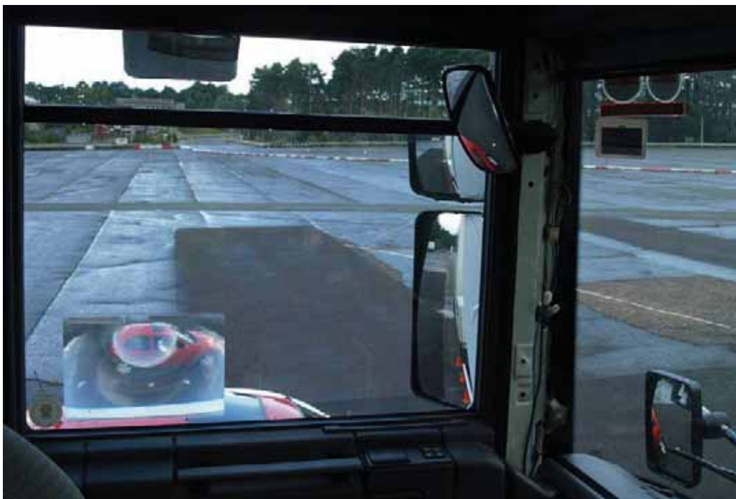
Figure 44: Small passenger car directly visible through side window as viewed from the 95 th percentile driver of the Renault (Photo ref: P8147852).
