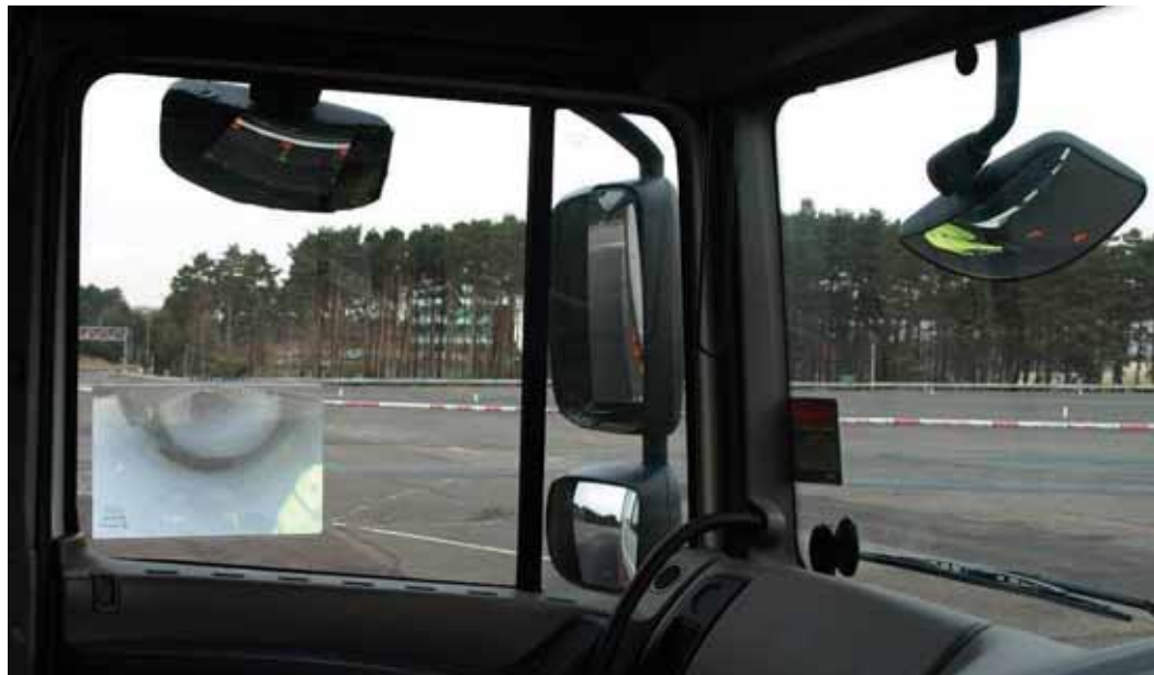
Figure 47: Pedal cyclist visible in Class VI (front) mirror fitted to DAF test vehicle (Photo ref: P2129721).
