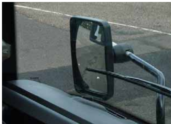
Figure 36: Windscreen wiper partly obstructing Dobli mirror on Renault test vehicle.
