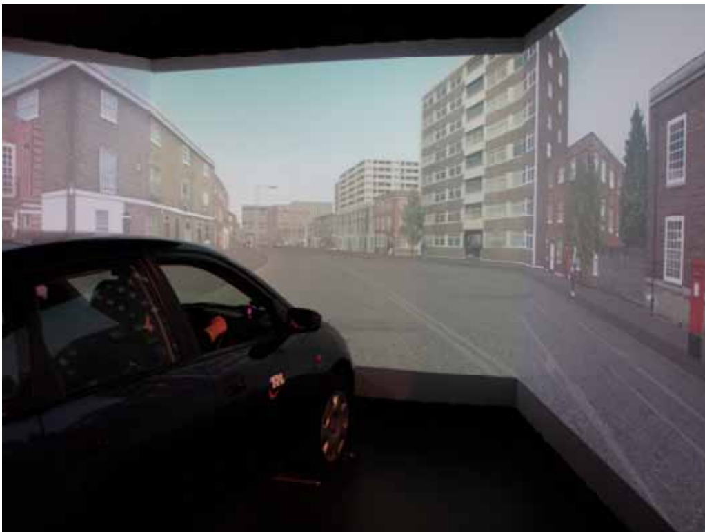
Figure 3.1: TRL CarSim (displaying the simulated London database created for this project)
