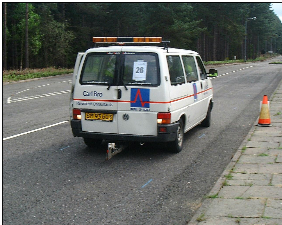
Figure B4: Grontmij-CarlBro vehicle-mounted HWD
